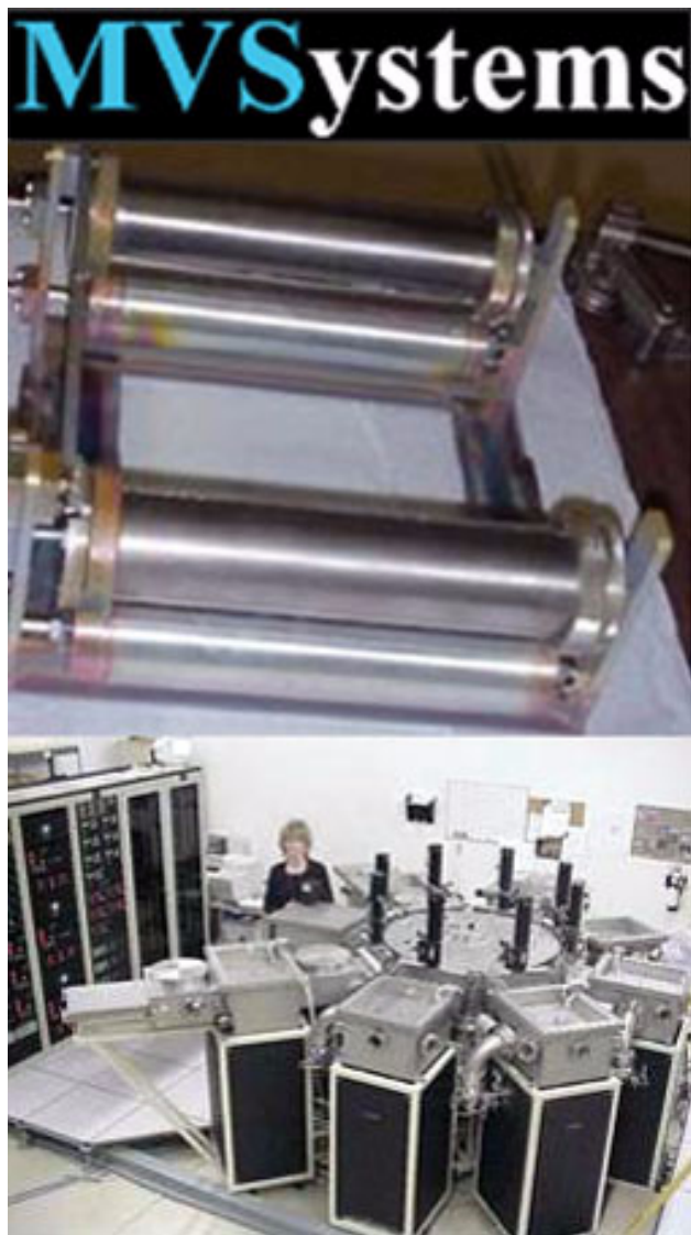
Figure 5. MVSystems' thin film fabrication equipment to be used as the basis for initial cost analyses of scaled-up HPE systems: (a) patented reel-to-reel cassette technology; (b) vacuum cluster tool using the cassette technology for depositing successive thin film layers over large areas of rolled foil substrates.
