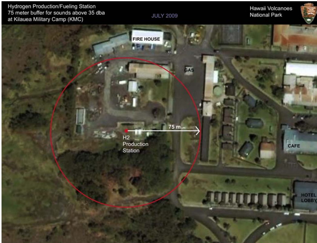
Figure 1: Hydrogen Production/Fueling Station Acoustic Specification
