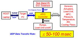
Fig. 2: New controller/communication Configuration
