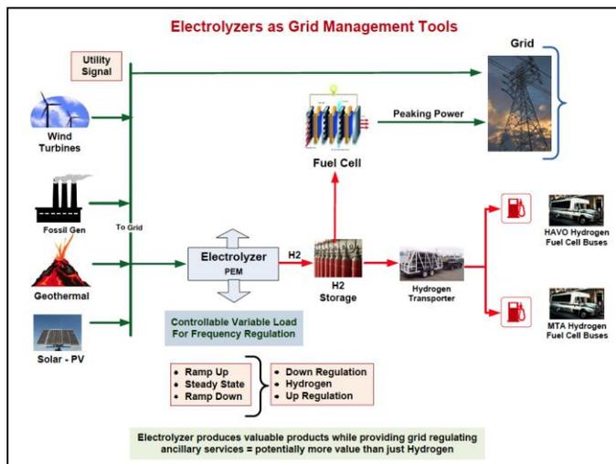
Figure 1: Batteries & Electrolyzers as Grid Management Tools
