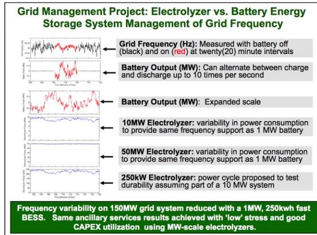
Figure 2: Comparison of a Battery Energy Storage System with a Dynamically Operated Electrolyzer Managing Grid Frequency
