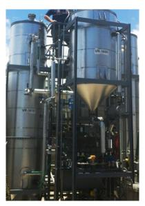
BACKGROUND: Over a number of years, an up-flow anaerobic packed bed reactor was developed. Packed with biochar in various formulations, these reactors were verified at lab and demonstration scale to treat high and low strength wastewaters efficiently. These exercises served to verify lab generated results upon scale up to commercial size and to provide crucial insights for design revision, as well as experience for discussion with manufacturers as well as equipment selection.
