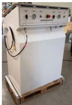
Figure 8: New hydrogen compression post
