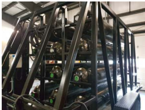
Figure 7: Hydrogen Transport Trailer undergoing certification at Powertech
