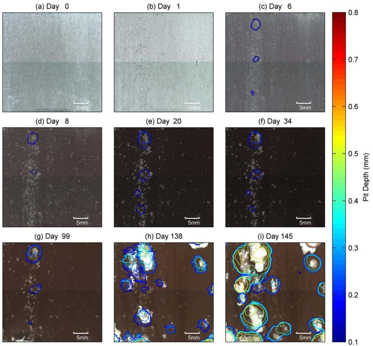
***Figure 3-8: Front view photographs of the 2024 Aluminum sample's area of interest after indicated days of submersion in surface seawater with ultrasonically measured pit depth contours overlaid.***
