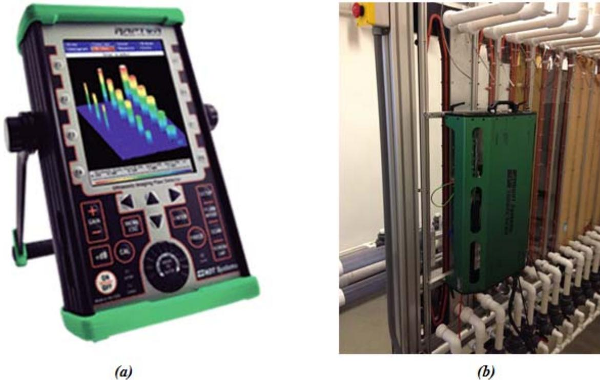
***Figure 3-5: NDT Systems RAPTOR imaging flaw detector and (b) TunnelScan mounted on the back side of Makai's corrosion rack.***
