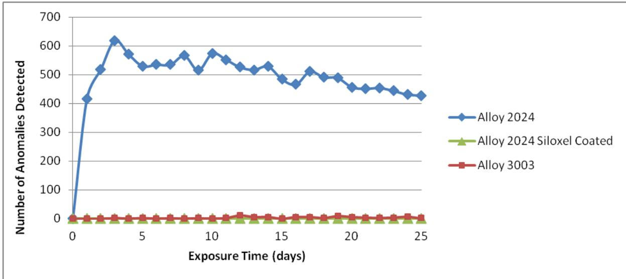
**Figure 3-3: Number of anomalies detected for the three different aluminum samples**
