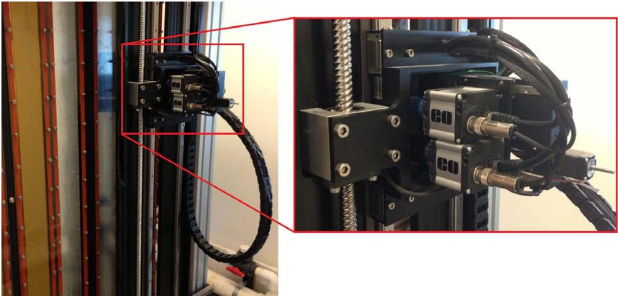
*Figure 3-1: Photograph of Makai's corrosion rack with motorized X-Y-Z stage and imaging apparatus. Zoomed in view shows the Y-stage and Z-stage with the two mounted cameras. The top camera has the long microscope lens attached and the bottom camera has the short wide field of view lens.*
