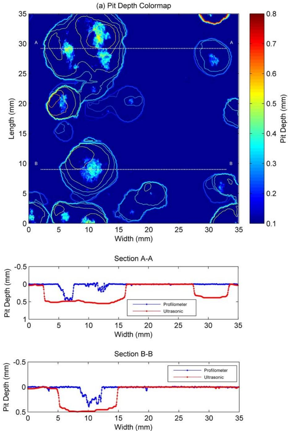
**Figure 3-10: (a) Map of the 2024 Aluminum sample's area of interest after 145 days of submersion in surface seawater with profilometrically measured pit depth shown as a solid color, and ultrasonically measured pit depth contours overlaid. Both data sets use the color bar scale. (b)-(c) Cross section views showing depth data as measured with the profilometer (blue) and ultrasonic (red).**
