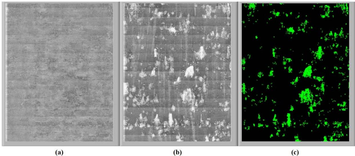
***Figure 3-2: (a) Sample area of Alloy 2024 at day 1. (b) Alloy 2024 at day 26. (c) Detected pitted area shown in green***
