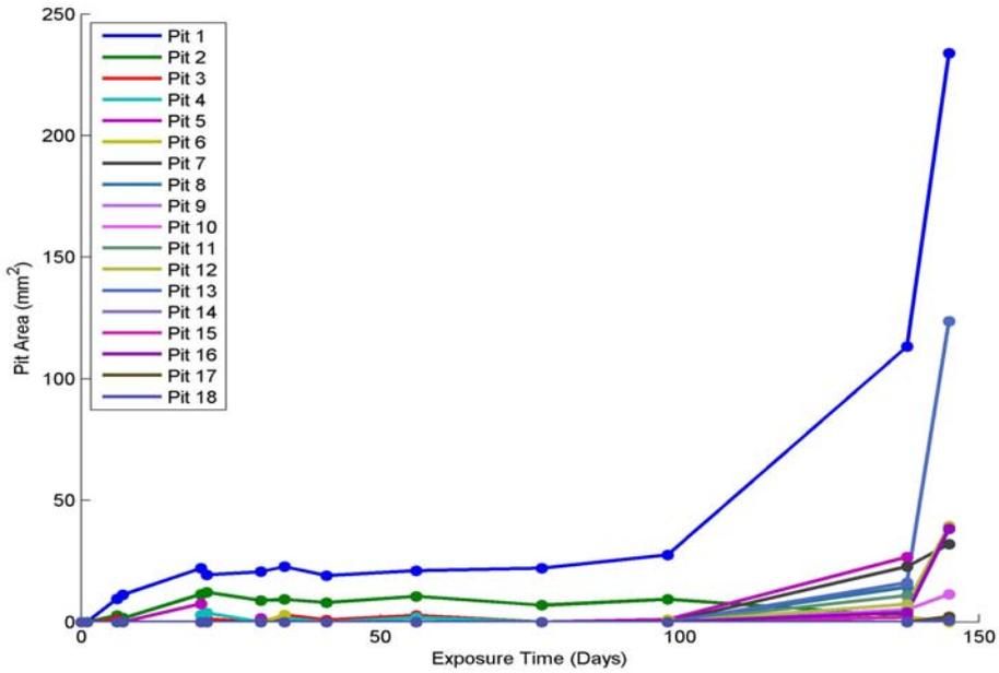
**Figure 3-7: The ultrasonically measured area of 18 tracked pits on the 2024 Aluminum sample submerged in surface seawater for 145 days.**
