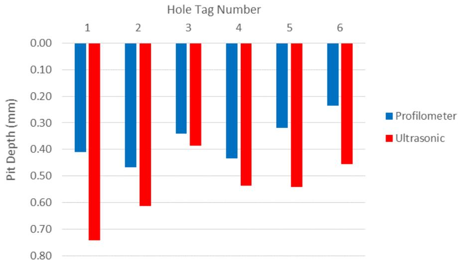
***Figure 3-9: Comparison of pit depth of the 2024 Aluminum sample’s area of interest after 145 days of submersion in surface seawater measured using ultrasonic and profilometry techniques.***
