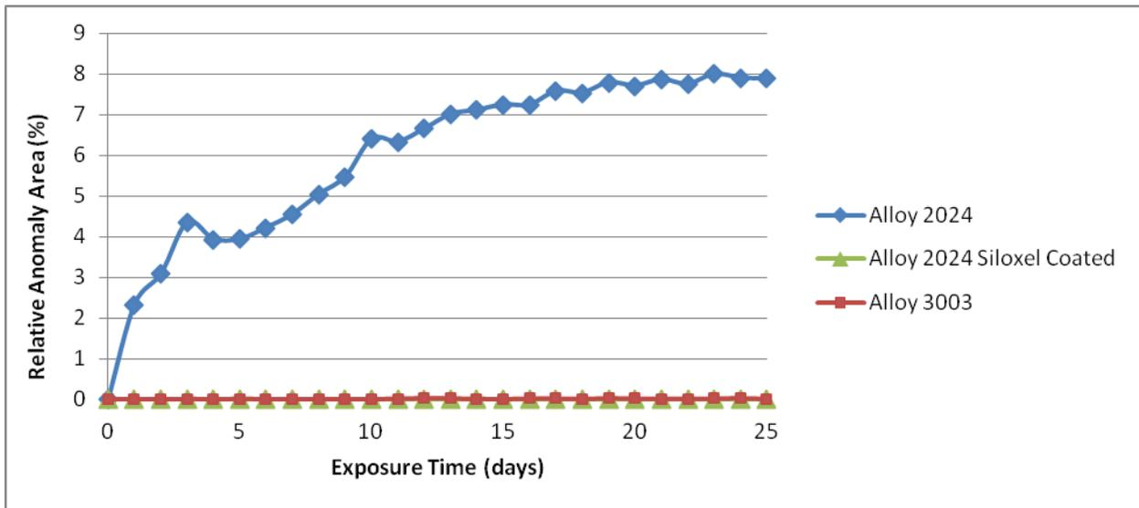
**Figure 3-4: Relative anomaly area (%) for the three aluminum samples**
