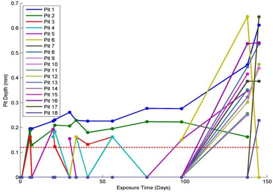
**Figure 3-6: The ultrasonically measured depth of 18 tracked pits on the 2024 Aluminum sample submerged in surface seawater for 145 days.**
