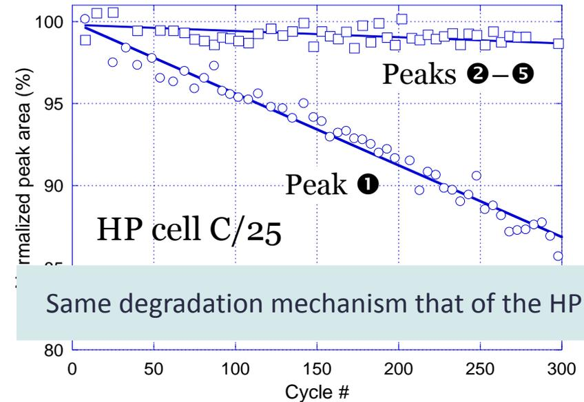
Mechanistic analysis proved that the capacity loss for both cells is solely induced by LLI and that it seems to be always accompanied by some  $LAM_{deNE}$
