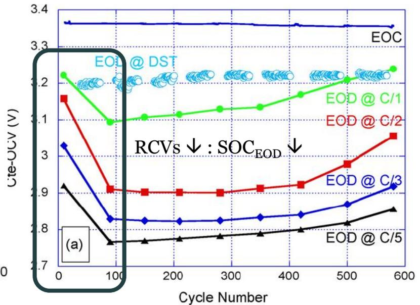
We speculated it was the result of a combination of LLI and a “reservoir effect” arisen from the loading matching between the PE and the NE.
