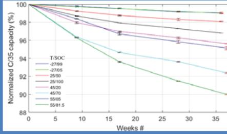
Capacity loss influenced by both temperature and SOC.
