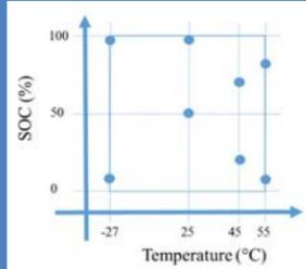
Calendar aging experiment designed for maximum accuracy @ high temperature & high SOC
