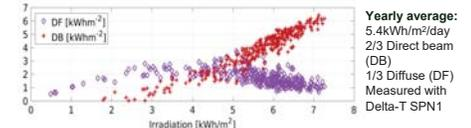
Fig. 3: Energy from the direct and diffuse components versus global irradiation
