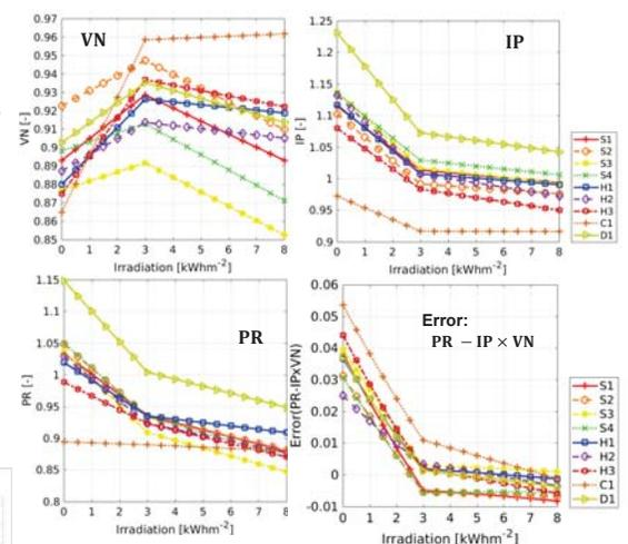
Fig. 4: PV Performances versus Irradiation – Module Comparison
