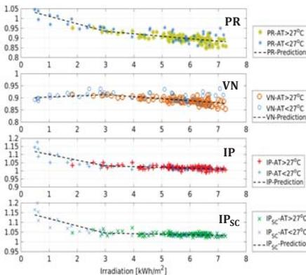
Fig. 2: PV Performances versus Irradiation – Data and model (Module S4)
