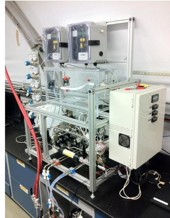
Custom made air filtration material gas sorption testing stand.
