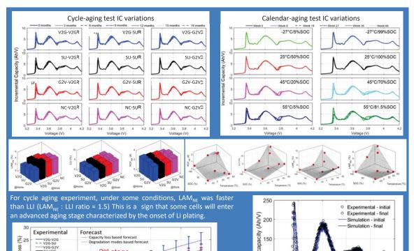
Results led to prediction of a second accelerated aging stage characterized by the onset of lithium plating.
