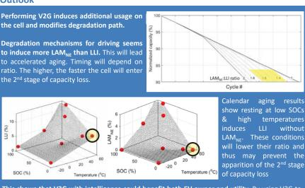
This shows that V2G with intelligence could benefit both EV owner and utility. By using V2G to get the battery in a calendar aging condition that lowers the LAM $_{\rm NE}/{\rm LLI}$  ratio, the overall durability of the battery might increase despite the additional usage.
