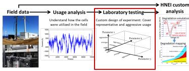
Laboratory testing encompassing a wide range of grid applications including frequency regulation, reserve and peak shaving.
