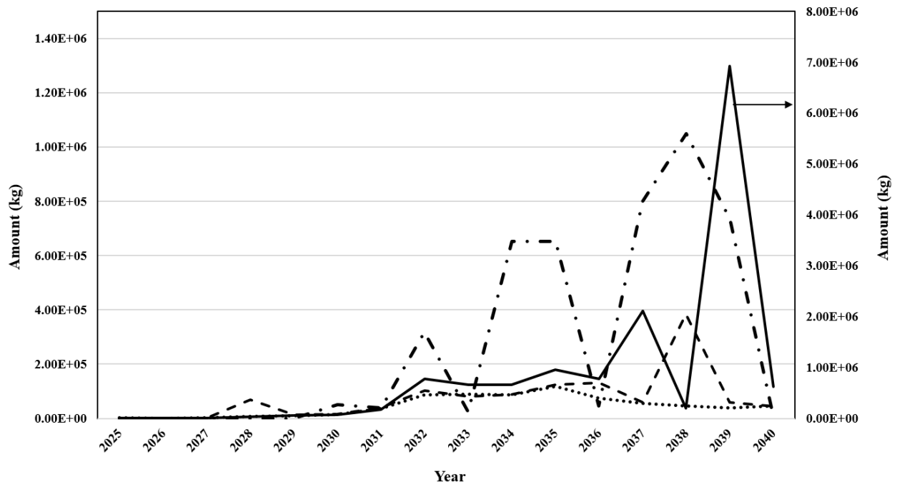
Figure 34. Aggregate disposal rates of steel from PV mounting structures across all scale for each island through 2040. Legend: O’ahu (solid line), Maui County (dashed line), Hawai’i County (dotted line), and Kaua’i (dashed-dotted line). For O’ahu, use right hand axis; for all other islands, use left hand axis.
