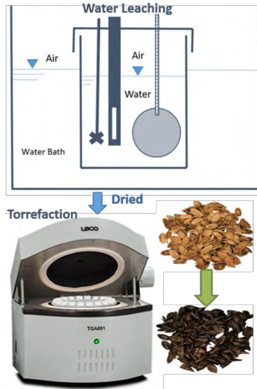
Figure 9. Laboratory scale leaching and torrefaction test equipment.
