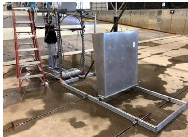
Figure 1. HNEI's HAWSEC system in Oregon State University's wave basin for testing.
