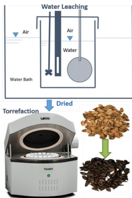
Figure 22. Laboratory scale leaching and torrefaction test equipment.
