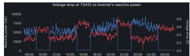
Figure 3. Voltage drop (red) is reduced when the advanced CVR controller is enabled, and reactive power (blue) is dispatched.
