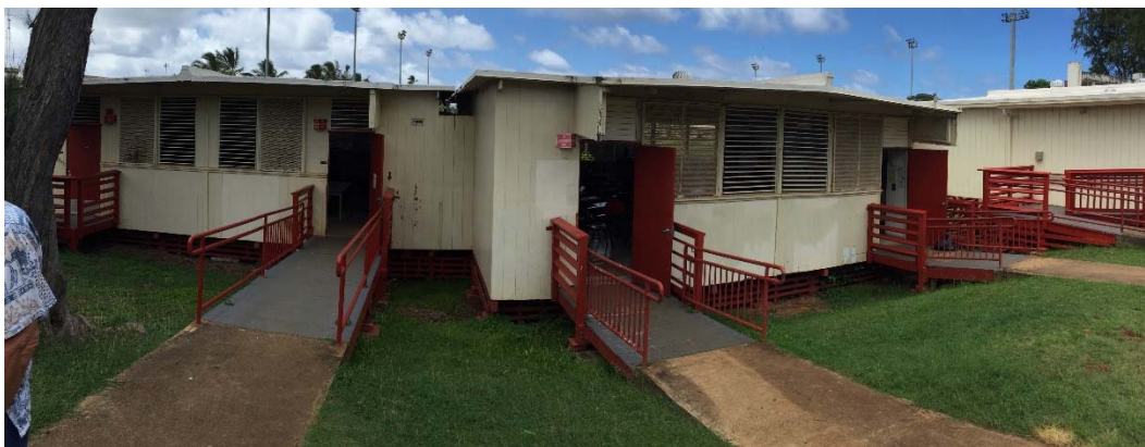
Figure 7.5.4: Some of the class rooms which were affected the most by mold growth and very high indoor temperatures. Typical indoor temperatures and R.H. for portables classrooms inspected: Air temperature range 85°F - 87°F, ceiling temperature range 84°F - 85°F, Wall temperature range 84°F - 85°F, R.H. 60% to 65%
