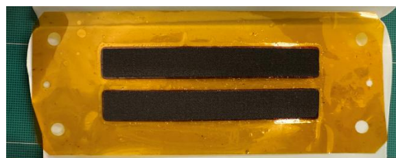
Figure 1. Demonstrated ability to fabricate a 2-cell membrane electrode assembly using flexible PCB technology.
