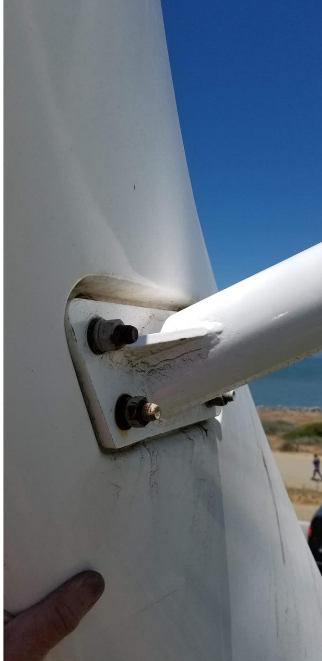
Figure 2. Rust on Blade bolts. We need to keep an eye on these. Consider replacing.
