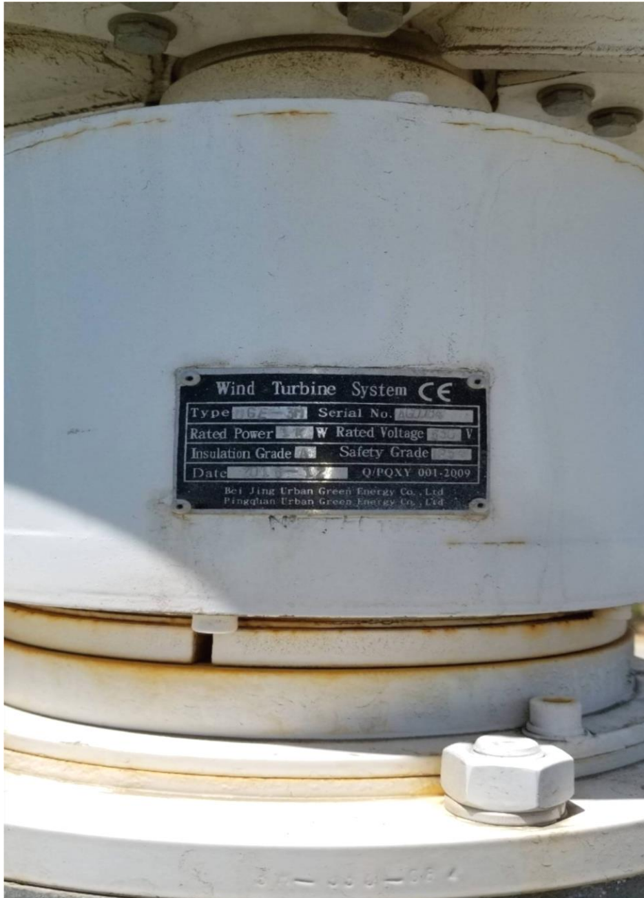
Figure 1. North UGE rust present at generator housing and flange
