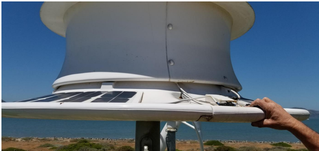
Figure 6. North Omniflow – replaced seized power generator.
