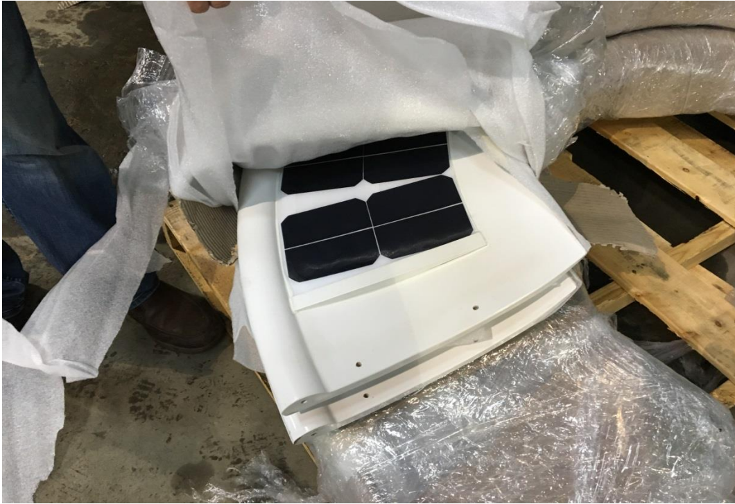
Figure 9: Omniflow Cowling with PV cells partially unpacked
