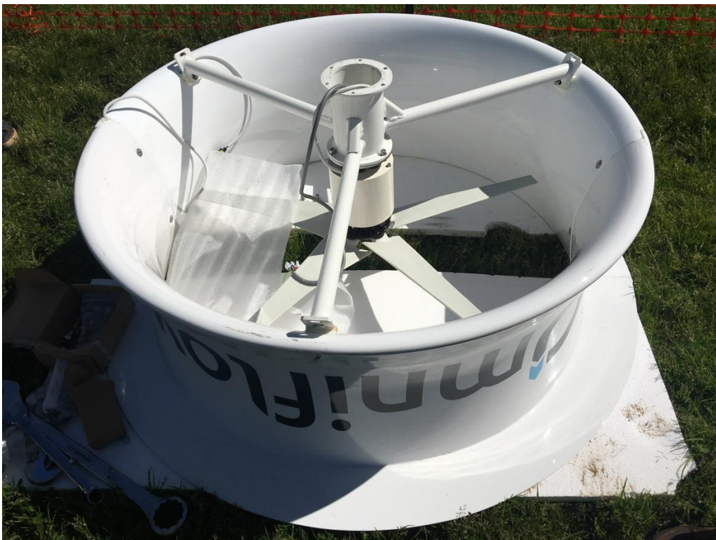
Figure 10: Omniflow main housing and rotor unpacked
