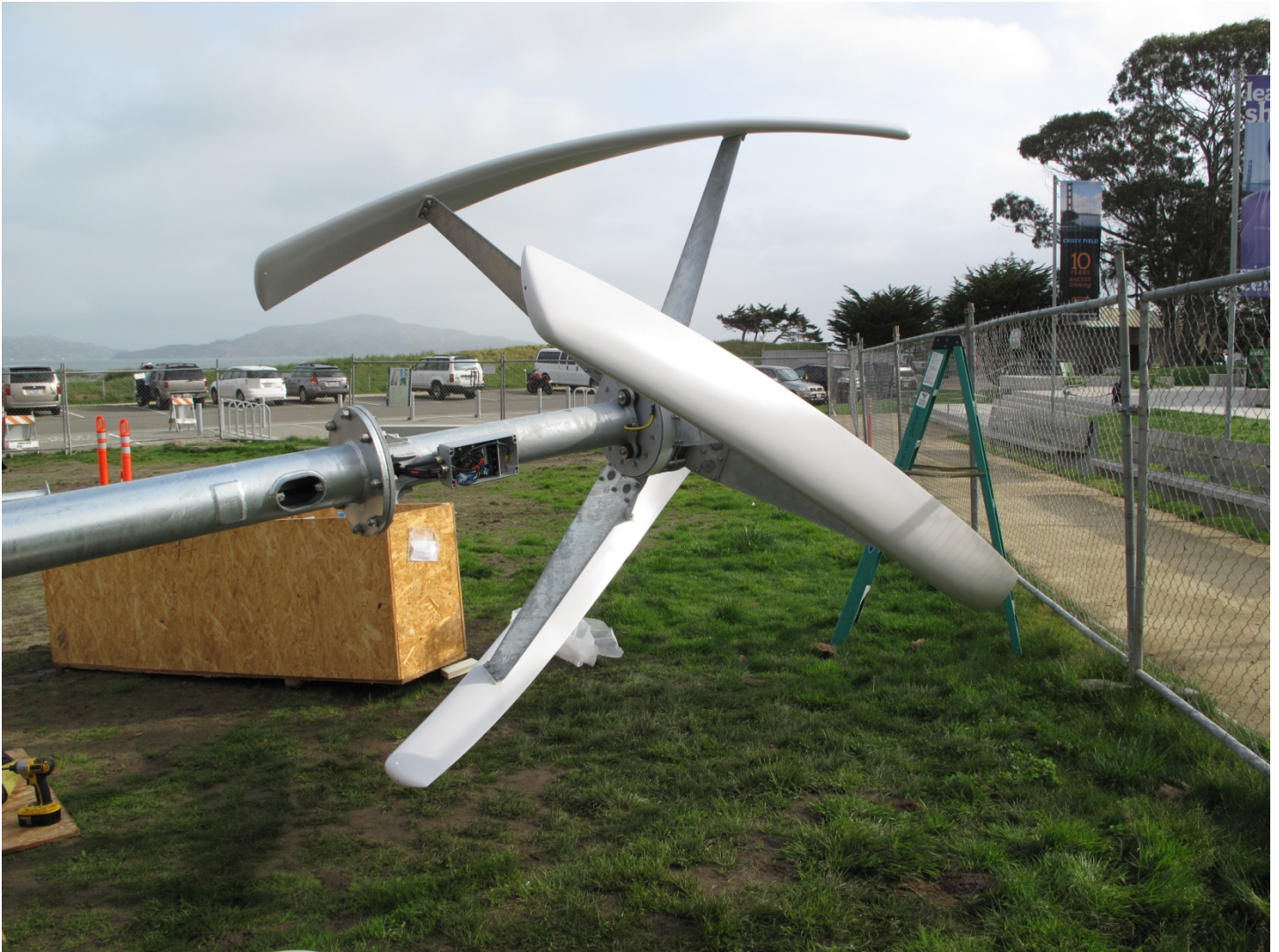
Venco unit mounted to its Tower
