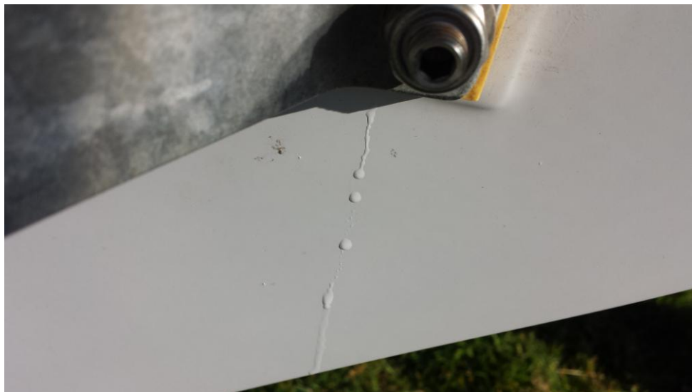
Figure 5: Water is lodged inside the blades on the South turbine even though weep holes on the bottom of the blade are clear.
