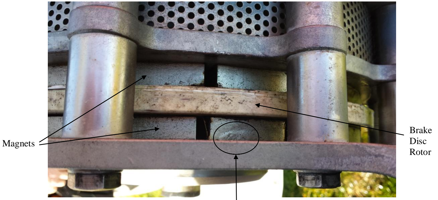
Figure 1: Plating Blistering on the Magnet
