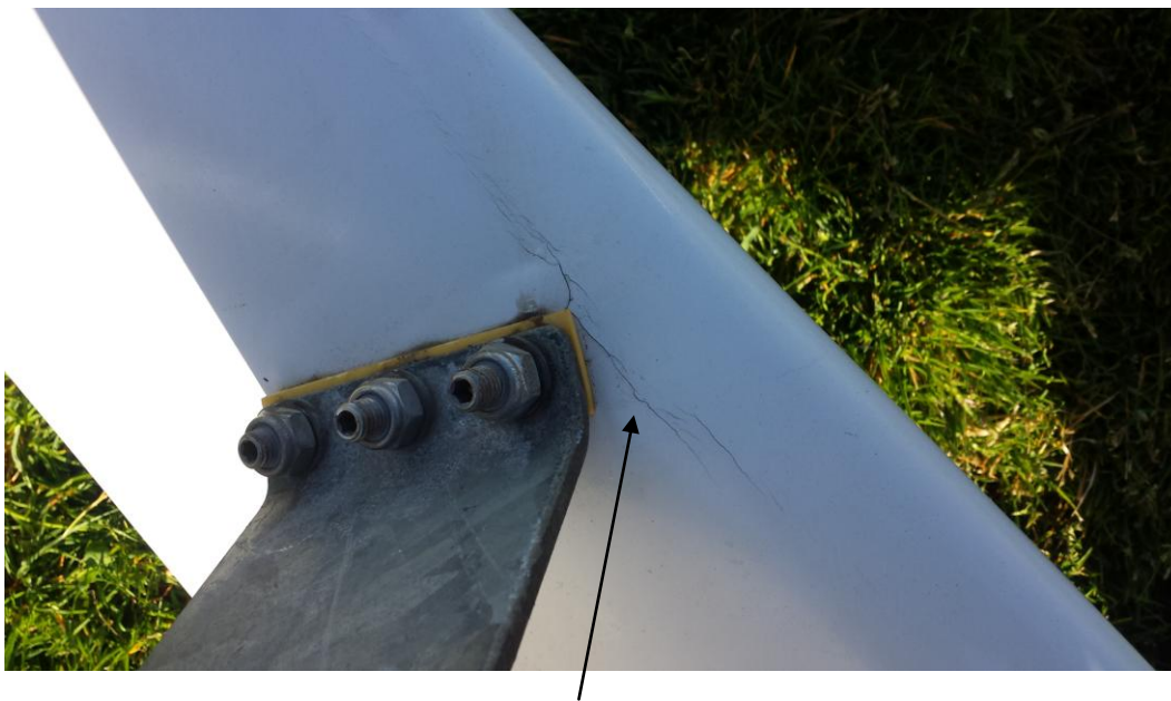
Figure 4: Stress cracks on one of the blades of the South turbine
