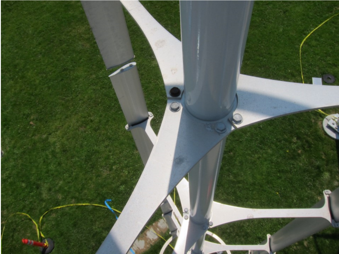
Figure 2. Northern Windspire. Some galvanized bolts were starting to rust on rotor flange connections. Cold galvanizing compound was applied.
