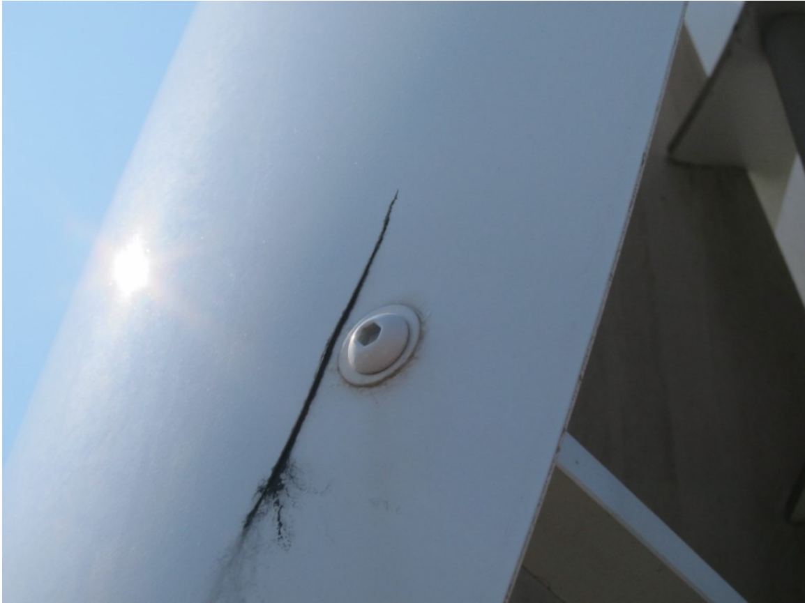
Figure 9. Tangarie. Blade crack.
