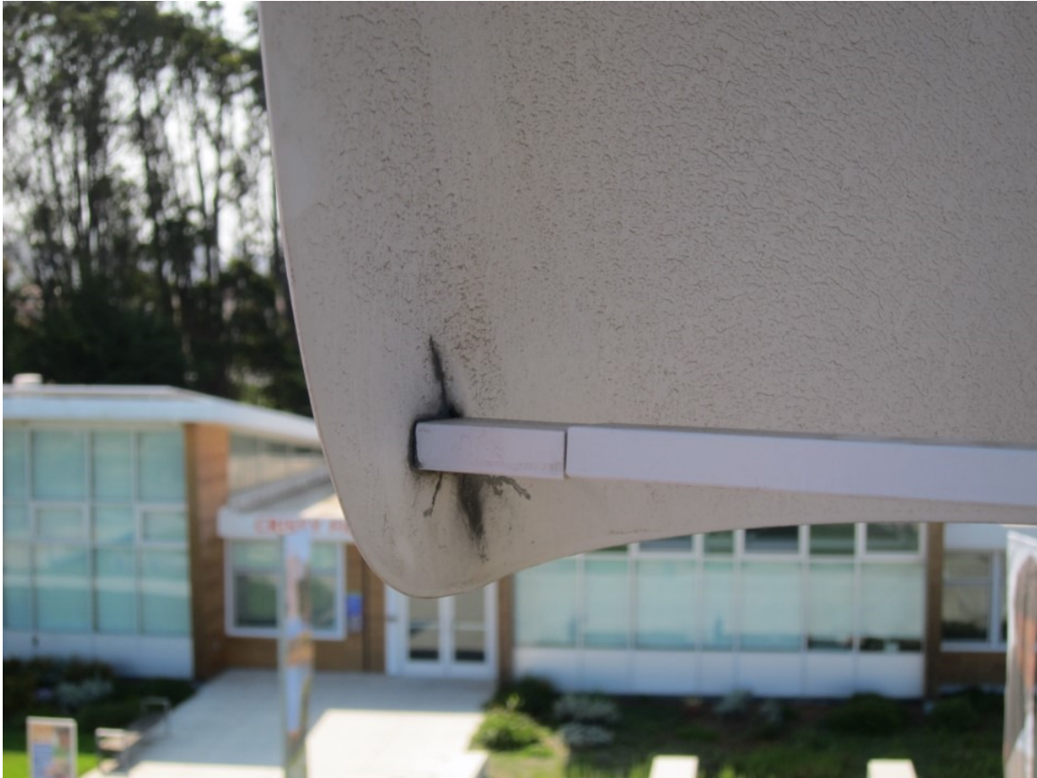
Figure 10. Tangarie. Blade crack.
