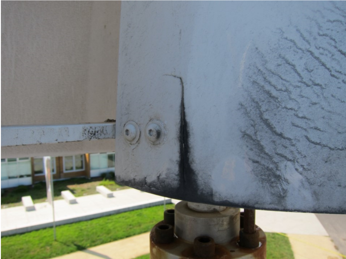
Figure 6. Tangarie. Lower blade crack.
