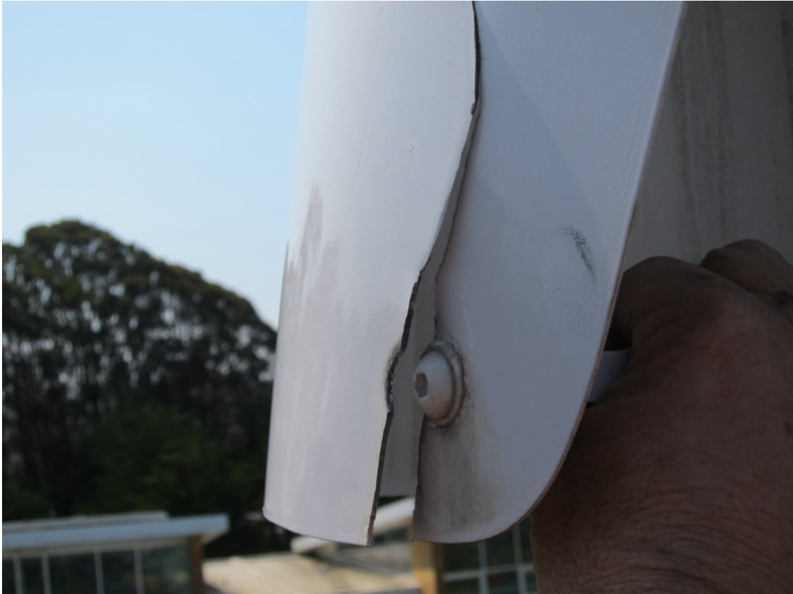
Figure 8. Tangarie. Lower blade crack.
