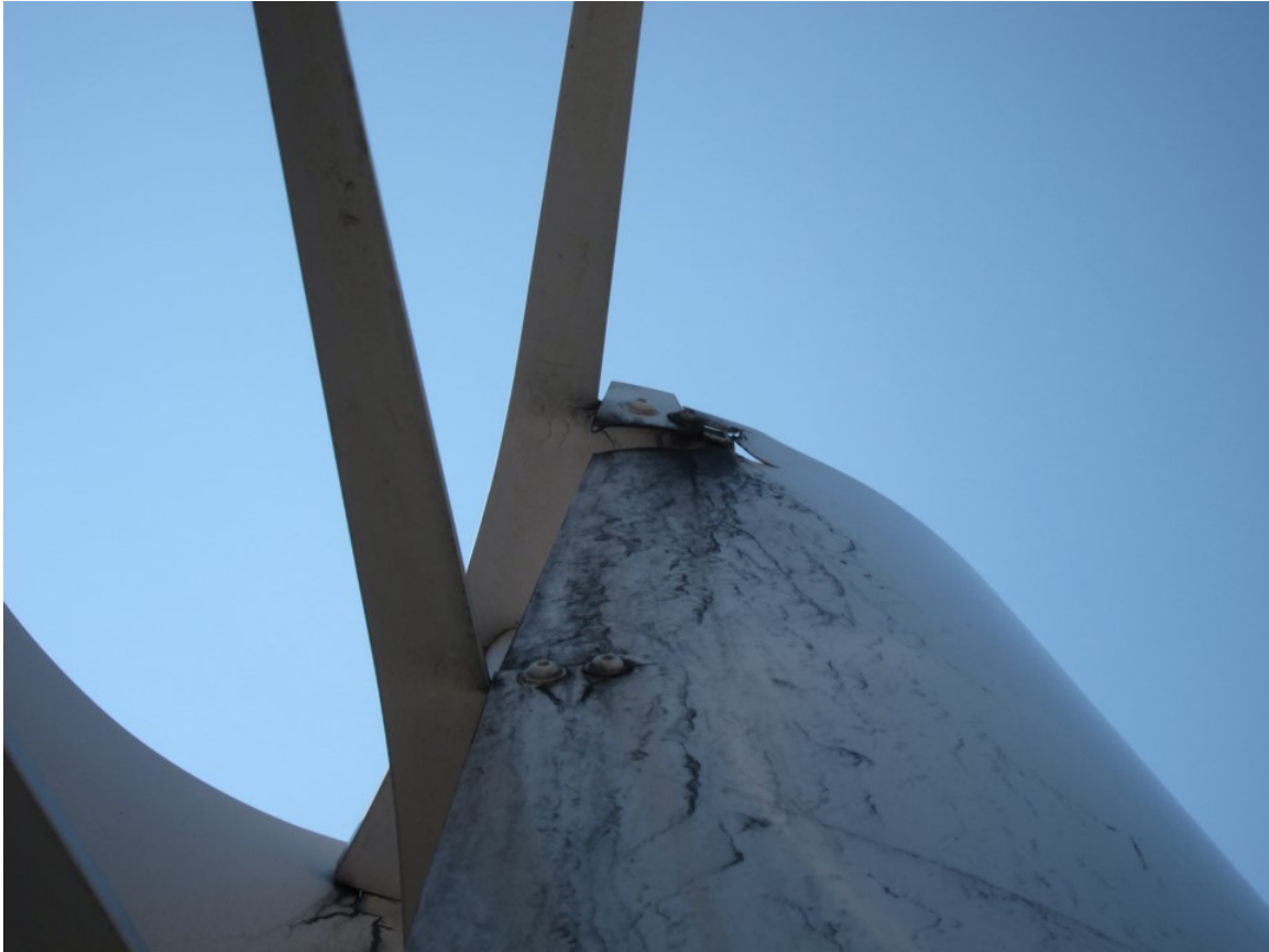
Figure 7. Tangarie. Upper portion of blade cracked and severed from strut.
