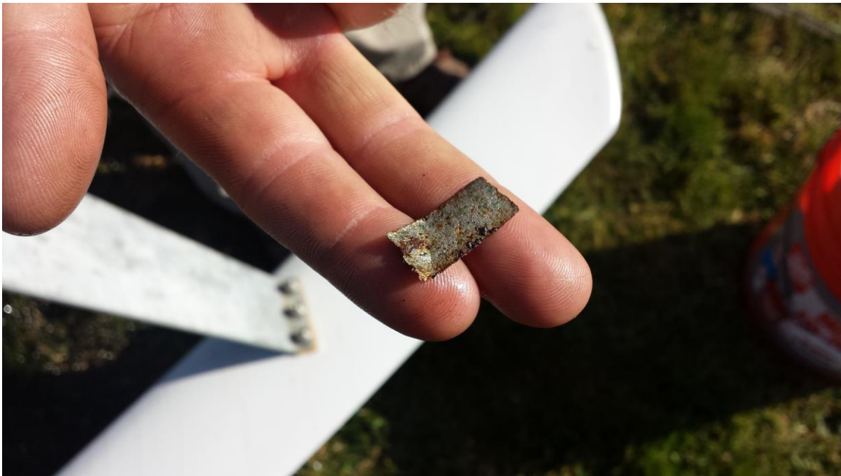
Figure 2: An example of the plating that has detached from the magnet
