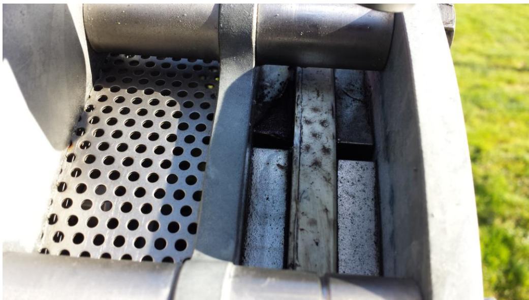
Figure 3: The plastic coating on the disc is becoming dislodged
