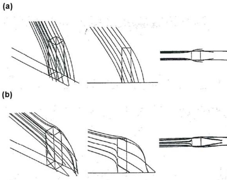
Fig. 2.2.K: Perspective, side and plan view of raindrop trajectories for (a) 5 mm radius raindrops and (b) 0.25 mm radius raindrops both in the 10 m/s flow field. (Blocken and Carmeliet ,2004)
