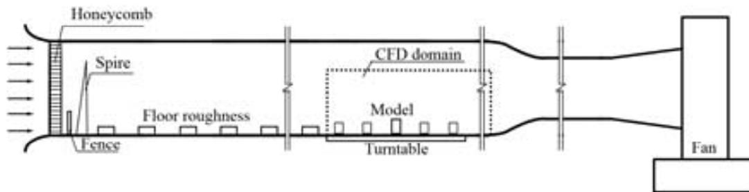
Figure 3.2.4.A Schematic of CFD domain in wind tunnel (Li and Ward, 2007)
