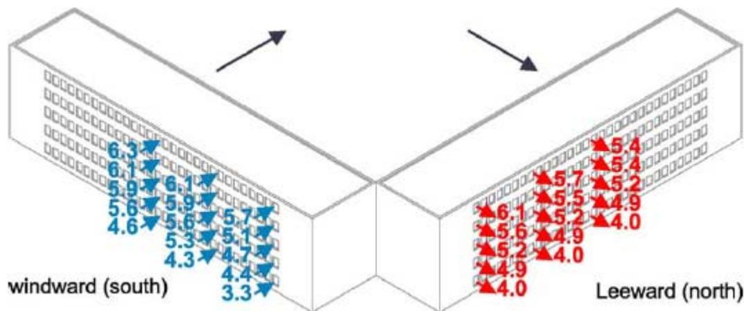
Fig. 2.2.L: ach results for a 4 m s<sub>-1</sub> normal wind in an open environment: whole building. (Moeseke and etal, 2005)
