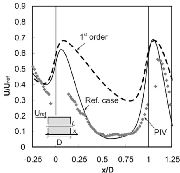
Figure 3.3.6.F: CFD simulation results for sensitivity analysis: impact of discretization scheme on the streamwise wind speed ratio along the centerline. For the reference case, a second-order discretization scheme is used. (Ramponi and Blocken, 2012).
