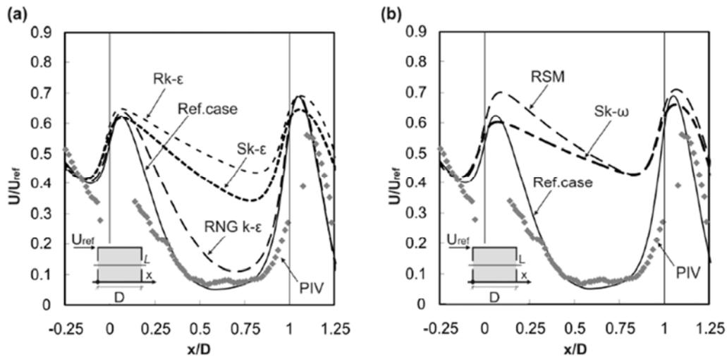
Figure 3.3.1.C: CFD simulation results for sensitivity analysis: impact of turbulence models on the streamwise wind speed ratio along the centerline. Comparison between the reference case (Ref.case = SST k- $\omega$  model) and (a) the k- $\epsilon$  models and (b) the RSM and standard k- $\epsilon$  model.
