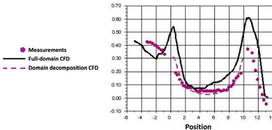
Figure 3.1.4.F: Velocity ratio  $V_X/V_{ref}$  along line joining inlet and outlet openings for Case C (Meroney, 2009) modified
