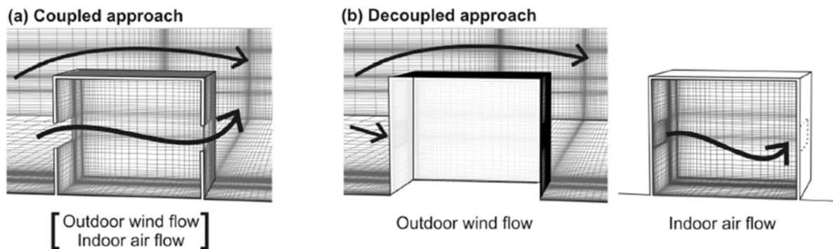
Figure 3.1.4.A: (a) Coupled and (b) decoupled approach for analysis of wind-induced cross-ventilation of buildings (Ramponi and Blocken (2012))
