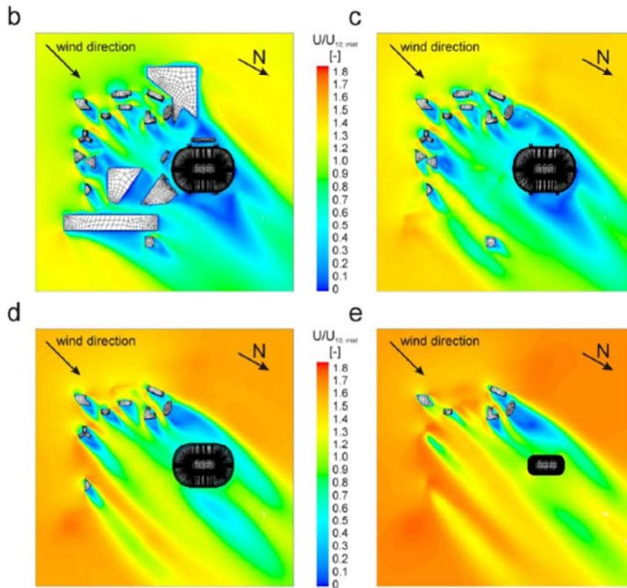
Figure 3.1.4.E: Contours of non-dimensional velocity magnitude  $U/U_{10}$  in four horizontal planes at different heights (VanHoff and Blocken, 2010a; modified)
