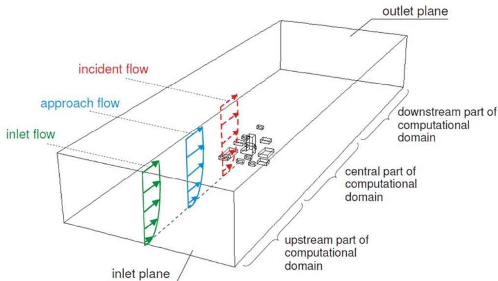
Figure 3.2.4.E Computational domain with building models for CFD simulation of ABL flow – definition of inlet flow, approach flow and incident flow and indication of different parts in the domain for roughness modeling (Brocken et al, 2007)
