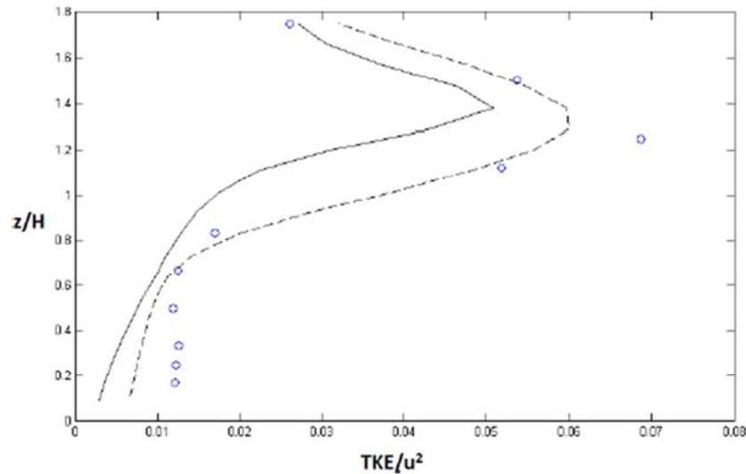
Figure 3.3.1.B: Normalized TKE profiles from CFD model with un-modified constants (black line), modified constants (dashed line) and wind tunnel data (circles)
