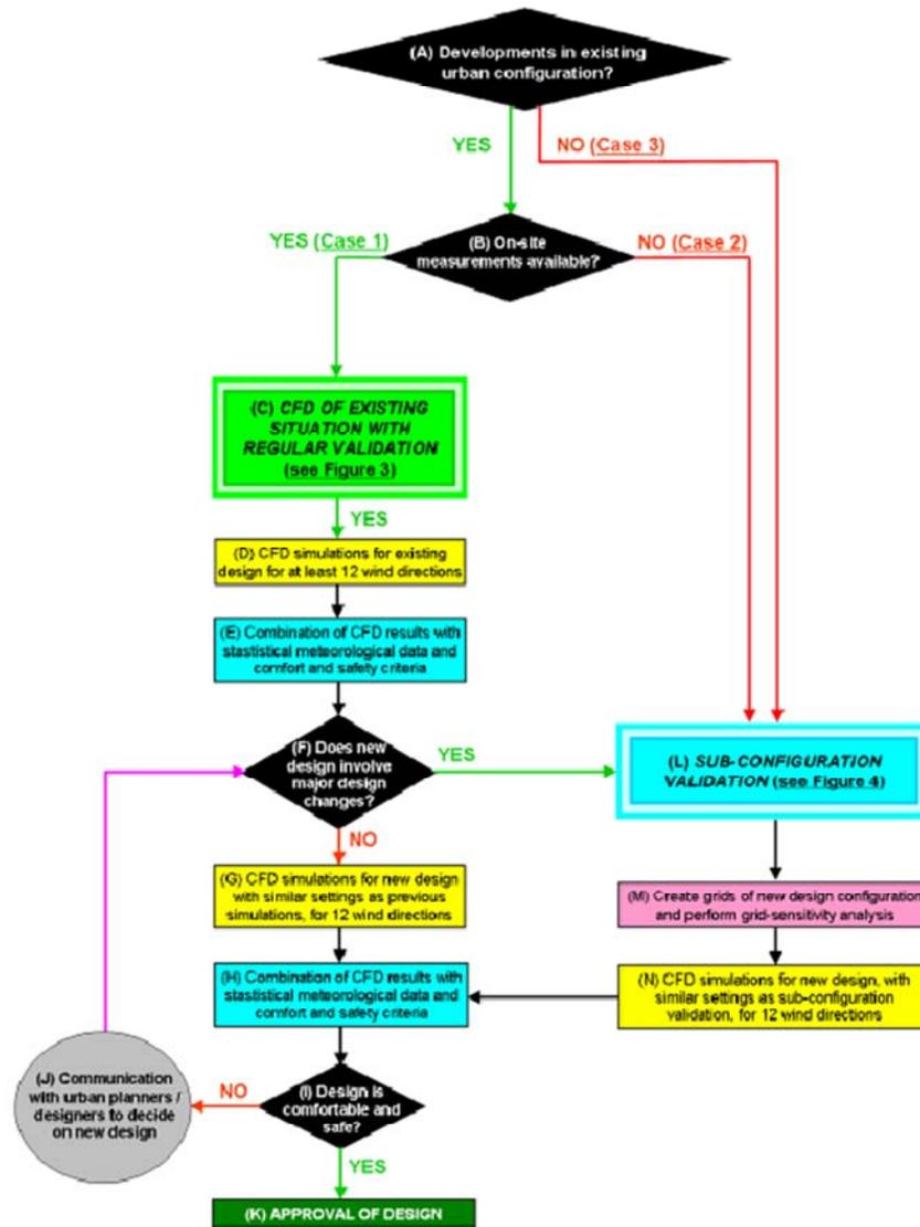
Figure 3.1.3.B: Flowchart illustrating the framework for the assessment of pedestrian wind comfort and safety with CFD for Case 1 (Blocken et al, 2012)
