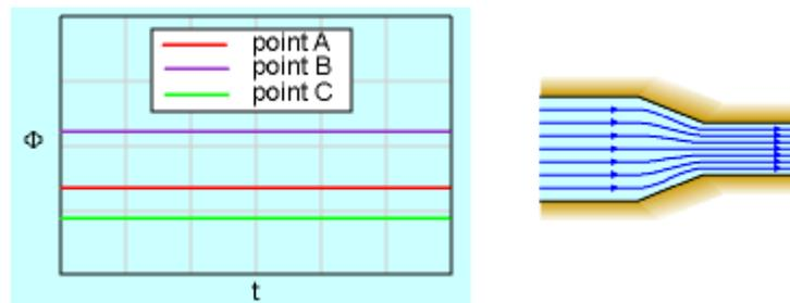
Figure 3.3.2.A: Steady flow: (a) Steady Flow (b) Flow with changing velocity
