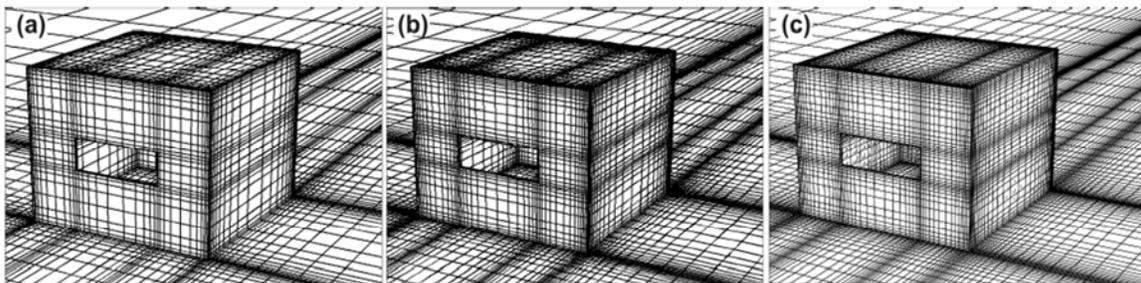
Figure 3.3.6.C: Perspective view of grids for grid-sensitivity analysis: (a) Coarse grid A with 144,696 cells; (b) Middle grid B with 314,080 cells; (c) Fine grid C with 575,247 cells (reference case). (Ramponi and Blocken, 2012).
