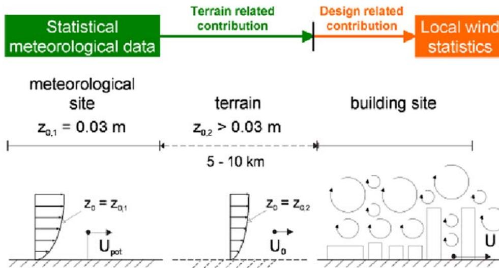
Figure 3.1.3.A: Transformation of statistical meteorological data from the meteorological site to the building site (Blocken et al, 2012)
