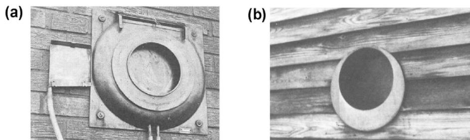
Fig. 2.2F: (a) Two gauges with the collection area fitting flush into the wall and (b) The recessed gauge designed (Blocken and Carmeliet ,2004)
