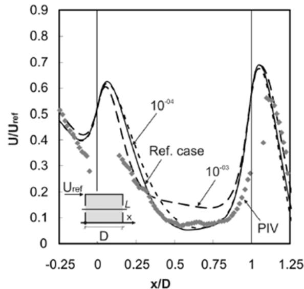
Figure 3.3.6.I: CFD simulation results for sensitivity analysis: impact of iterative convergence limit on the streamwise wind speed ratio along the centerline. The convergence for the reference case is assumed when all the scaled residuals leveled off and reached a minimum of  $10^{-6}$  for  $x$ ,  $y$  and  $z$  momentum,  $10^{-5}$  for  $k$  and  $10^{-4}$  for  $\omega$  and continuity. (Ramponi and Blocken, 2012).
