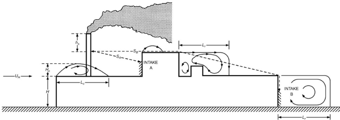
Figure 1.1.J: Flow Recirculation Regions and Exhaust-to-Intake Stretched-String Distances (ASHRAE, Chapter 16, 2005)
