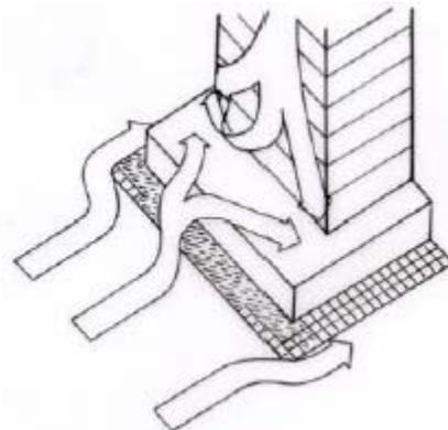
Figure 1.2.G (Left): A large canopy as a solution to the pedestrian-wind problem
