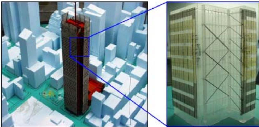
Figure 3.2.3A: Case Study I Wind Tunnel Models (a) 1:400 Scale (left) and (b) 1:50 Scale (right). (Browne and etal, 2007)
