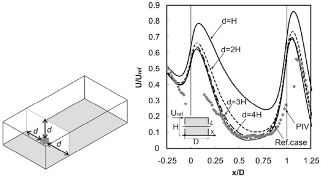
Figure 3.3.6.B: CFD simulation results for sensitivity analysis: impact of the size (cross-section) of the computational domain on the streamwise wind speed ratio along the centerline (Ramponi and Blocken, 2012).
