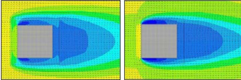
Figure 3.2.3C: Velocity Field and Pressure Contours from CFD Simulation (a) with a 50% porous screen (left), and (b) without screen (Browne and etal, 2007)
