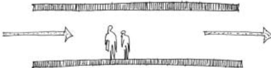
Figure 1.1F: Sketch of cross ventilation. As a rule of thumb, cross-ventilation is effective up to 5 times the floor to ceiling height. (Kleiven, 2003)
