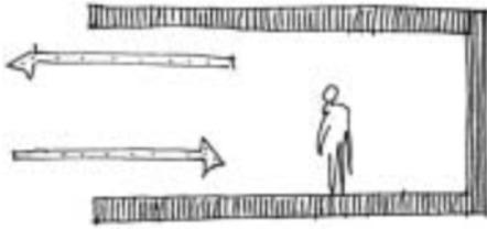
Figure 1.1E: Sketch of single sided ventilation. As a rule of thumb, single-sided ventilation is effective to a depth of about 2 – 2.5 times the floor to ceiling height. (Kleiven, 2003)
