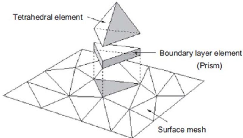
Figure 3.1.3.E Arrangement of grid elements near solid surface in unstructured grid. (Tominaga et al, 2008)
