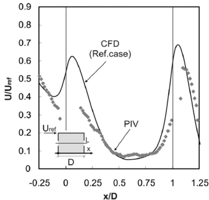
Figure 3.1.4.C: Comparison of experimental (PIV) and reference CFD case for the streamwise wind speed ratio  $U/U_{ref}$  along the centerline.
