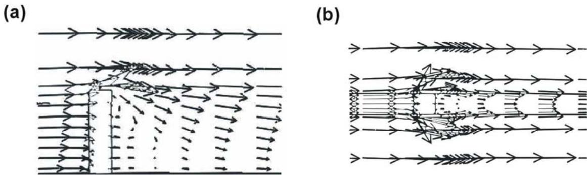
Fig. 2.2.J: Wind flow pattern around a building ( $10 \times 10 \times 40 \text{ m}^3$ ) calculated with Stead-state CFD simulation by using standard  $k-\epsilon$  turbulence model.
