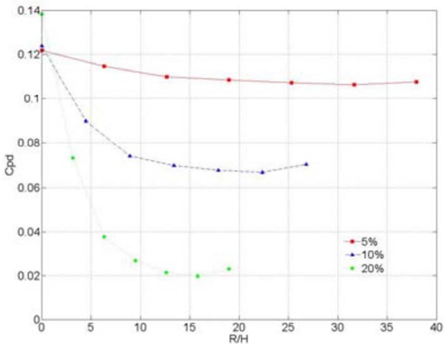
Figure 3.2.4.C Example of the effect of fetch on the pressure coefficient difference– staggered pattern (Li and Ward, 2007)
