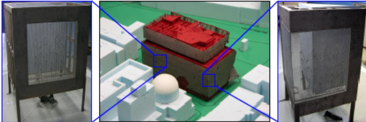
Figure 3.2.3B: Case Study II Wind Tunnel Models (a) 1:200 Scale (centre), (b) Full-Scale Prototype of Central Wall Condition (left), (c) Full-Scale Prototype of Corner Condition (right). (Browne and etal, 2007)
