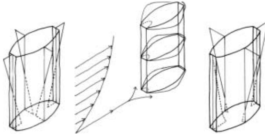
Figure 1.1D: The buoyancy-induced pressure distribution upon the envelope of a high-rise building with an oval shape. (Kleiven, 2003)
