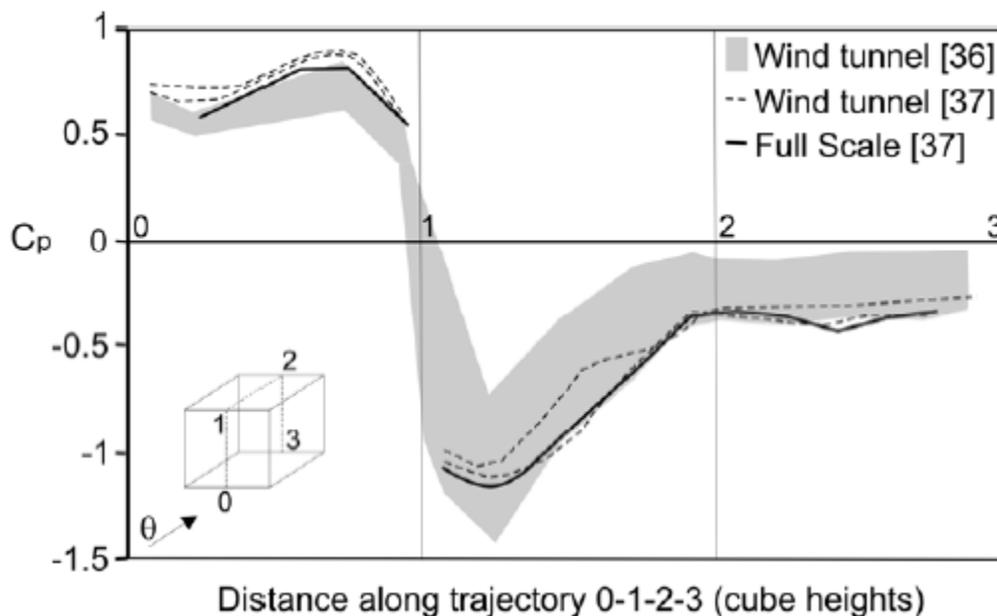
Figure 2.1.K: Comparison of different wind tunnel experiments (Cóstola and etc., 2009)
