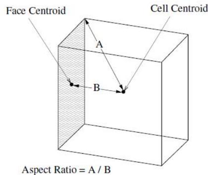
Figure 3.2.2.A: The aspect ratio for a unit cube (ANSYS, 2009)
