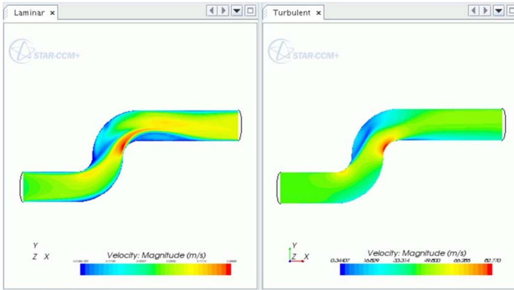
Figure 3.4.D. Multiple snapshot from different design scenarios for comparing the resulting data (STAR-CD+)
