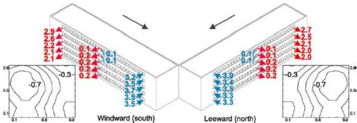
Fig. 2.2.N: Pressure coefficients obtained with M. Grosso’s model (left and right) and ach results (centre) for a 4 m s<sub>-1</sub> 908 incident wind in an open environment (Moeseke and etal, 2005)
