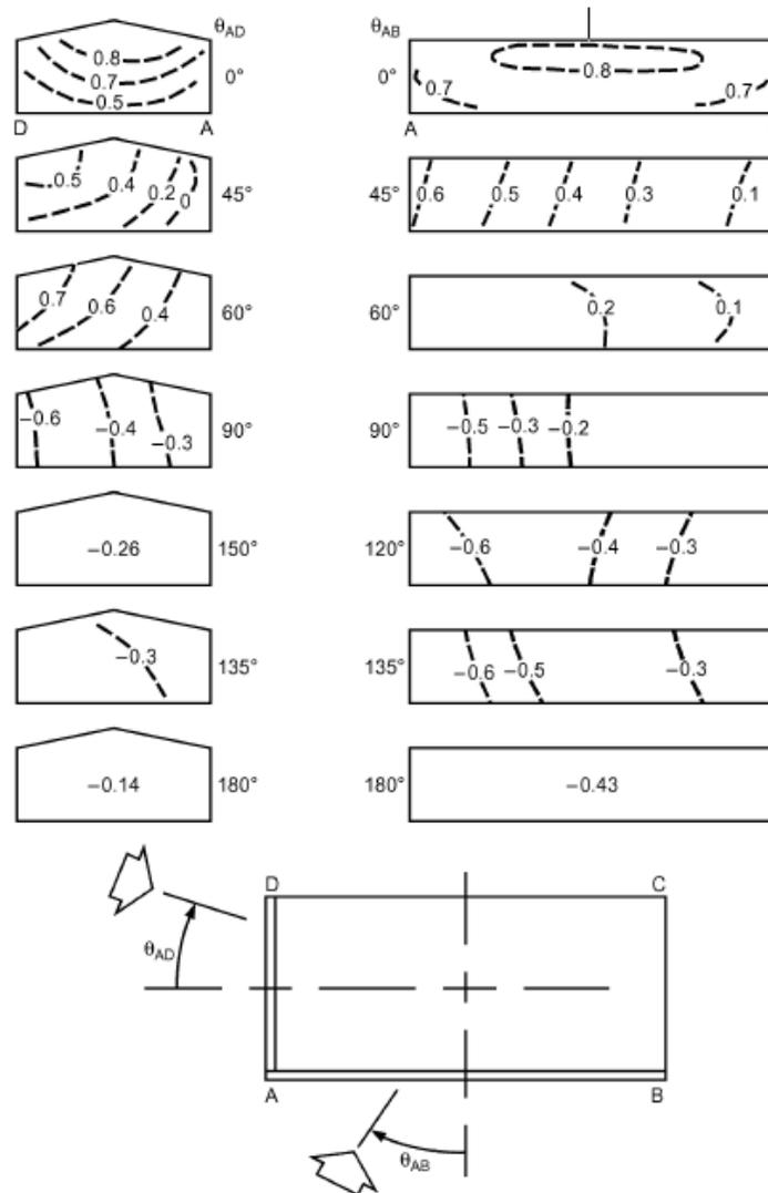
Figure 1.1.L: Local Pressure Coefficients for Walls of Low-Rise Building with Varying Wind Direction (ASHRAE, Chapter 16, 2005)
