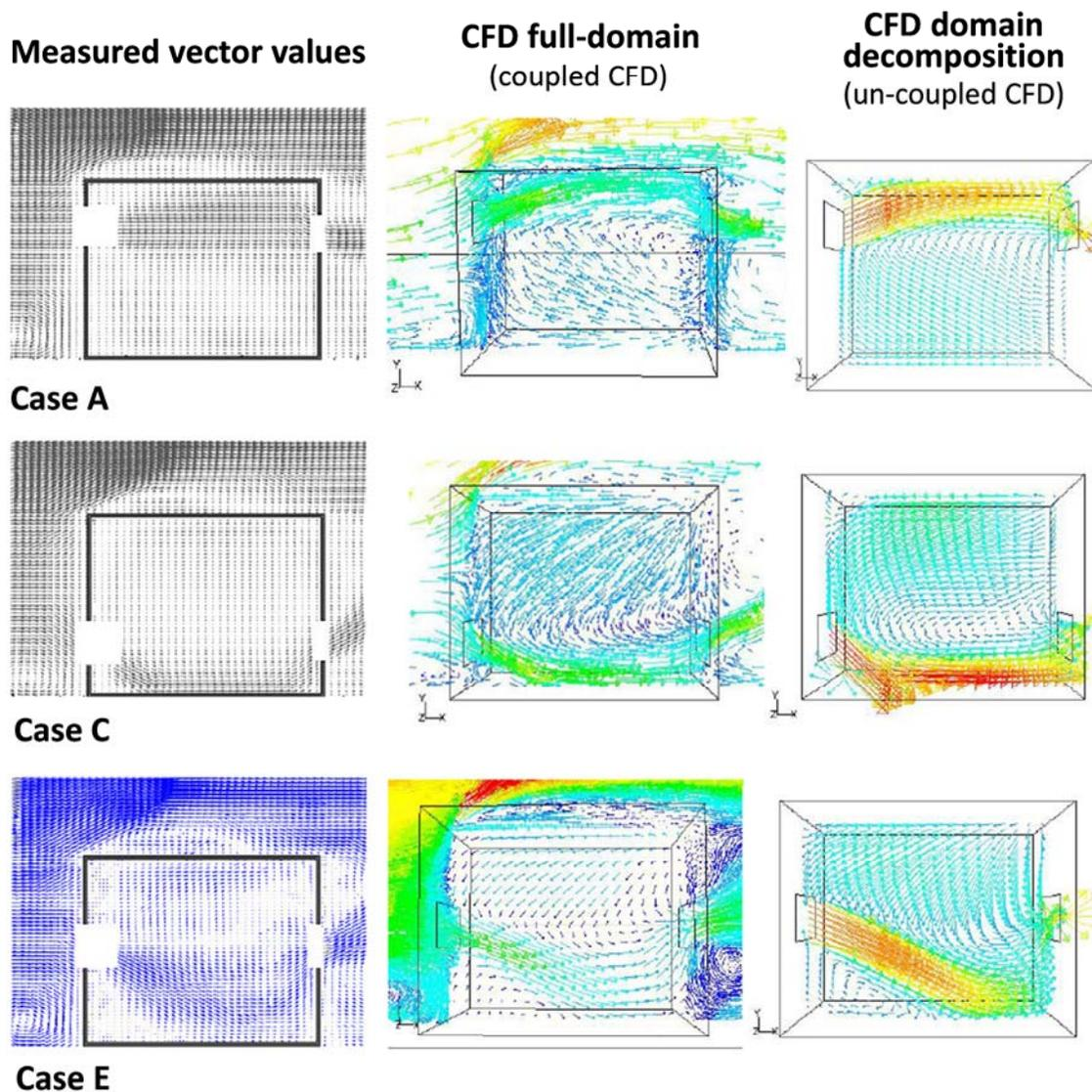
Figure 3.1.4.E: Velocity vectors on building vertical midplane for three case Cases, obtained from measured air flow and coupled and uncoupled flow domains (Meroney, 2009; modified)
