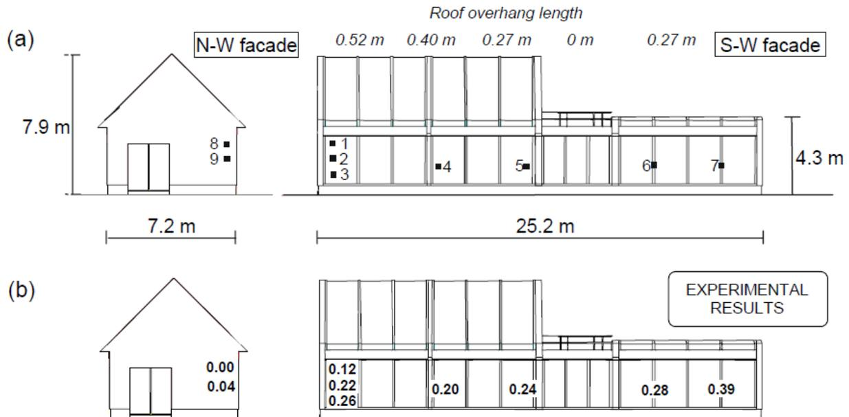
Fig. 2.2.H: (a) North-west and south-west facade. Building dimensions, roof overhang length, positions and numbers (1-9) of wind-driven rain gauges. (b) Spatial distribution of measured catch ratio values at the end of the rain event given in estimated measurement error: 0.04. Multiply catch ratio values with  $Sh = 24.8$  mm to obtain the wind-driven rain amount. (Blocken and Carmeliet, 2004)
