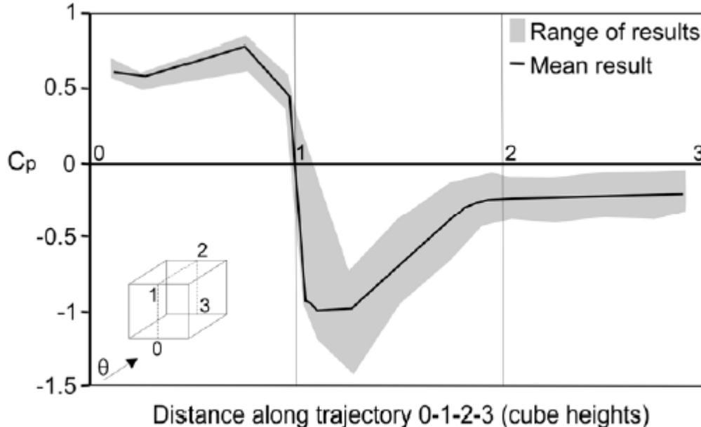
Figure 2.1.L: Comparison of different wind full scale results (Cóstola and etc., 2009)
