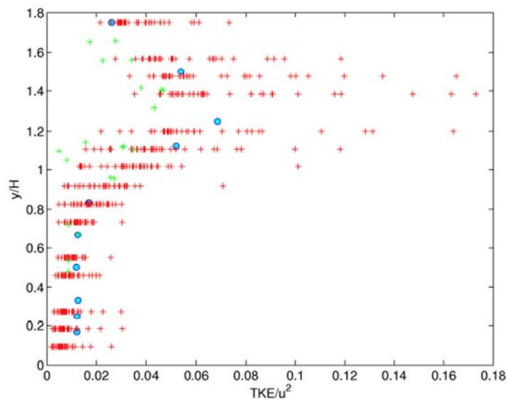
Figure 3.3.1.A: Normalized TKE (e.g. turbulence kinetic energy) data from wind tunnel (blue circles) and CFD simulation (crosses) against normalized by the height  $h$  of the buildings. (Glover et al, 2006)
