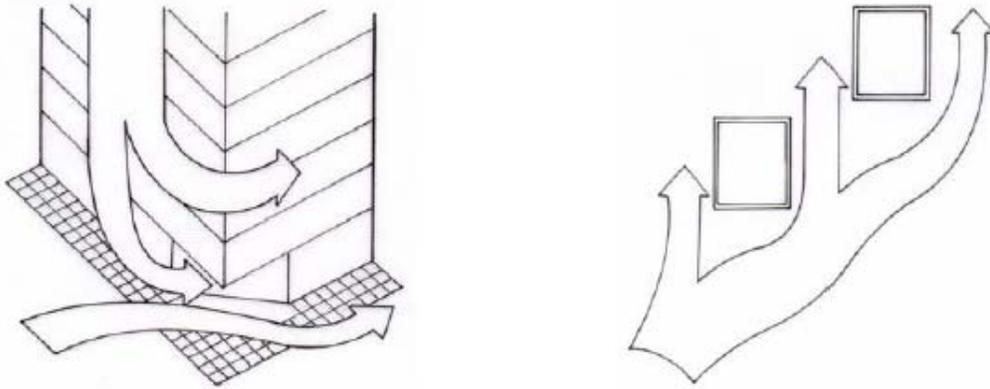
Figure 1.2.K (Left): Accelerated corner flow from downwash
