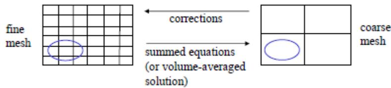
Figure 3.3.4E: Coarse mesh calculations (Bakker, 2006)
