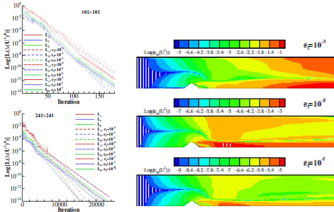
Figure 3.3.4G (Left): Convergence history of  $U_1$  for the flow around a two-dimensional hill.  $101 \times 101$  and  $241 \times 241$  grids.  $Rn = 60000$ , (Eca, 2006 )
