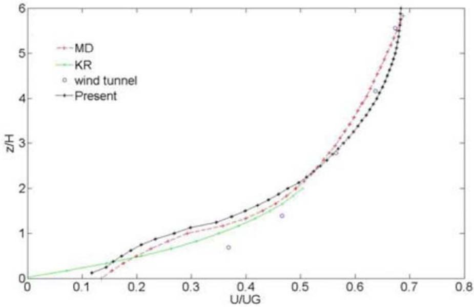
Figure 3.2.4.B Mean velocity profile in urban roughness elements region(Li and Ward, 2007)
