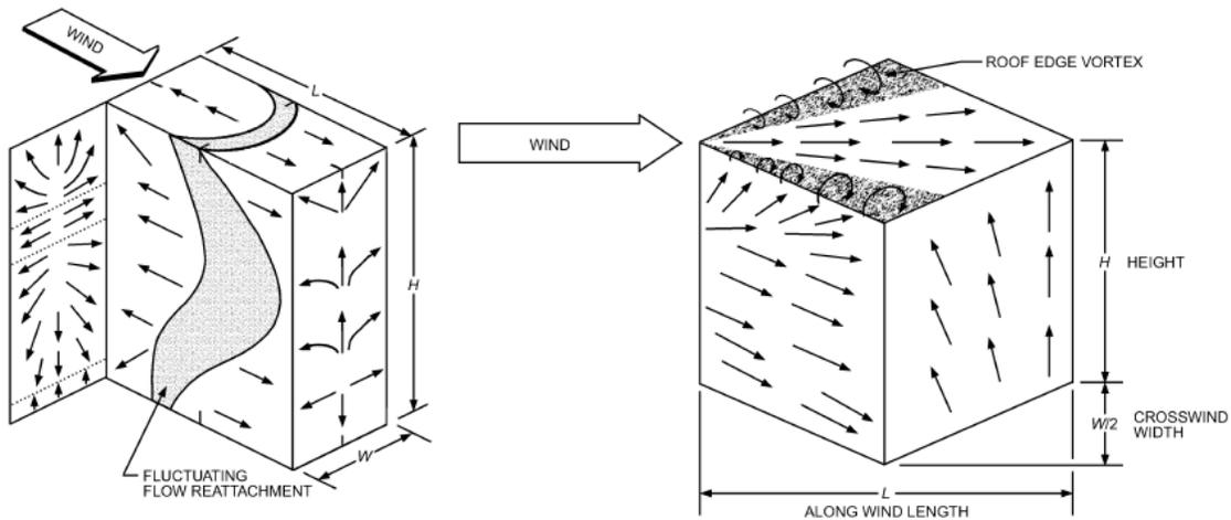
Figure 1.1I: Surface Flow Patterns and Building Dimensions (ASHRAE, Chapter 16, 2005)
