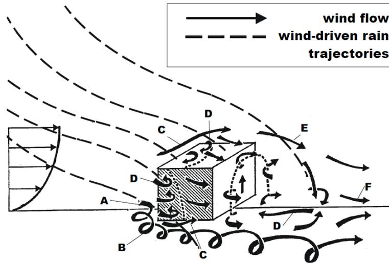
Fig. 1.2.B: A representation of the wind flow pattern around a building and of raindrop trajectories in the wind flow pattern. The flow pattern includes a frontal vortex (A), corner streams (B), separation at building corners (C), recirculation zones (D), shear layers (E) and a far wake (F) (Blocken and Carmeliet, 2004)
