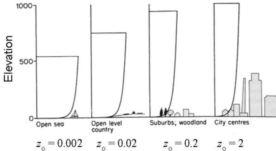
Figure 1.3.A: Mean wind profiles for different terrains (Mendis and etc, 2007)
