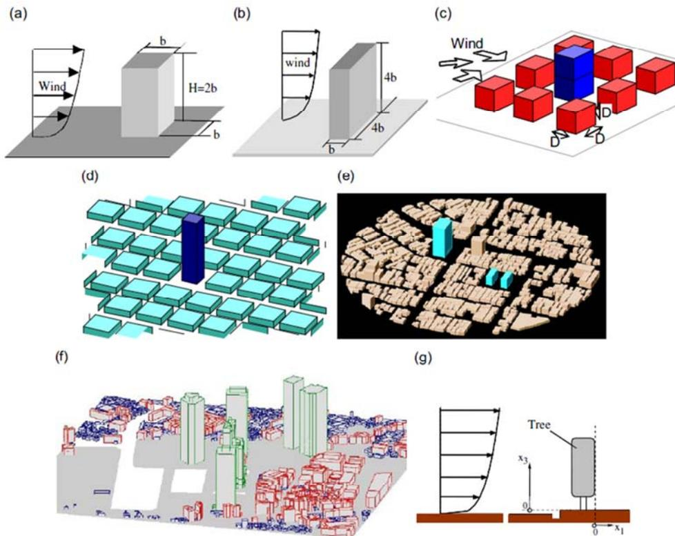
Figure 3.1.3.C: Seven test cases for cross-comparison. (a) Test case A (2:1:1 square prism); (b) Test case B (4:4:1 square prism); (c) Test case C (Simple city blocks); (d) Test case D (High-rise building in city); (e) Test case E (Building complexes with simple building shapes in actual urban area); (f) Test case F (Building complexes with complicated building shapes in actual urban area); (g) Test case G (Two-dimensional pine tree).
