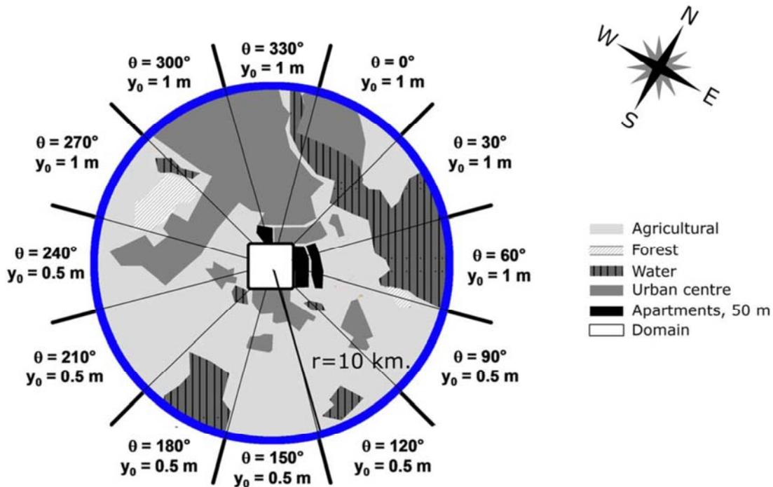
Figure 3.2.1A: Terrain surrounding the stadium with a radius of 10 km and estimated aerodynamic roughness lengths  $y_0$ . The white square represents the computational domain used in this study (Blocken and Person, 2009).
