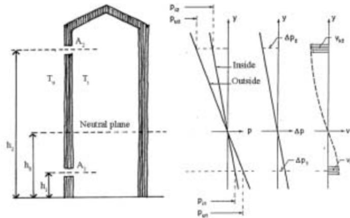
Figure 1.1B: Thermal buoyancy in a space with two openings. (Kleiven, 2003)
