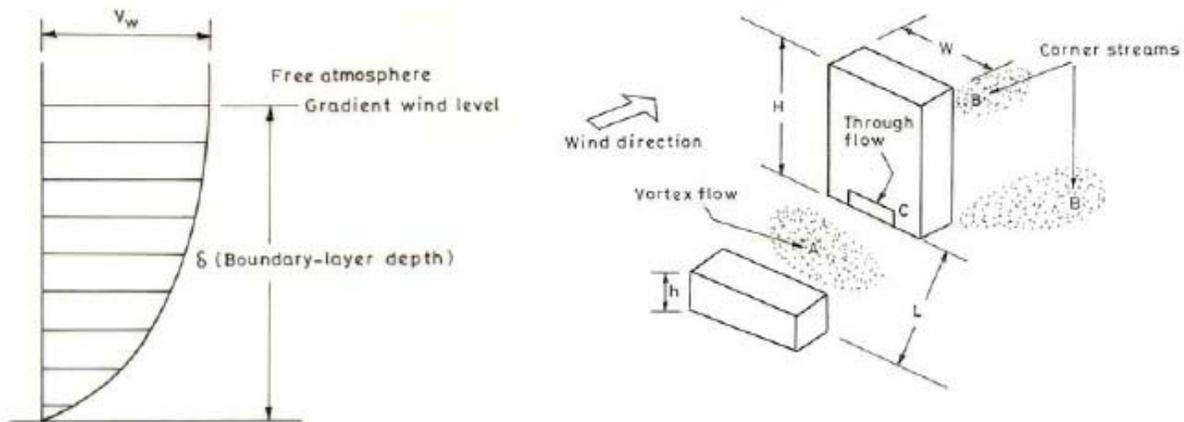
Figure 1.2.C (Left): The atmospheric boundary layer and
