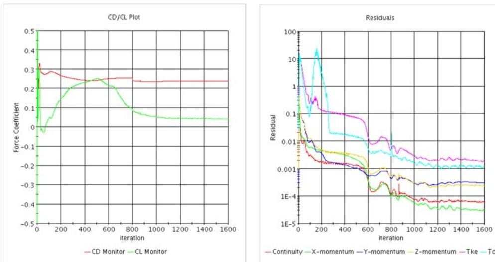
Figure 3.3.5.A: Monitor-based stopping criteria can be used to stop the simulation when an appropriate level of convergence has been reached, based on an appropriate combination of residual monitors or monitors of other physical quantities (CD-adapco, 2013).
