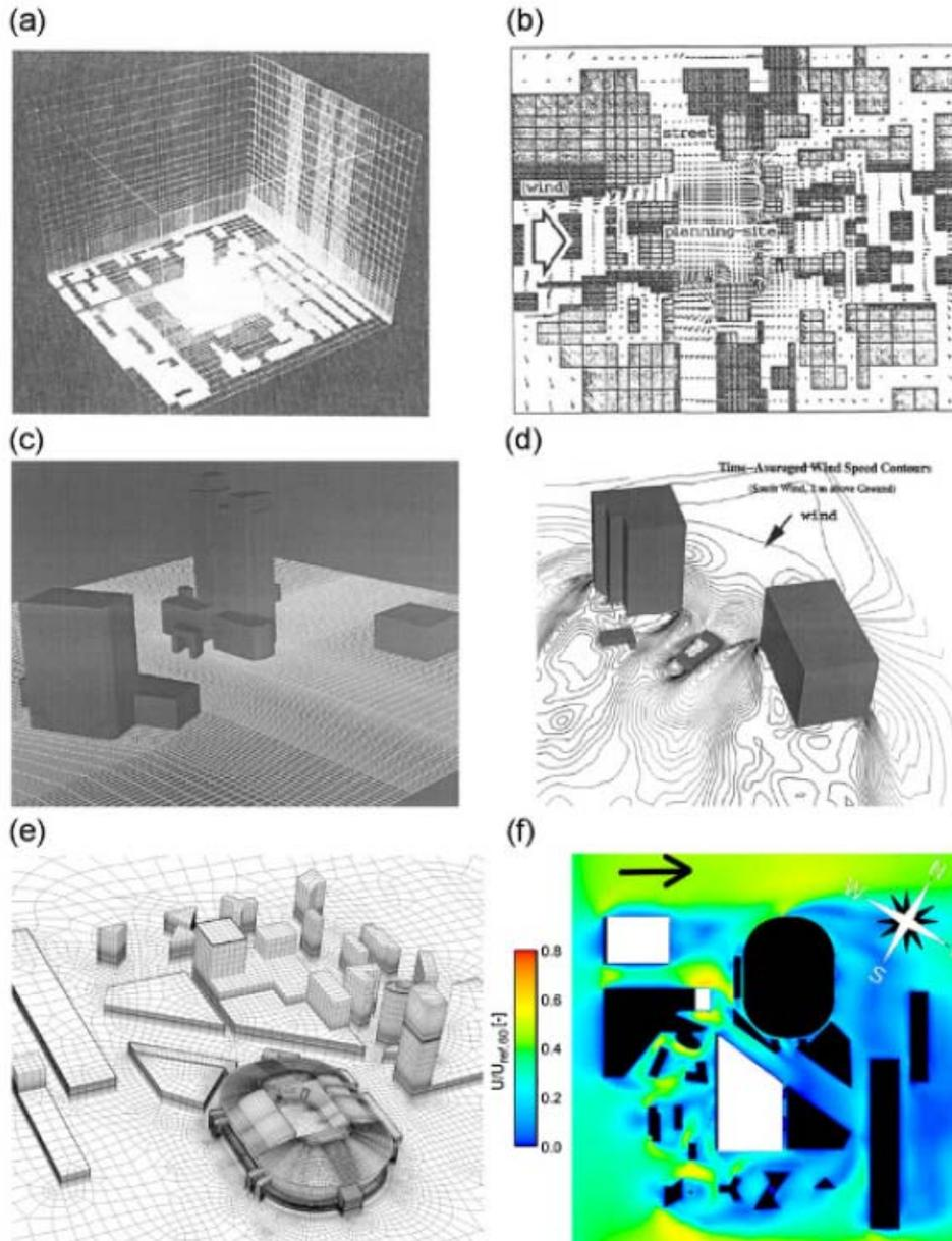
Figure 3.1.2.A: Examples of CFD studies of pedestrian-level wind environment in urban areas: (a-b) Grid (finite elements) and wind-velocity vectors based on steady RANS simulations, (c-d) Grid (total cell count unknown) and wind speed contours based on, (e-f) Grid (2.8 million cells) and wind speed ratio contours, based on steady RANS (Blocken and etal, 2011).
