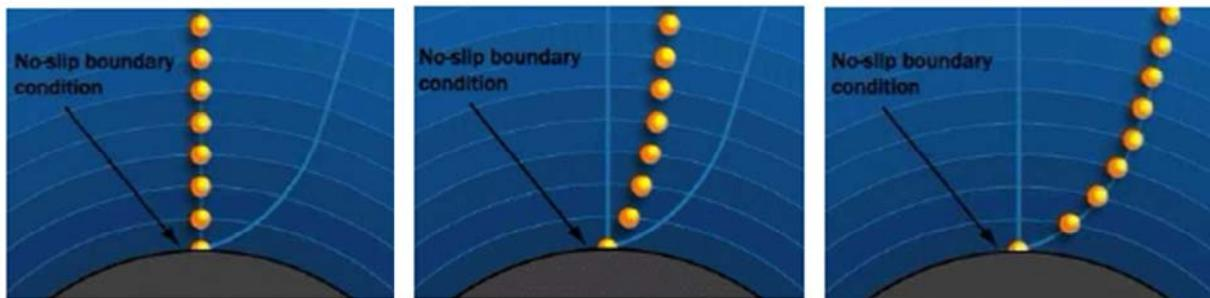
Figure 3.3.3D: No-slip wall (Bakker, 2006)
