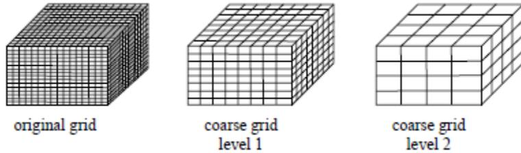
Figure 3.3.4D: Fine meshes (Bakker, 2006)
