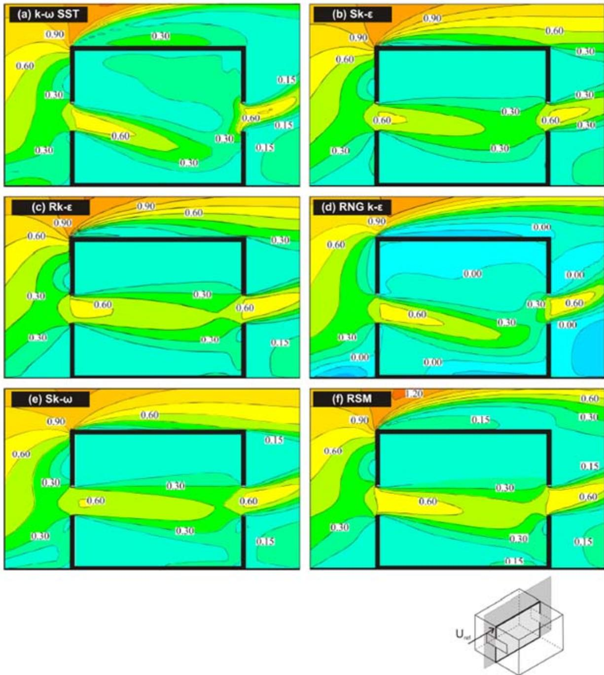
Figure 3.3.6.H: CFD simulation results for sensitivity analysis: impact of turbulence models on the wind speed ratio contours in the vertical centerplane. The SST  $k-\omega$  model is the reference case in this study. (Ramponi and Blocken, 2012).
