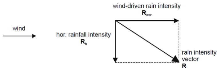
Fig. 1.2.A: Rain intensity vector  $R$  and its components: wind-driven rain intensity  $R_{wdr}$  and horizontal rainfall intensity  $R_h$  (Blocken and Carmeliet, 2004)
