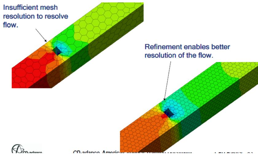
Figure 3.3.4F: Grid Generation Guidelines (CD-adapco, user manual )
