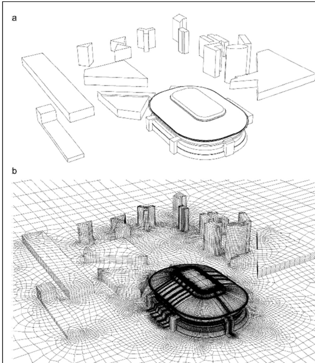
Figure 3.1.4.D: (a) Computational model geometry, view from northeast; (b) Computational grid on the building surfaces and part of the ground surface. A high resolution is used in the proximity of the stadium, and a lower resolution at a larger distance from the stadium. (VanHoff and Blocken, 2010a)
