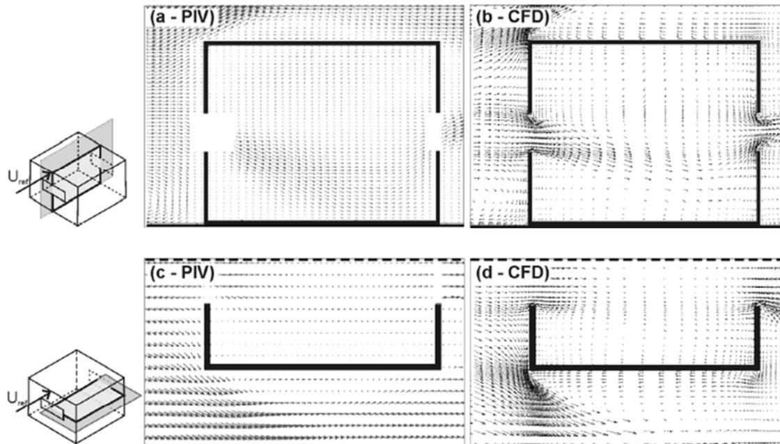
Figure 3.1.4.B: Comparison of the velocity vector fields obtained with the PIV measurements and the CFD reference simulation case in the vertical centerplane and in the horizontal plane at mid-height through the openings (Ramponi and Blocken (2012))
