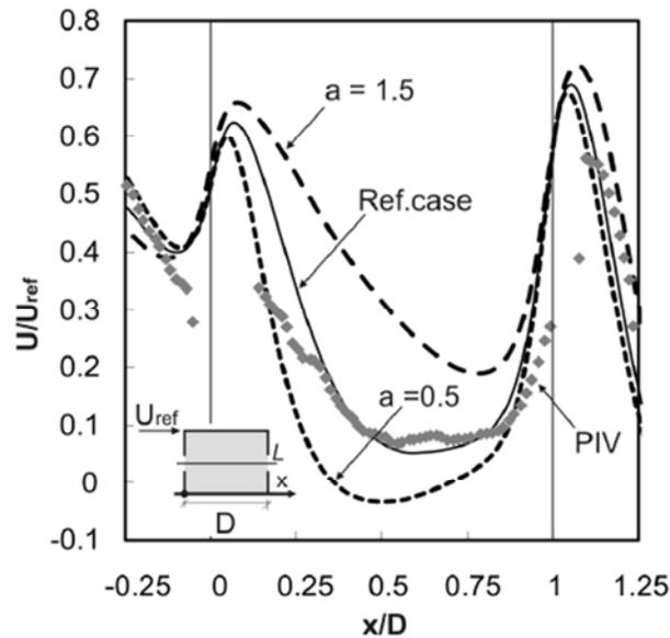
Figure 3.3.6.E: CFD simulation results for sensitivity analysis: impact of approach-flow turbulent kinetic energy profile parameter  $a$  on the streamwise wind speed ratio along the centerline ( $a = 1$  for the reference case).. (Ramponi and Blocken, 2012).
