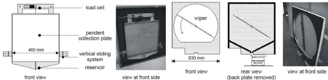
Figure 2.2.G (Left): Special wind-driven rain gauge designed to measure adhesion water. The collection plate and the reservoir are suspended from a load cell. Figure 2.2 G (Right): Special wind-driven rain gauge designed to measure adhesion water. The collection area is equipped with an automated wiper. (Blocken and Carmeliet ,2004)
