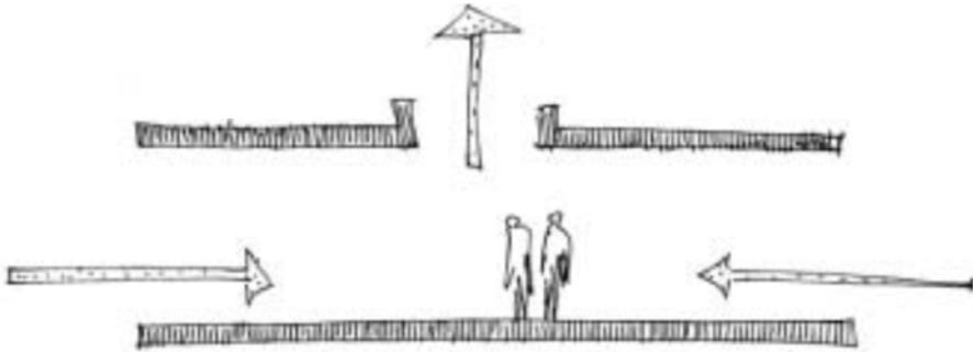
Figure 1.1G: Sketch of stack ventilation. As a rule of thumb, stack ventilation is effective across a width of 5 times the floor to ceiling height from the inlet to where the air is exhausted. (Kleiven, 2003)
