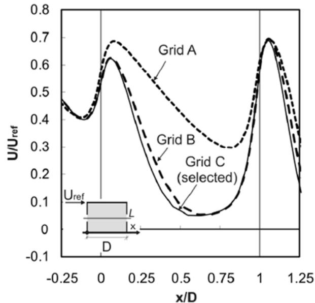
Figure 3.3.6.D: CFD simulation results for sensitivity analysis: impact of the grid resolution on the streamwise wind speed ratio along the centerline; Comparison of results from the three grids. (Ramponi and Blocken, 2012).
