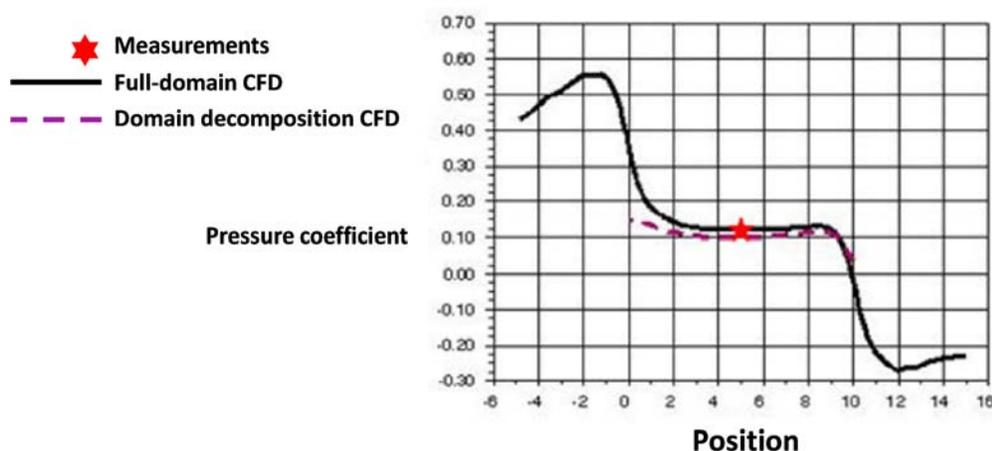
Figure 3.1.4.G: Static pressure coefficient,  $C_p$ , along line joining inlet and outlet openings for Case C
