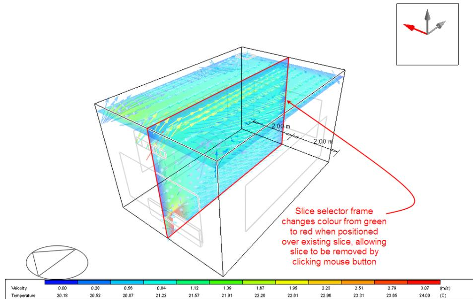
Figure 3.4.A: Setting up section plan for showing 2d data visualization in DesignBuilder CFD.
