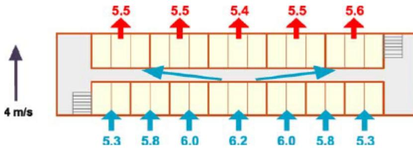
Fig. 2.2.M: ach results for a 4 m s<sub>-1</sub> normal wind in an open environment: fourth storey, basic opening regime. (Moeseke and etal, 2005)
