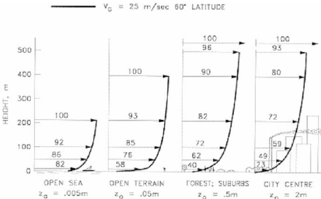
Figure 1.3.D: Different velocity profiles for four kinds of terrain typologies. (Crašto, 2007)
