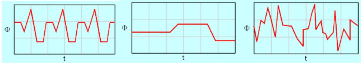
Figure 3.3.2.B: Time dependency of unsteady flow: (a) Periodic Flow, (b) Non-Periodic Flow and (c) Random Flow
