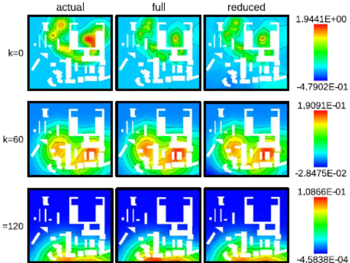
Figure 3.2.3D: Comparison between the actual contamination event (left column), inversion and prediction by the full model (center column), and inversion and prediction by the reduced model of dimension  $m = 800$  (right column) at the initial condition  $k = 0$  (top row), at the end of the observation period  $k = 60$  (middle row), and at the end of the prediction period  $k = 120$  (end row). All plots are cuts through  $z = 0.1$ , a representative slice. (Lieberman and etal, 2012)
