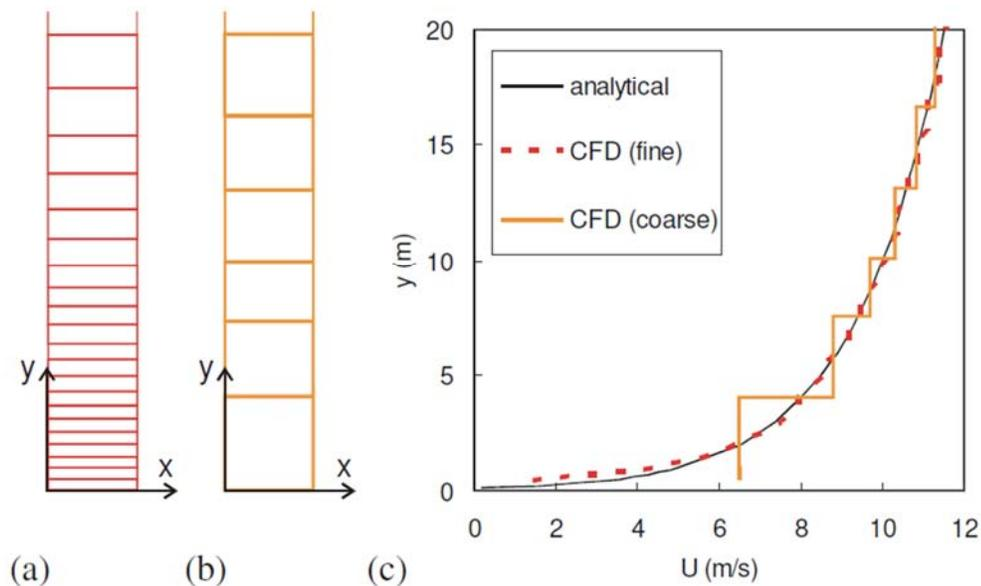
Figure 3.2.4.F (a-b) Fine and coarse vertical near-ground mesh distribution at the inlet plane. (c) Corresponding mean wind speed profile at the inlet of the domain: the analytical profile (imposed boundary condition) and the CFD profiles (one variable value per cell) for the fine and the coarse mesh distribution.
