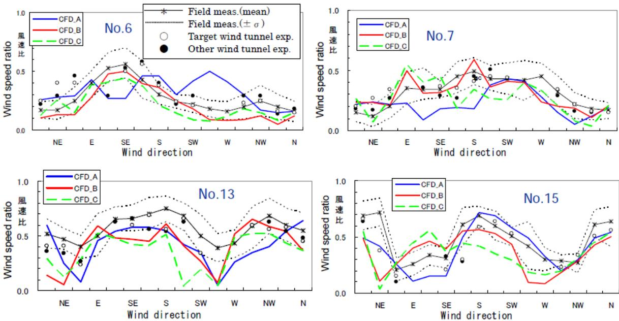
Figure 3.2.5.C: Comparison of wind speed ratio for 16 wind directions Tominaga et. al (2005).
