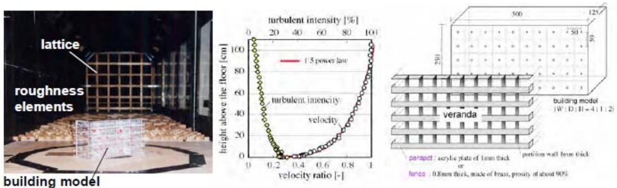
Figure 2.1A (Left): Wind tunnel set up
