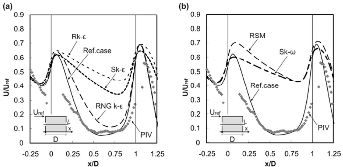
Figure 3.3.6.G: CFD simulation results for sensitivity analysis: impact of discretization scheme on the streamwise wind speed ratio along the centerline. For the reference case, a second-order discretization scheme is used. (Ramponi and Blocken, 2012).
