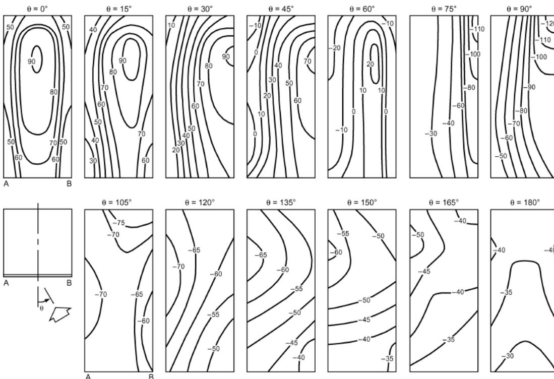
Figure 1.1.K: Local Pressure Coefficients ( $C_p \times 100$ ) for Tall Building with Varying Wind Direction (ASHRAE, Chapter 16, 2005)
