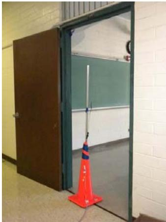
Deploying the anemometers at the test site; anemometers placement in doorway of room 313 (A4)
