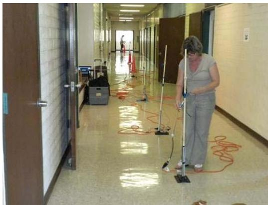
Deploying the anemometers at the test site; placement of all anemometers inside the hallway for measurements under test Scenario 1.
