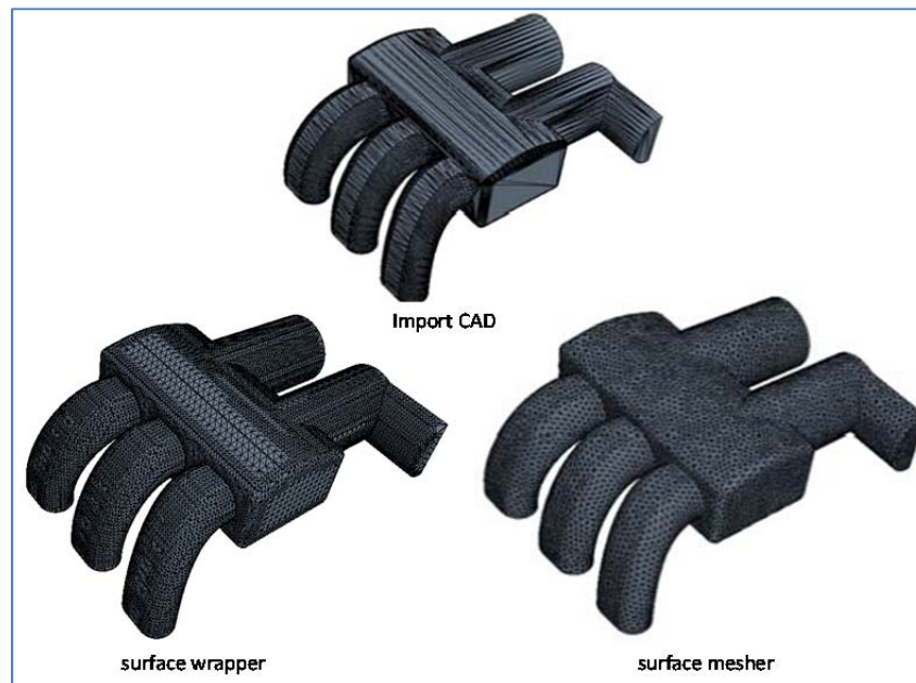
Figure 3.3.31: Comparison of surface wrapper and surface meshers from user guide version 8.02
