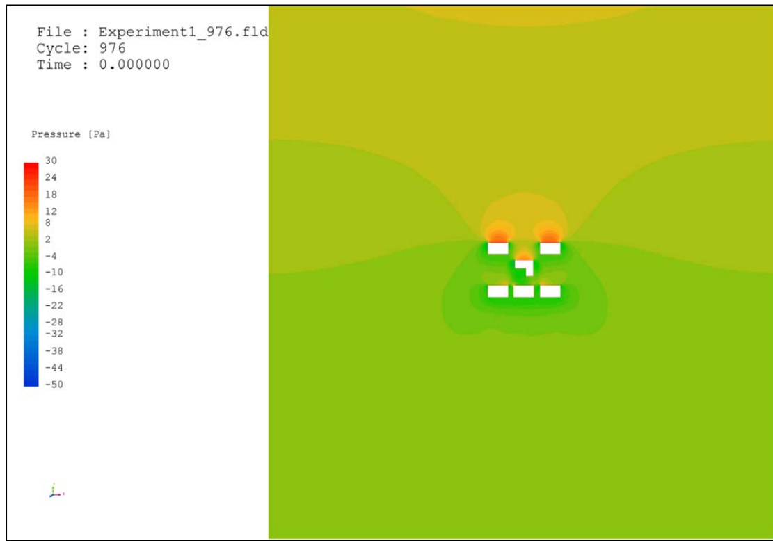
Figure 4.5.11: Pressure (Pa) contour map at the plane 10 feet above the ground (Cradle Stream).
