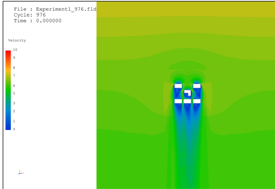
Figure 4.5.10: Velocity (m/s) contour map at the plane 10 feet above the ground (Cradle Stream).
