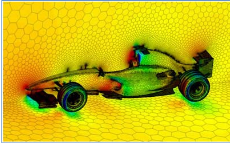
Figure 3.2.5B: Polyhedral meshing example from ANSYS Fluent
