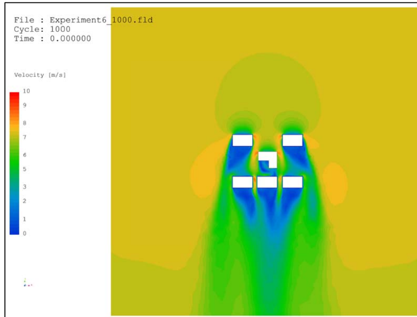
Figure 4.6.10: Velocity (m/s) contour map at the plane 10 feet above the ground (Cradle SC/Tetra).
