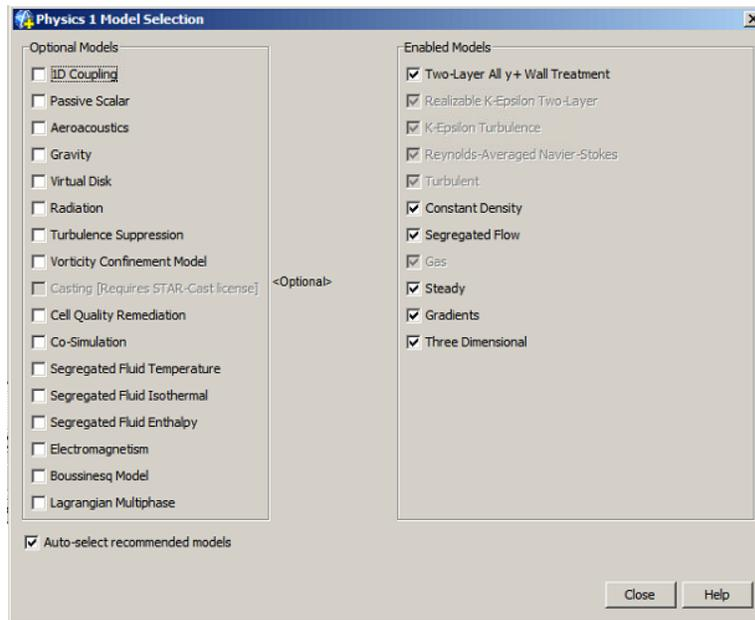
Figure 6.1.4: Data setting in STAR-CCM+ - Physics models selected for the simulation
