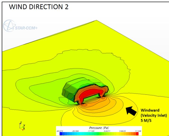
Figure 2.2.2: Initial CFD analysis results showing pressure distribution on the car surface and the ground (the perpendicular approach wind direction; Wind Direction 2)
