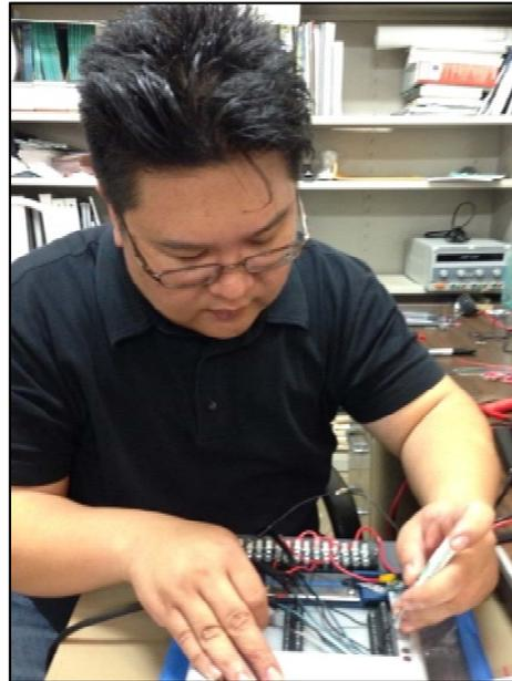
Figure 3.2.10. Integrating the sensors with the NI USB-6341 in office. Note the terminal block which distributes 24VDC electricity to the individual sensors
