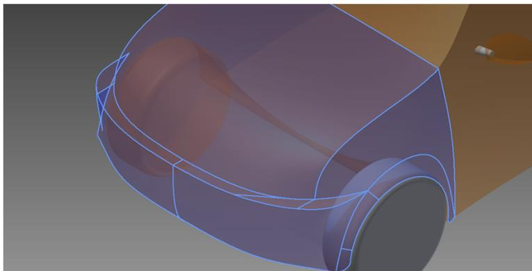
**Step 7.** Simple geometric objects can be easily modeled by using the Extrude command (ex. Wheels)
