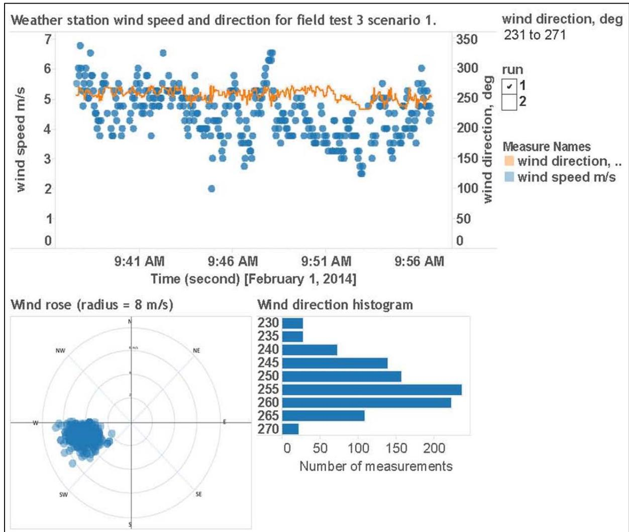
Figure 5.2.6.: Wind speeds and direction mapped for third field test (Scenario 1)
