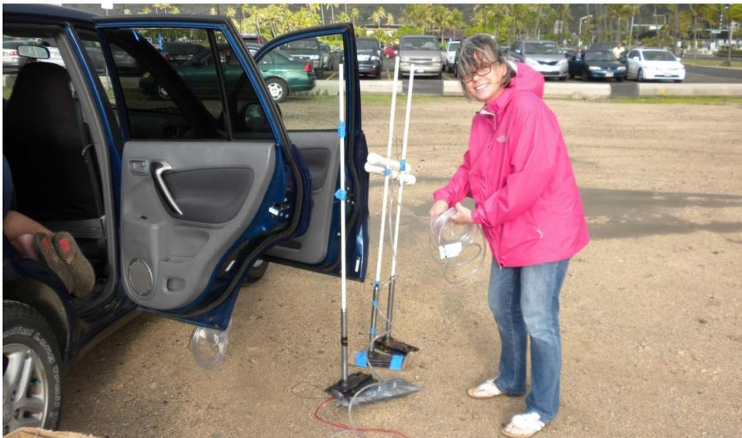
Figure 4.4.7.: Field Test Series #3: Attaching pressure tubing around the car, to measure pressure differentials
