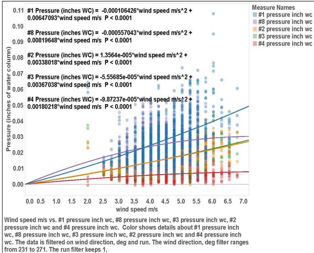
Figure 5.2.8: Pressures (in wc) compared to weather station wind speed readings (m/s)
