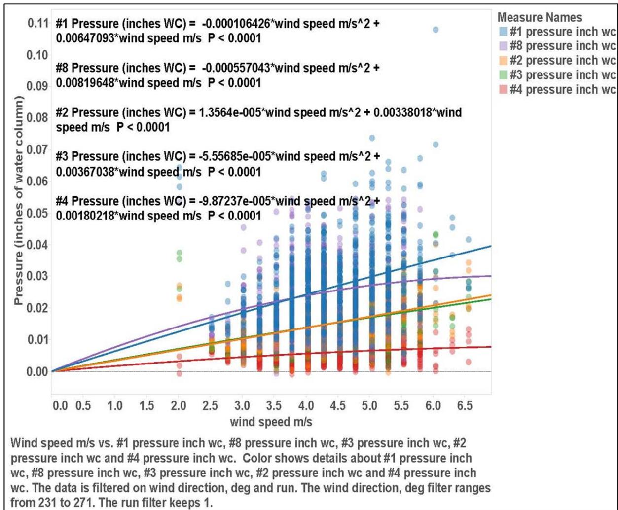
Figure 5.2.5.: Pressure readings (in wc) for sensors #1 2, 3, 4, and 8 for third field test (Scenario 1)
