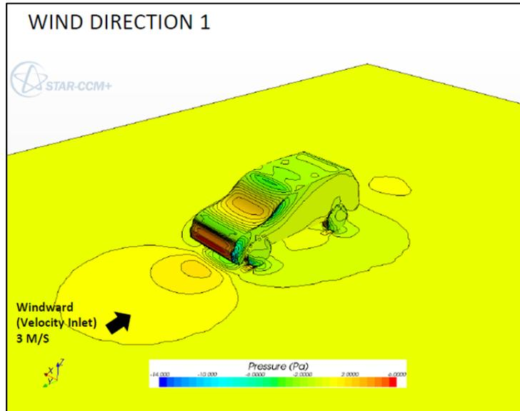
Figure 2.2.1: Initial CFD analysis results showing pressure distribution on the car surface and the ground (the parallel approach wind direction; Wind Direction 1).
