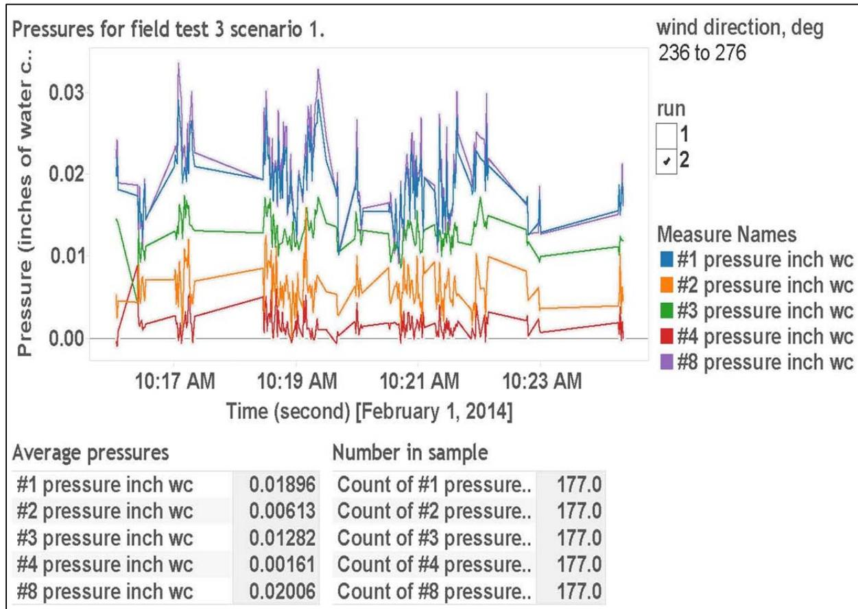
Figure 5.2.10.: Pressure readings (inch of wc) for third field test (Scenario 2)
