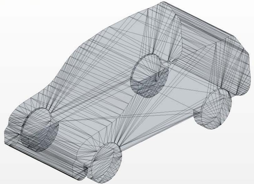
Figure 3: 3D CAD model in STAR-CCM+ in pre-meshing structure
