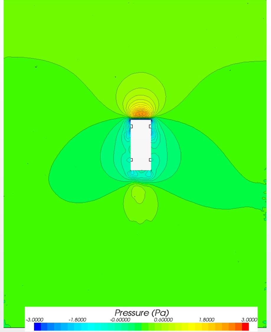
Figure 13: Example of velocity (m/s) and pressure (Pa) at 0.90 meter above ground
