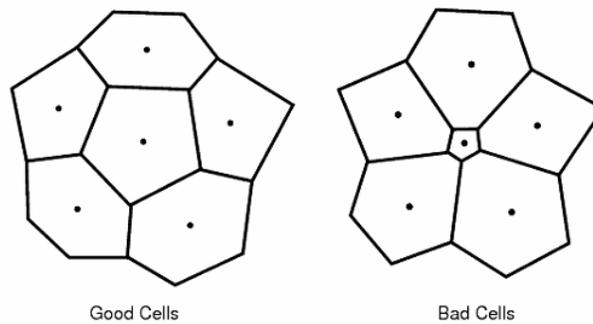
Figure 6.1.3.1: Example of good and bad cell based on volume change criterion (STAR-CCM+ Manual).
