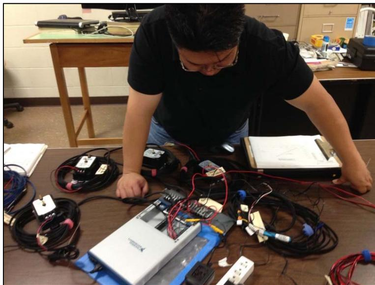
Figure 3.2.11. Overall picture of the integration of the various sensors fitted with 20' length wiring between the sensor and NI USB-6341 device
