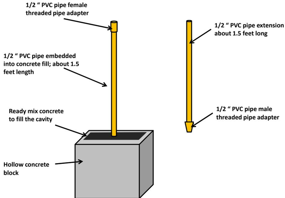
Figure 1: Simple instrument stands to be built for the shake-down test in the field
