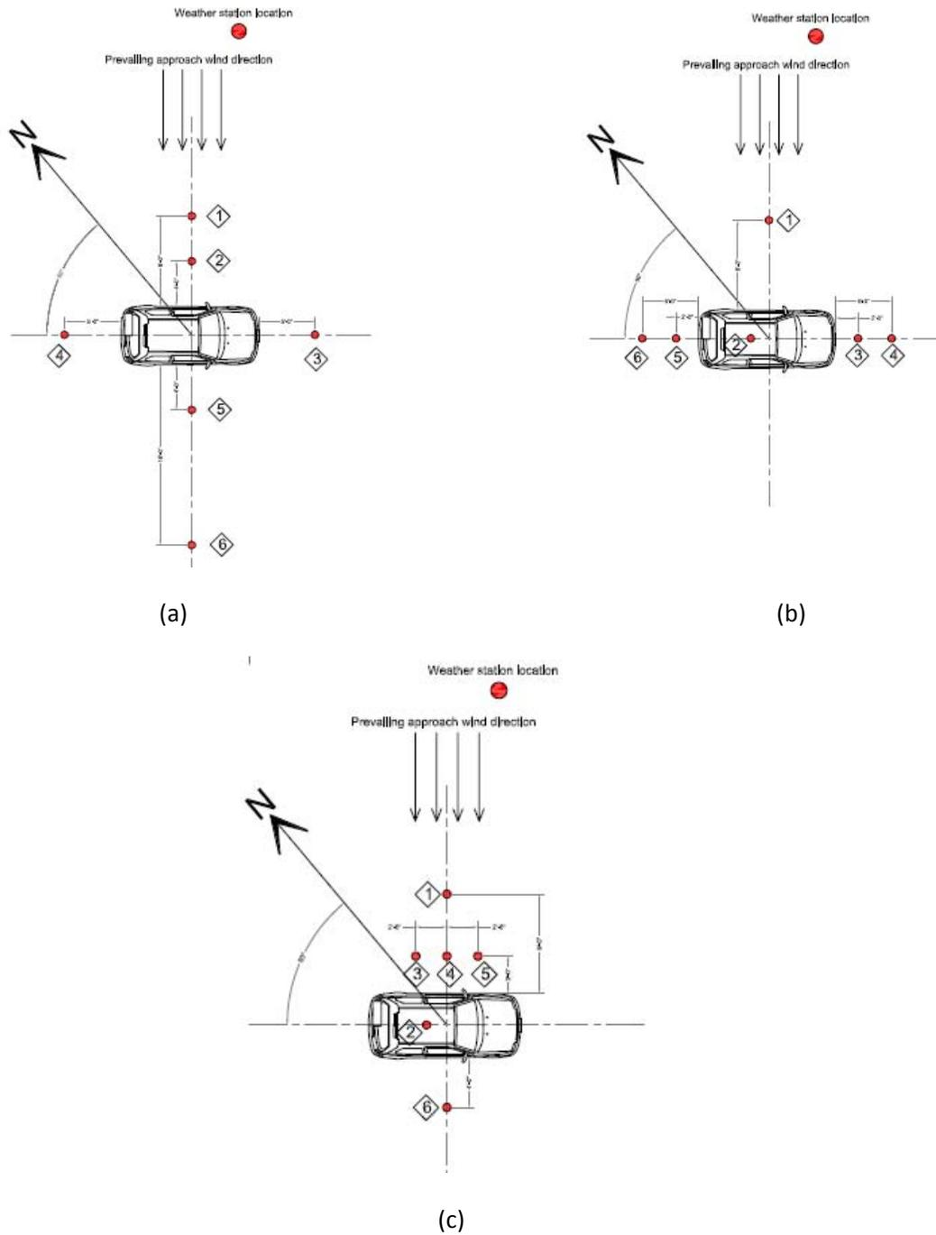
Figure 1. Scenarios of sensor layouts with wind perpendicular to the car for the first field test
