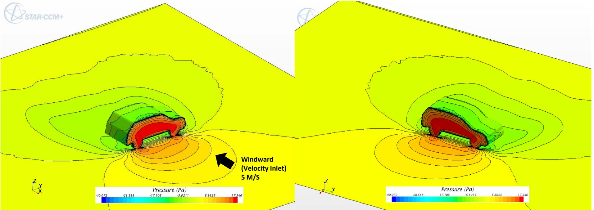
Figure 15: Example of pressure distribution on car surface in post simulation
