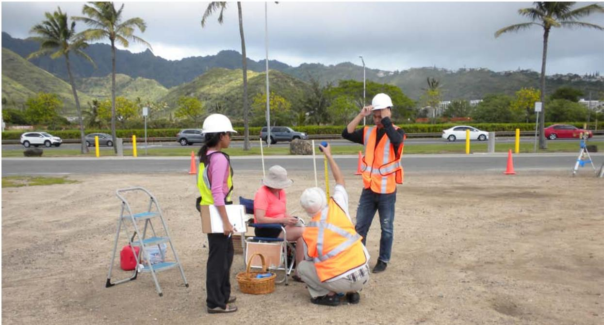
Figure 16. Measuring heights for setup of anemometers (F900 DegreeC sensors) for wind velocity profile
