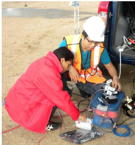
Figure 4.4.9.: Field Test Series #3: Setting up and ensuring pressure transducers are connected to measure and acquire data
