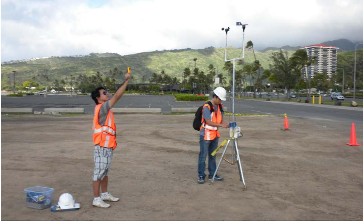
Figure 6. Setting up wind speed and direction sensors on the Hobo U30
