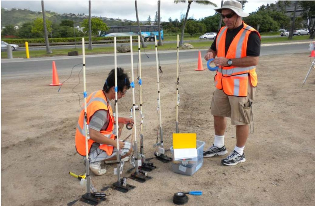
Figure 8. Anemometer (DegreeC F900) setup and labeling
