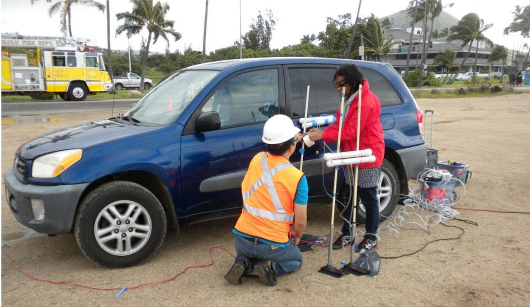
Figure 4.4.6.: Field Test Series #3: Setting up the pressure tubing to match heights and positions as indicated in the various CFD simulation setup scenario diagrams
