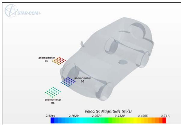
Small-grid probe to represent velocity data calculated in the CFD simulations
