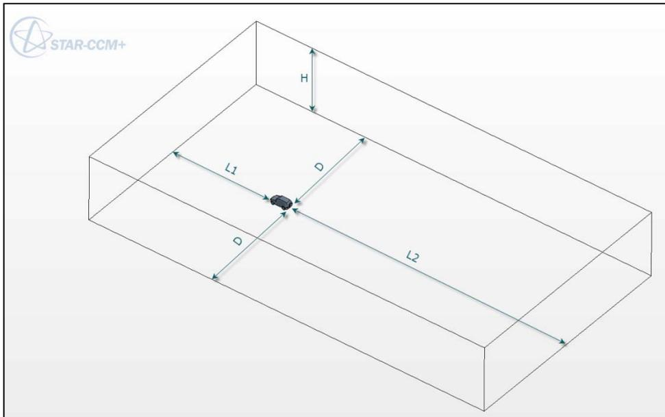
Figure 6.1.1.1a: The size of the computational domain for the car parallel to the prevailing wind test scenario
