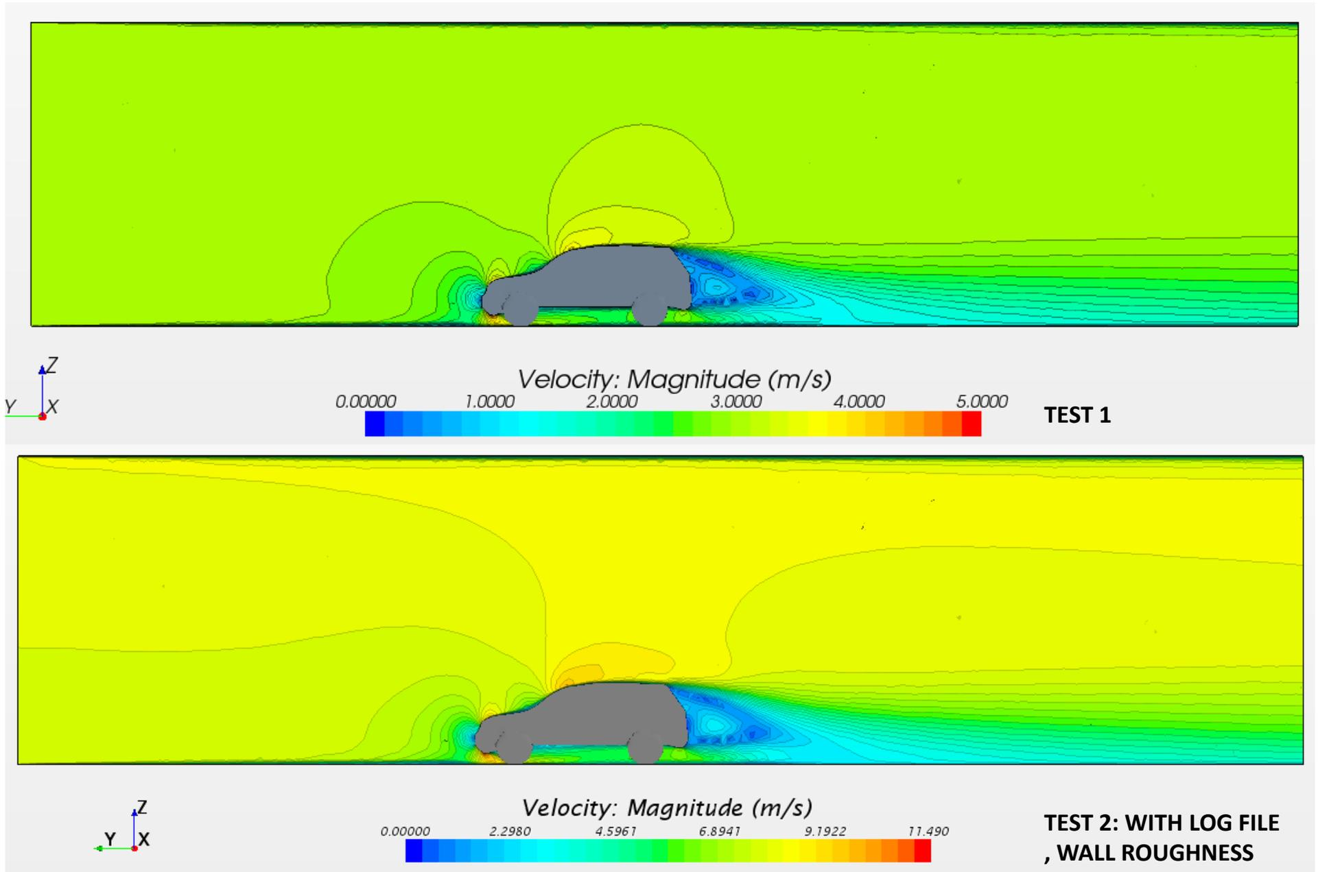
Figure 20: Compare simulation performance between Test 1 and Test 2
