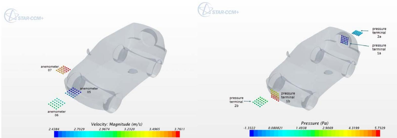
Figure 2: 1'x1' grid probes locations for extracted velocities and pressure data from CFD results for comparison (run 2: approach wind parallel to longitudinal axis of the car)
