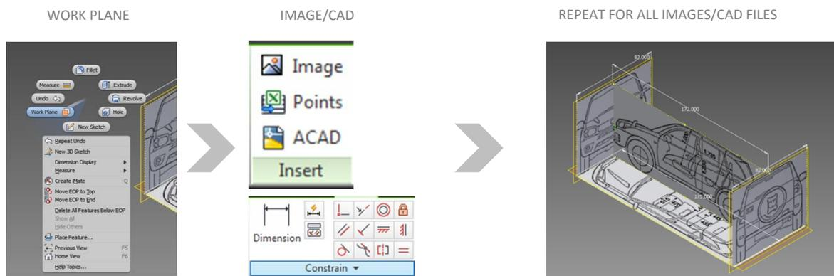
**Step 3.** Model the frame of the car using 2D sketch splines and 3D intersection curves.
