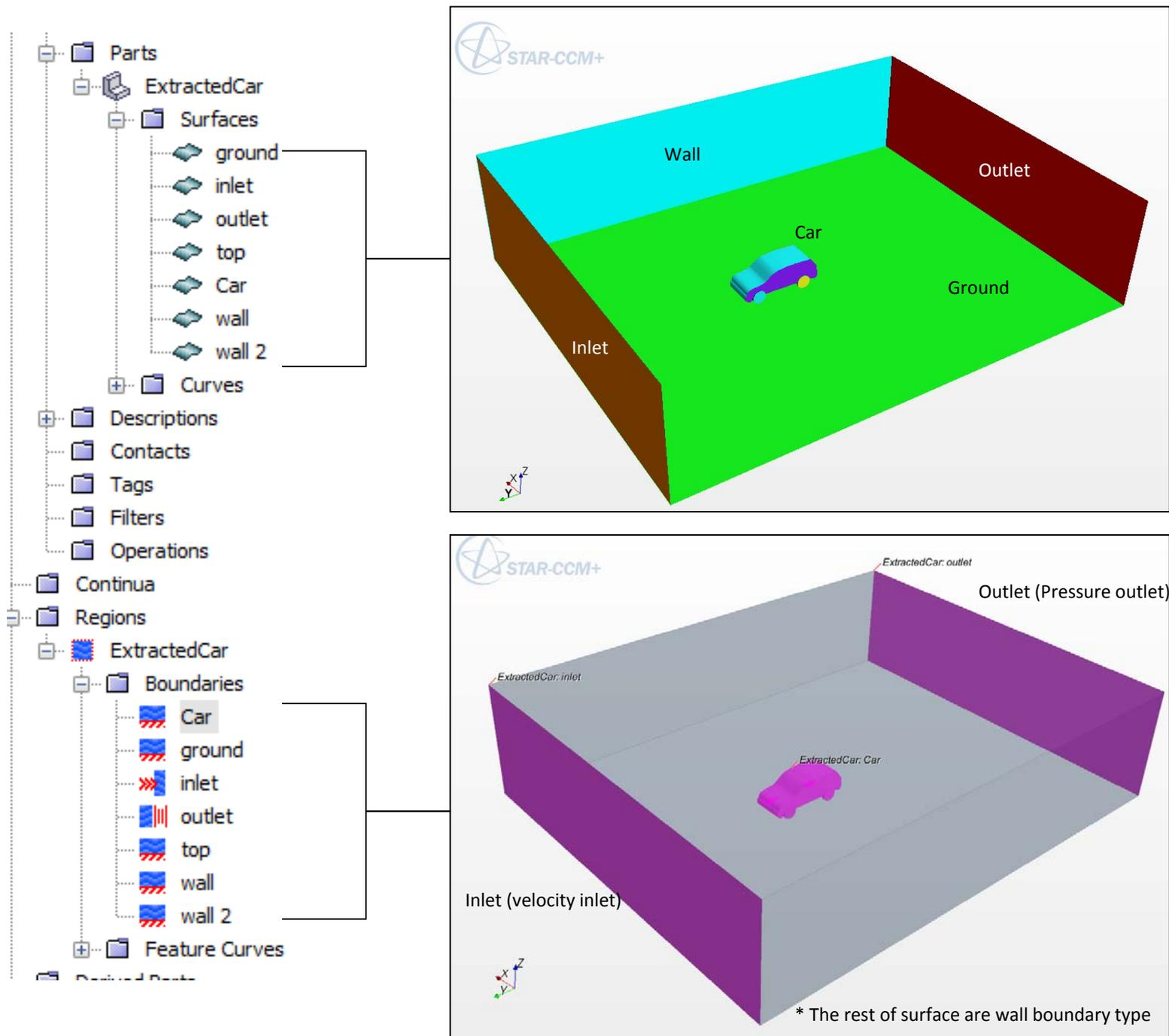
Figure 6: External CFD workflow for surface and regions set up
