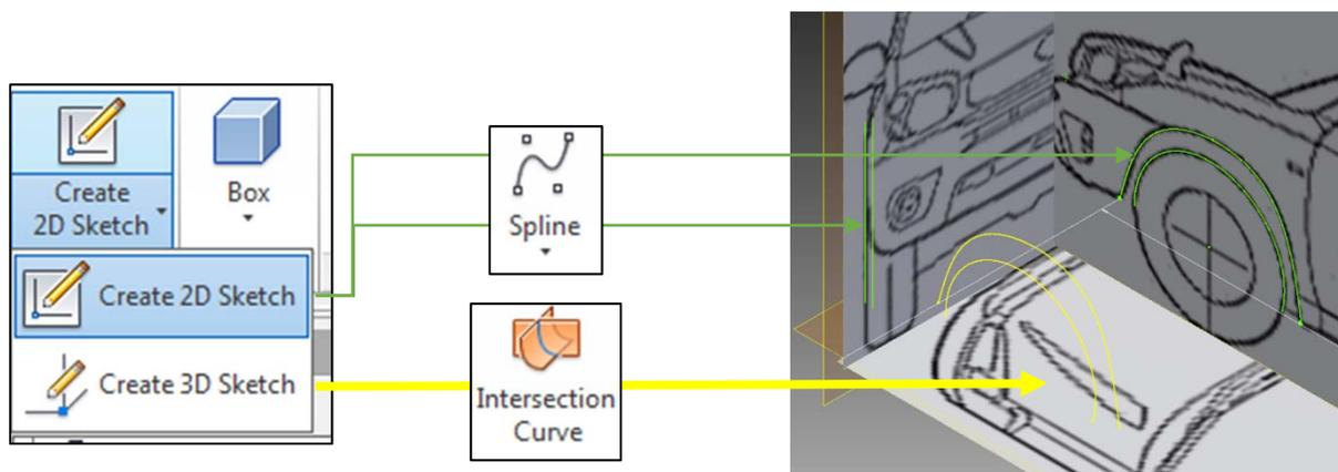
**Step 4.** Use project geometry while creating splines to insure all surfaces will intersect and not leave openings.
