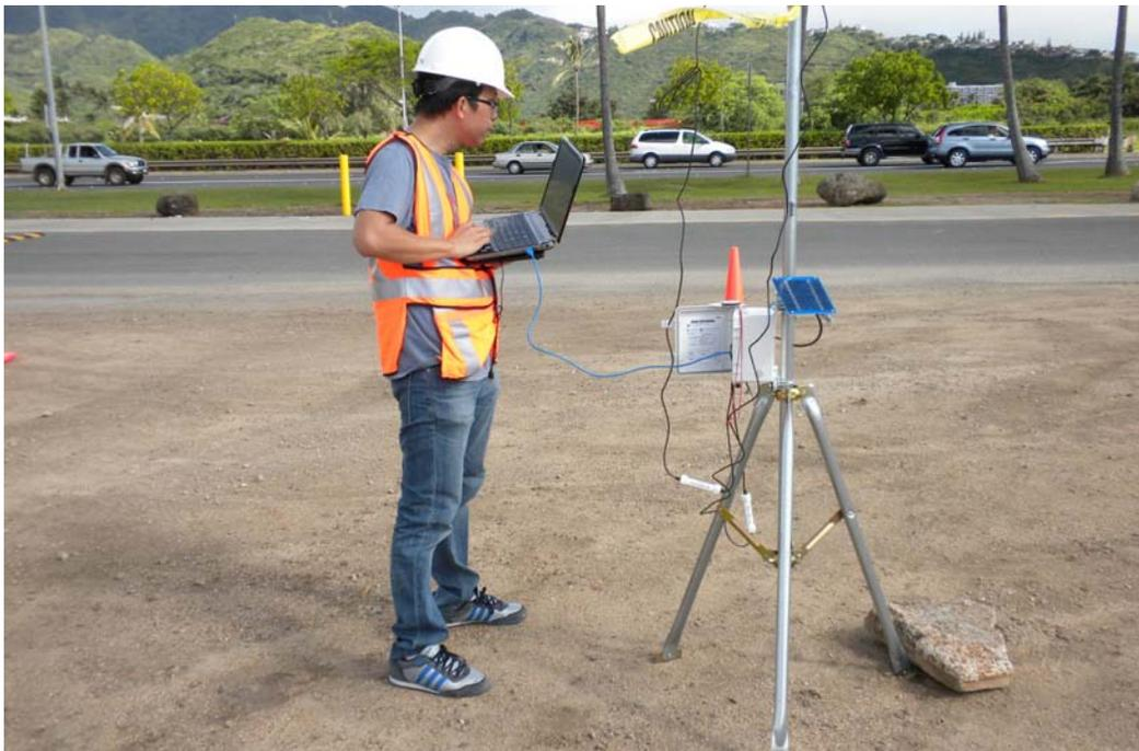
Figure 9. Setting up and downloading data acquisition (1-second intervals) on the Hobo U30 logger
