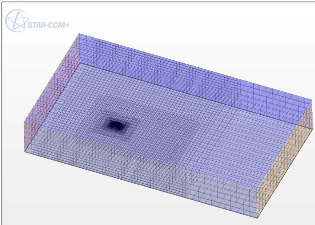
Figure 6.1.2.3: Meshing of computational domain and the car.
