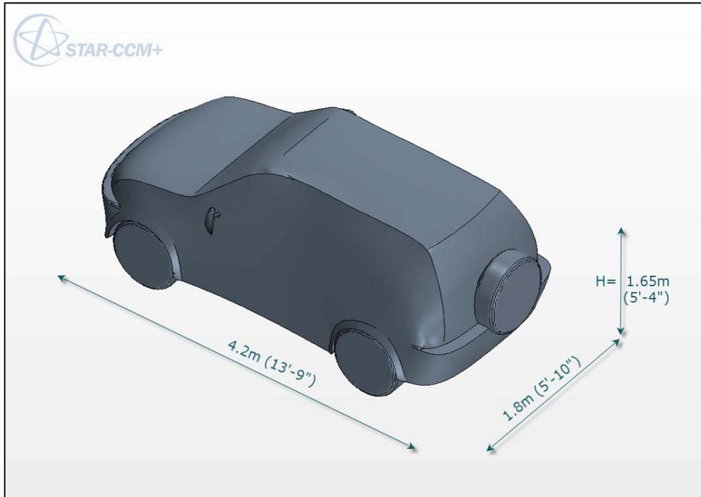
Figure 6.1.1.2: The dimension of the test structure (RAV-SUV) car which was used for the shakedown tests
