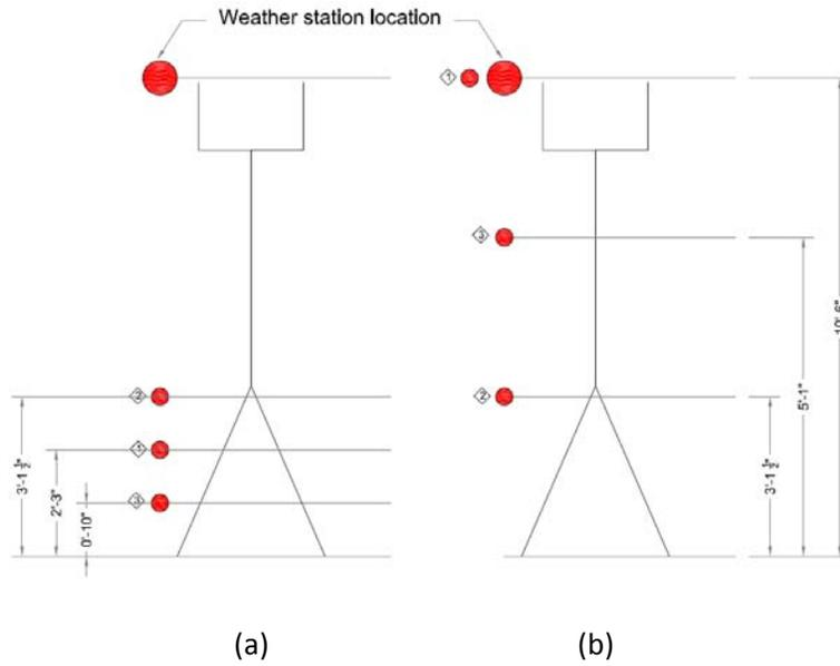
Figure 15. Sensor setup for measuring the approach wind velocity profile for the second field test (See Figs. 16-20 for corresponding site photos and layout)
