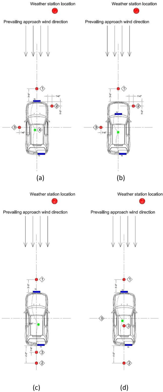
Figure 13. Scenarios of sensor layouts with wind parallel to the car for the second field test (See Fig. 14 for corresponding site photos, Figs. 15-20 for instrumentation and field setup)
