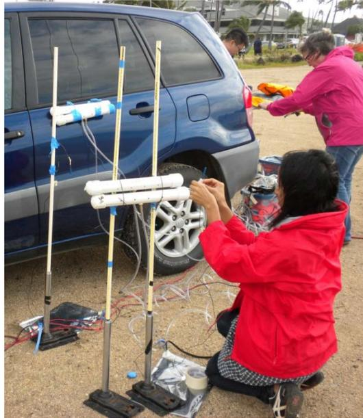
Figure 4.4.8.: Field Test Series #3: Checking measurements and angles of the anemometers
