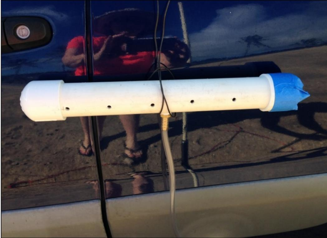
Figure 3.2.4.: Pressure tubing terminal unit used to provide undisturbed and averaged pressure conditions for the Setra and Halstrup-Walcher differential pressure transducers.
