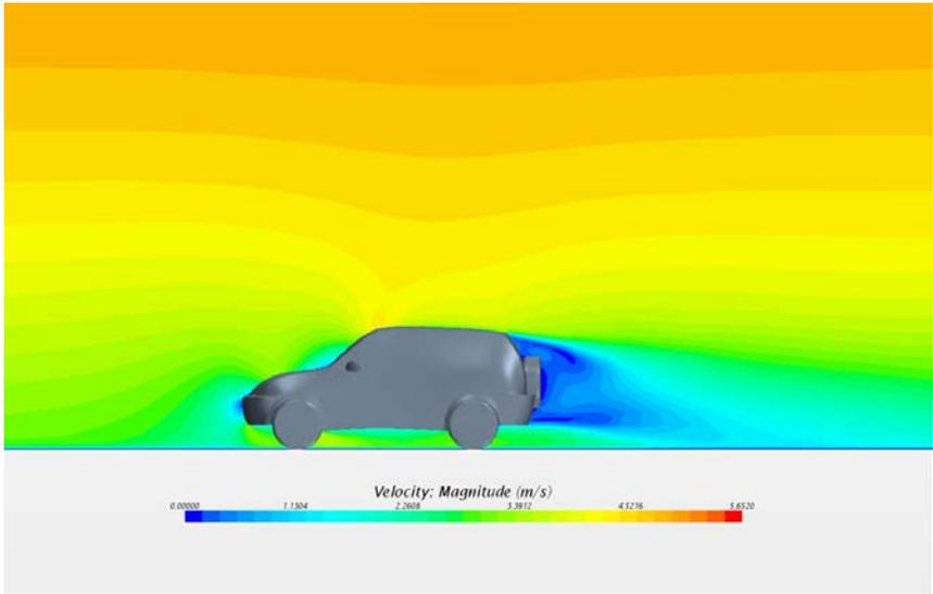
Figure 5: Velocity map on 3 feet elevation plane and at cross section (run 2: approach wind parallel to longitudinal axis of the car)
