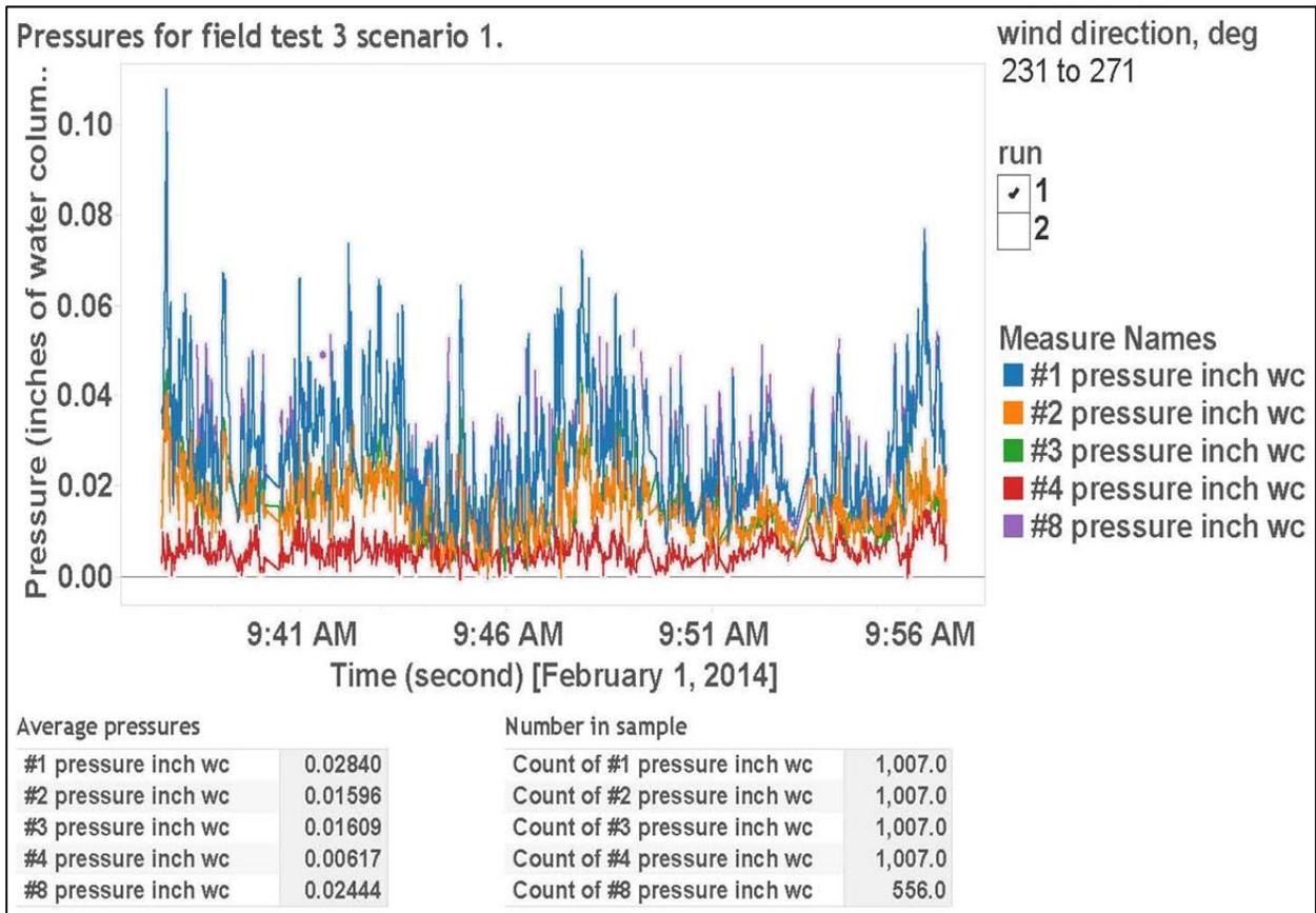
Figure 5.2.7: Pressures (in wc) mapped for third field test (Scenario 1)
