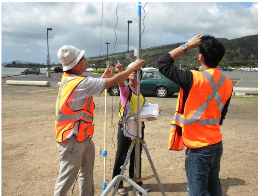
Figure 20. Setup of (F900) anemometers and (U30) weather station to match scenario in Fig. 15 (b)
