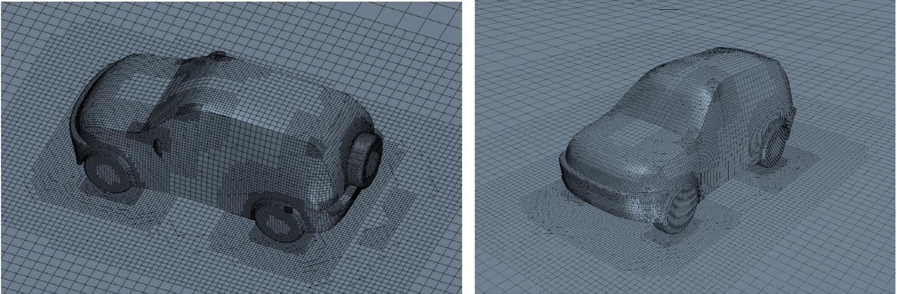
Figure 2: Detailed view of the car's meshing for two scenarios.
