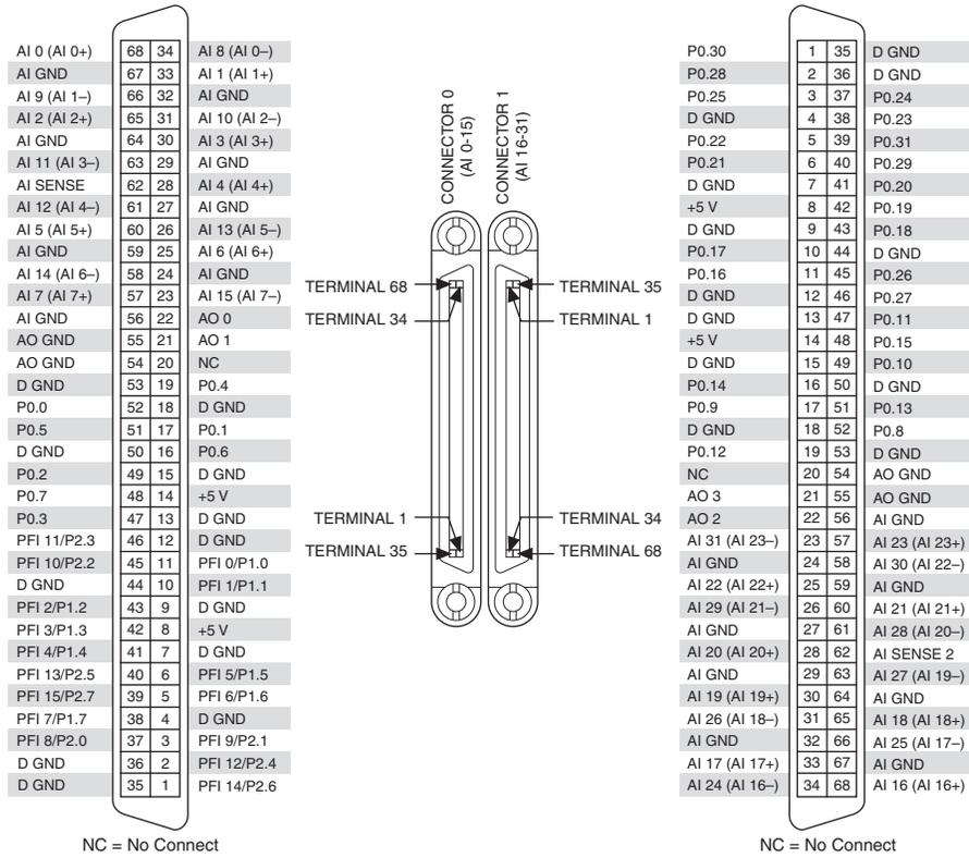
**Figure 5. NI USB-6343 Screw Terminal Pinout**
