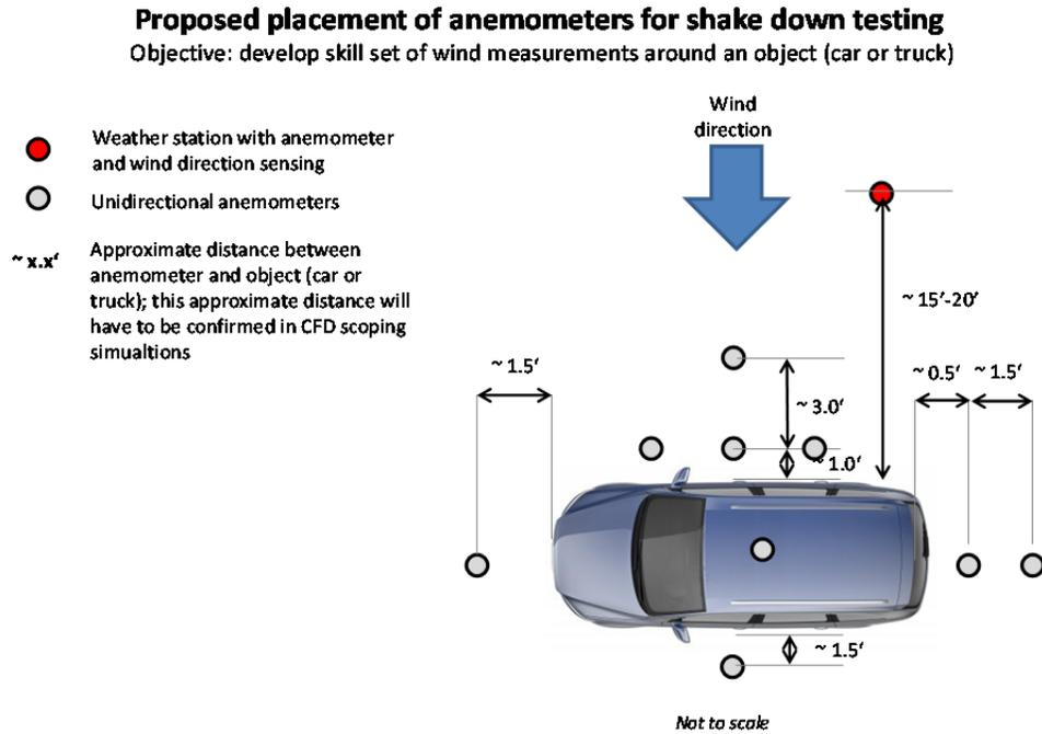
Figure 7: proposed placement of anemometers around the test specimen for shake-down testing
