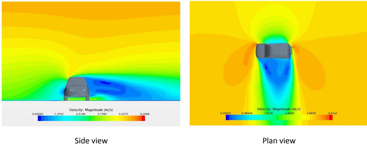
Figure 6.2.1.1: **Scenario 1:** Velocity map at cross section and Pressure map at 3 feet height elevation plane (Scenario 1: approach wind perpendicular to the longitudinal axis of the car)
