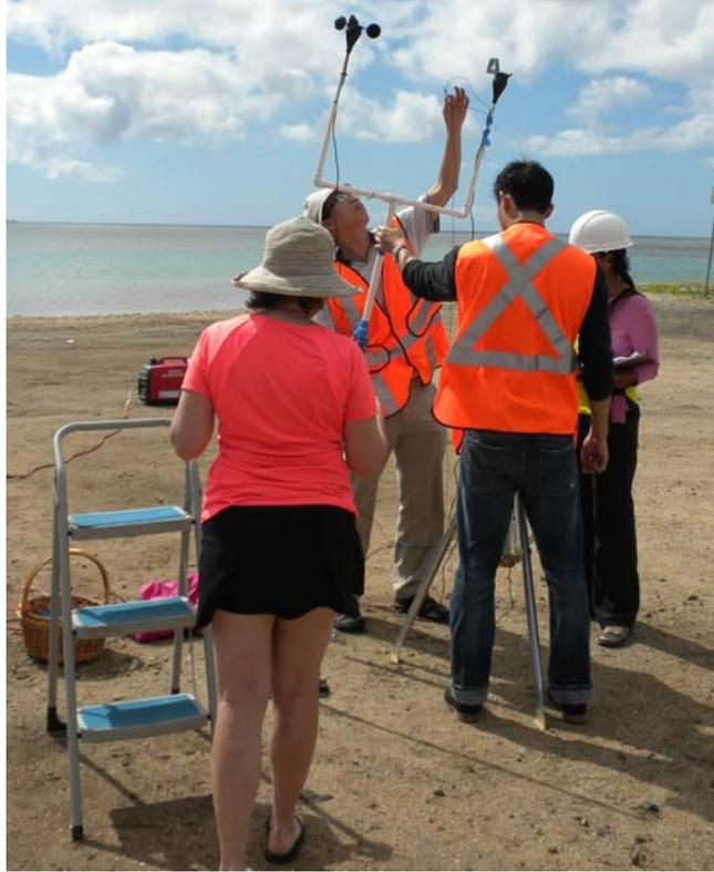
Figure 19. Setup of (F900) anemometers and (U30) weather station to match scenario in Fig. 15 (b)
