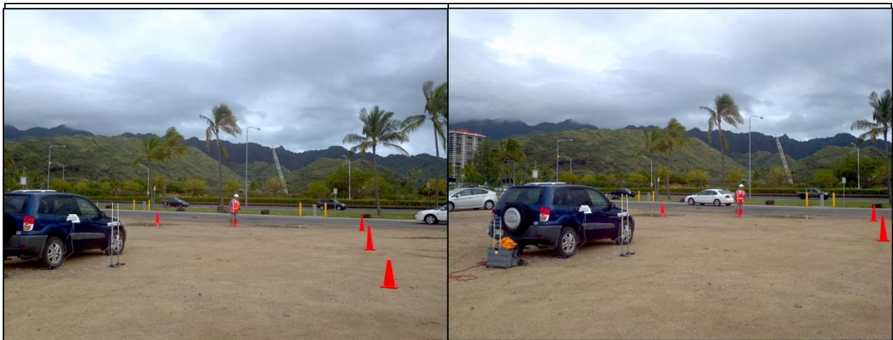
Figure 4.4.2: Sensor layout for the third field test: (a) Scenario 1 (wind perpendicular to the car)
