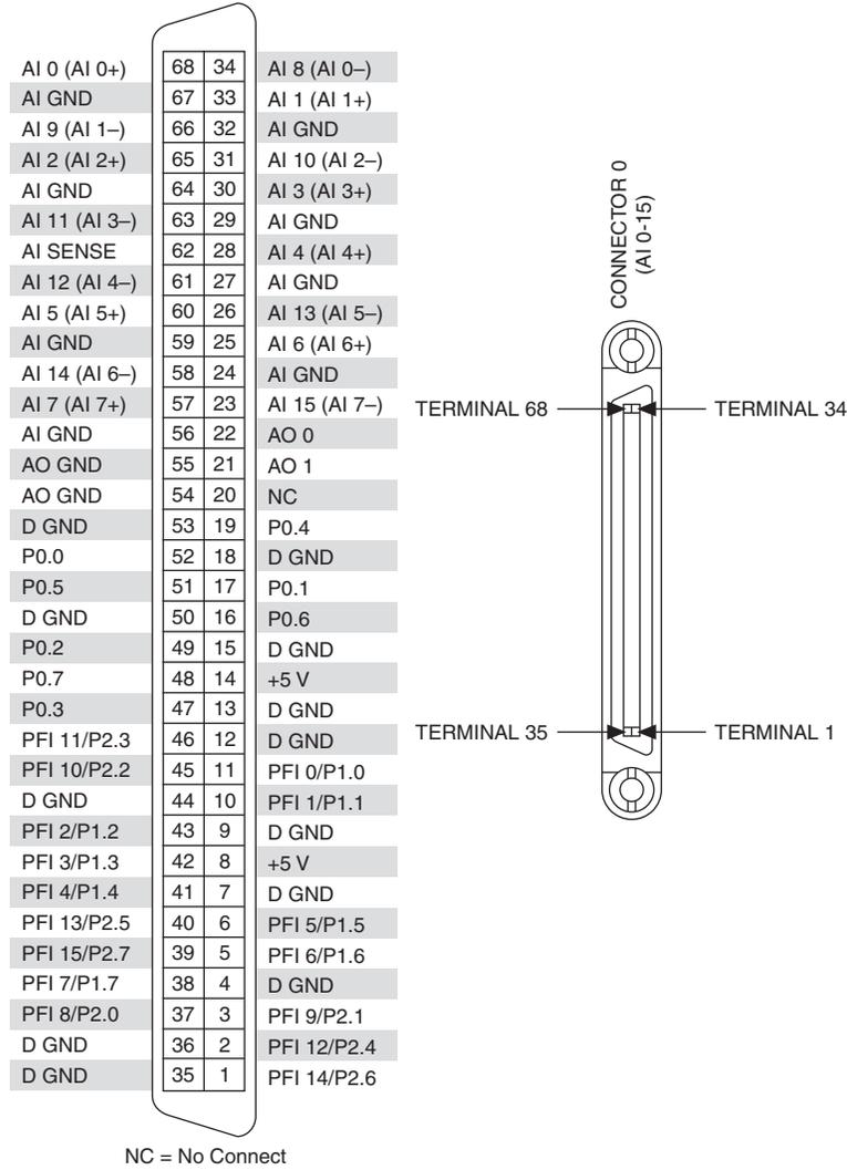
**Figure 2. NI USB-6341 Screw Terminal Pinout**
