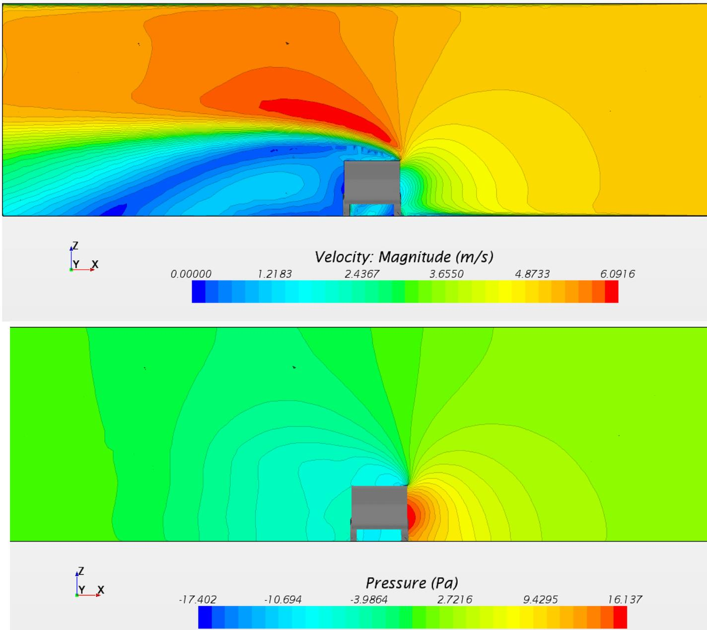
Figure 17: Example of velocity (m/s) and pressure (Pa) at cross section
