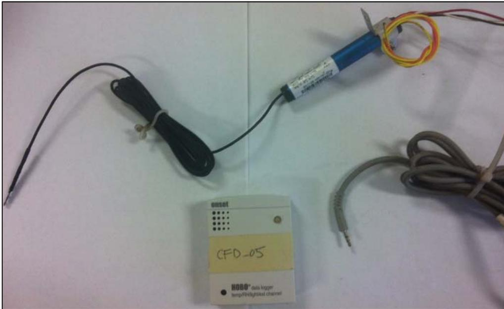
Figure 3.2.7.: The DegreeC F900 Anemometer. (shown with the cylindrical signal conditioning unit and the U12 data logger)
