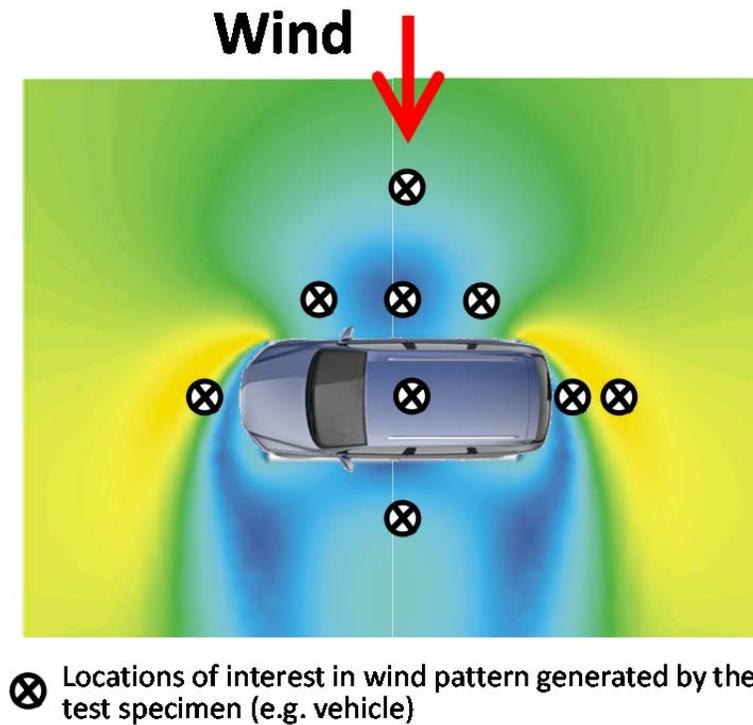
Figure 6: Anticipated locations of interest to obtain velocity data (Note: velocity pattern indicated is a generic pattern and does not reflect the CFD analysis for the test specimen)
