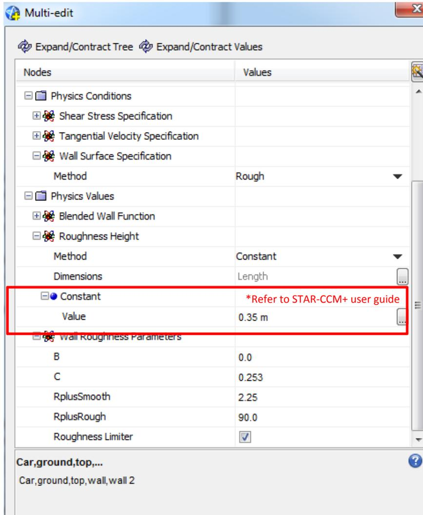
Figure 17: Wall roughness set up
