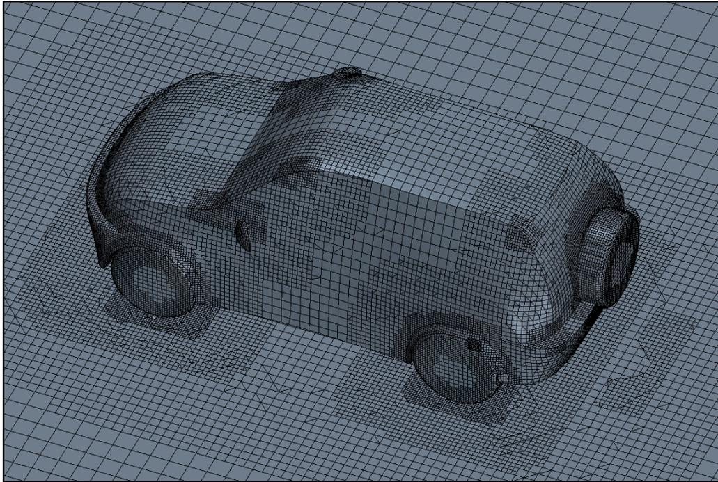
Figure 6.1.2.4: Detailed surface meshing of the car.
