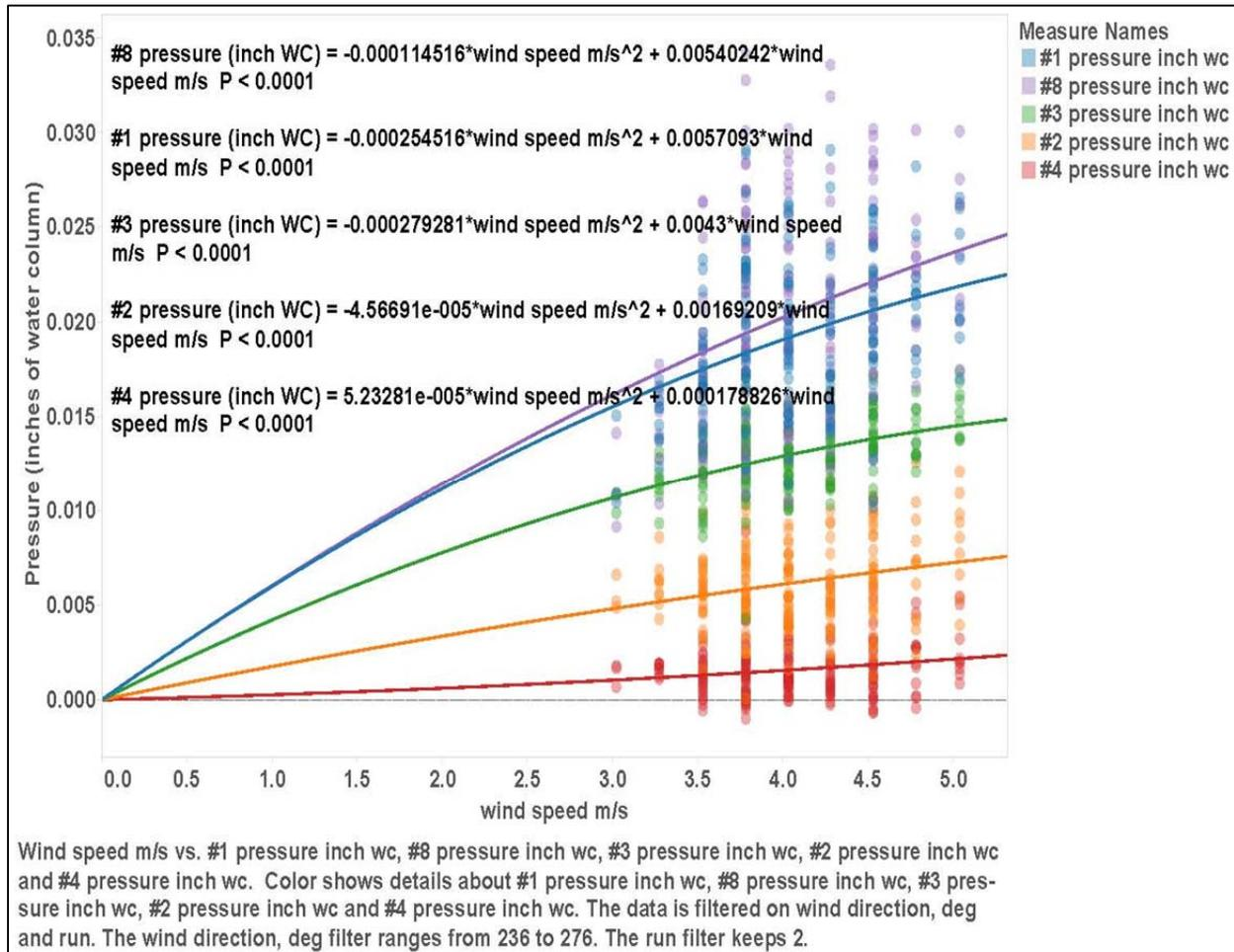
Figure 5.2.16. Pressure readings (in wc) for sensors #1 2, 3, 4, and 8
