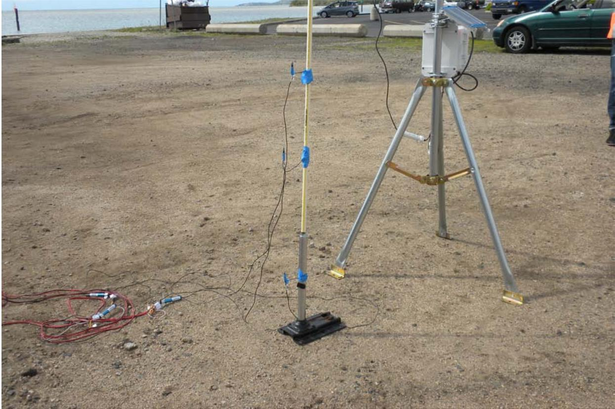
Figure 18. Setup of F900 anemometers and weather station to match scenario layout in Fig. 15 (a)
