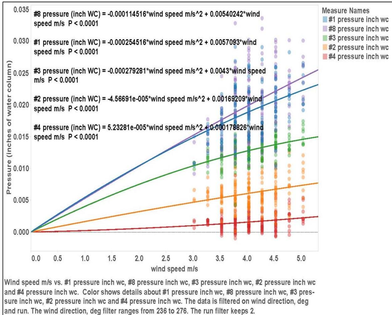
Figure 5.2.13: Pressure readings (in wc) for sensors #1 2, 3, 4, and 8
