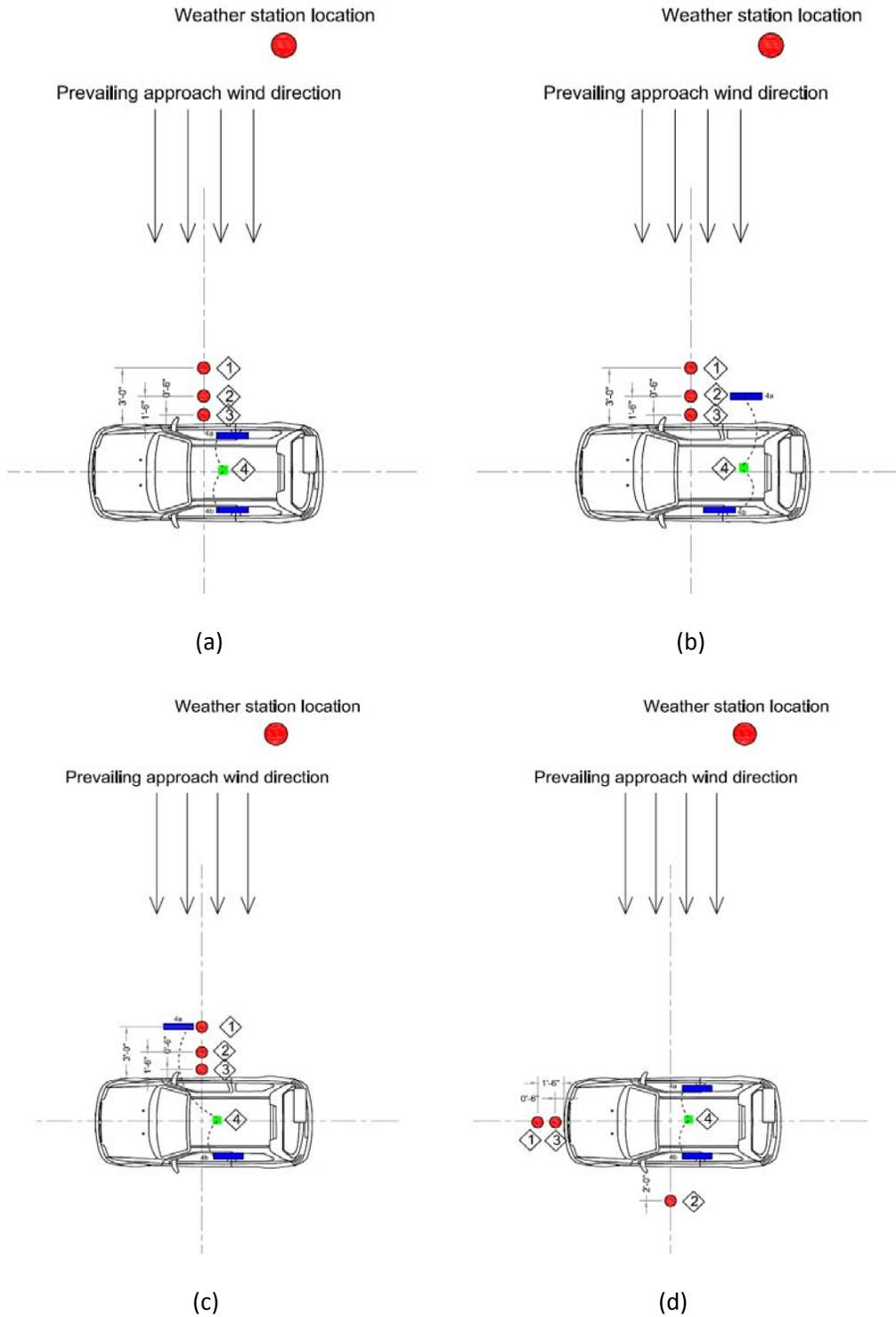
Figure 11. Scenarios of sensor layouts with wind perpendicular to the car for the second field test
