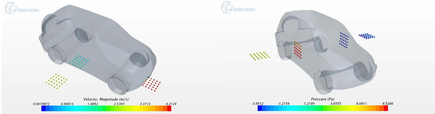
Figure 1: 1'x1' grid probes locations for extracted velocities and pressure data from CFD results for comparison (run 1: approach wind perpendicular to longitudinal axis of the car)
