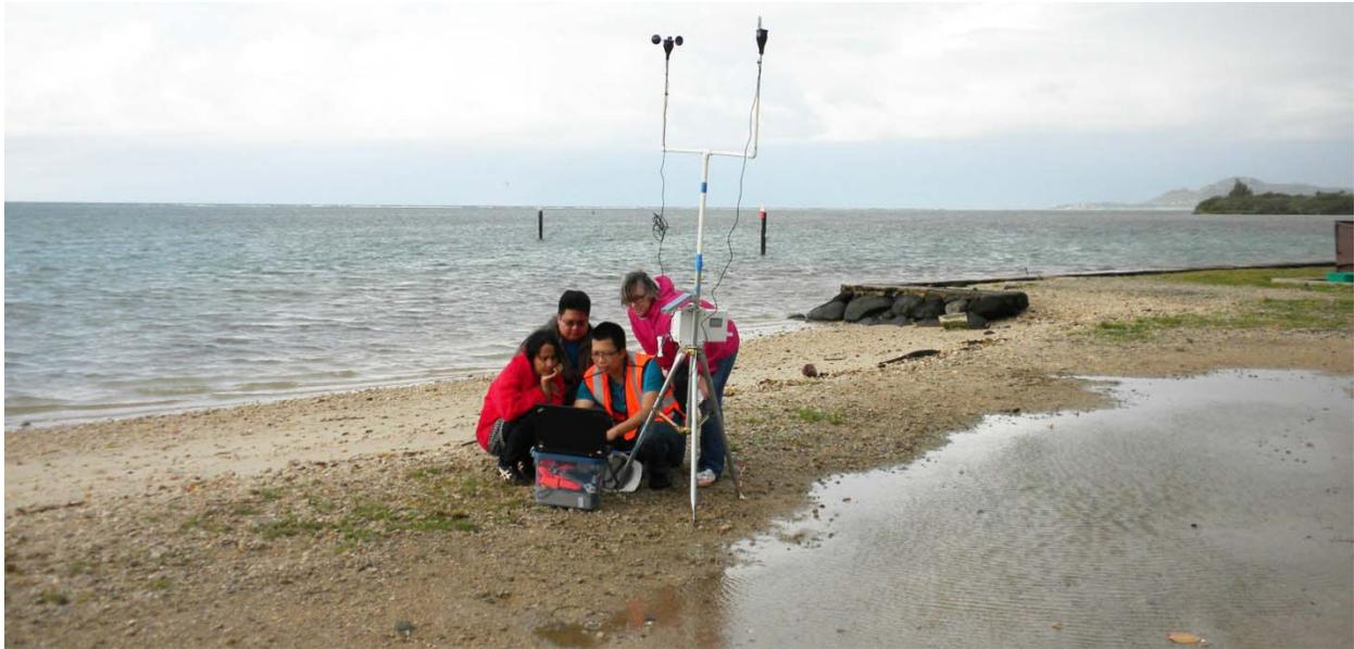
Figure 4.4.5.: Field Test Series #3: Setting up the Hobo U30 weather station (wind speed and direction sensors)
