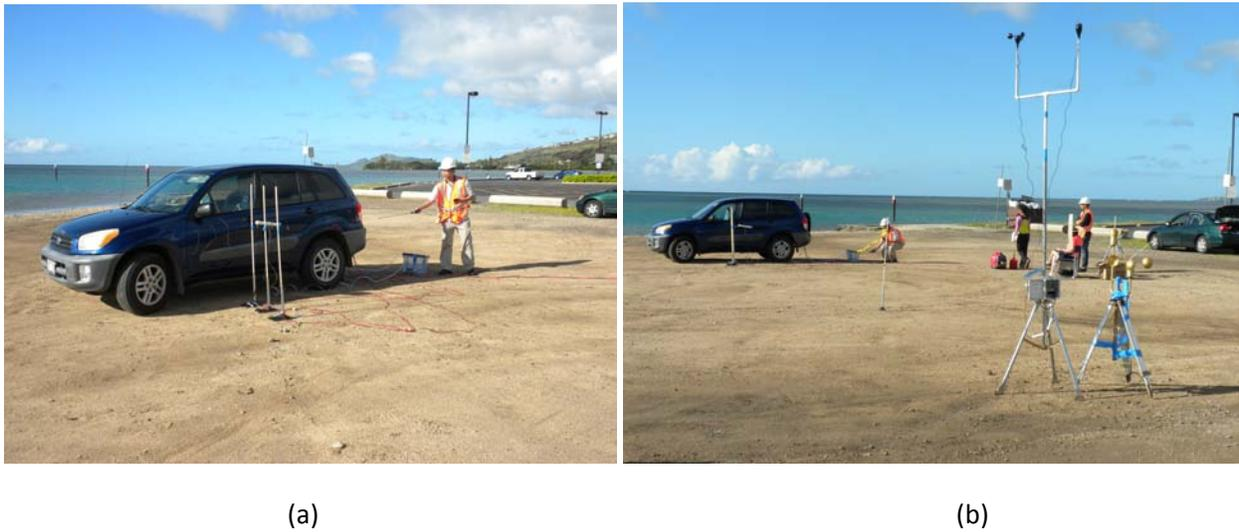
Figure 12. Site photos of sensor setup (wind perpendicular to the car) for the second field test
