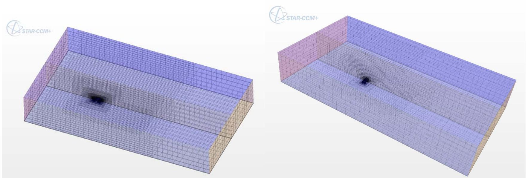
Figure 1: Meshing of the computational domain for two scenarios
