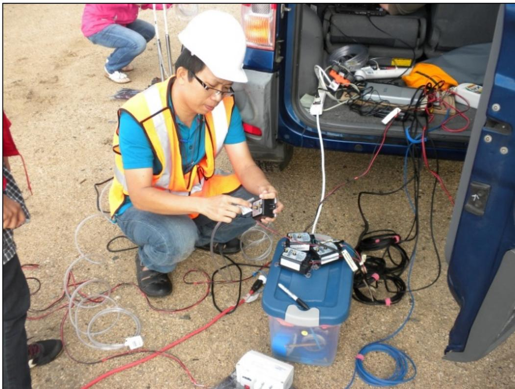
Figure 3.2.3.: Dr. Tuan Tran sorting the Setra and Halstrup-Walcher differential pressure transducers with the signal multiplexer (NI USB-6341) device (shown in the rear of the car).
