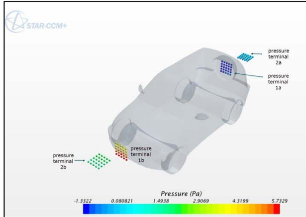
Small-grid probe to represent pressure data calculated in the CFD simulations
