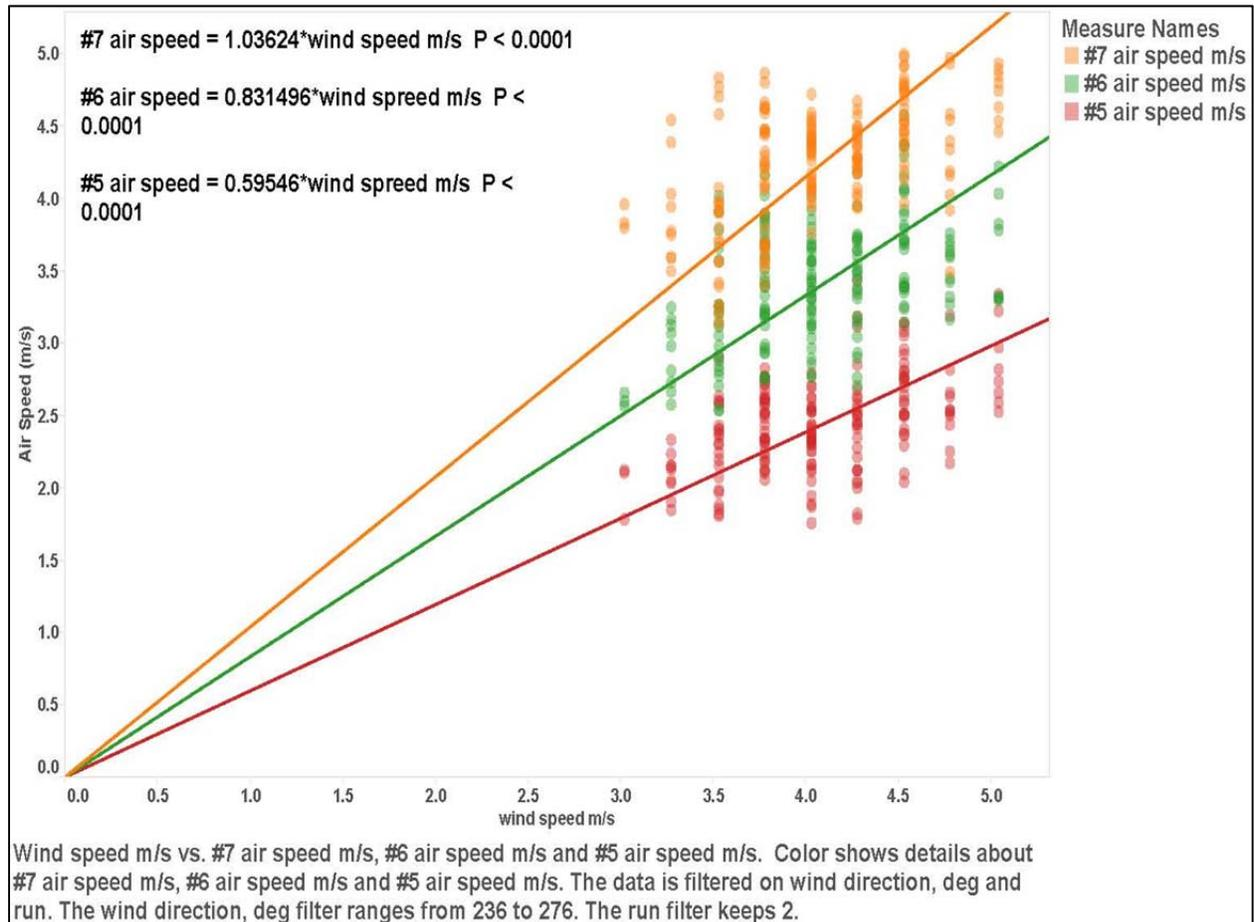
Figure 5.2.12. Wind speeds (m/s) for sensors #5, 6, and 7
