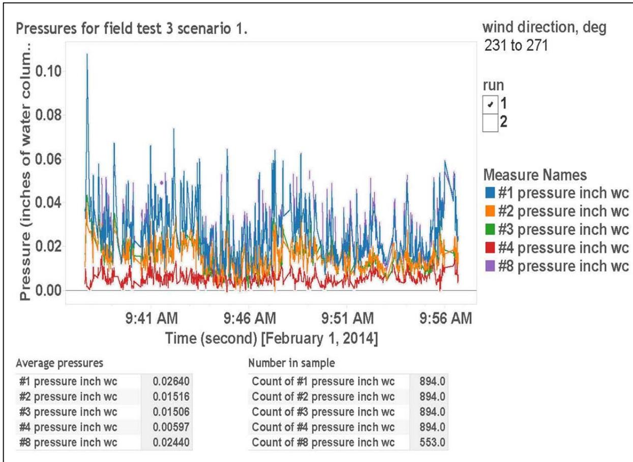
Figure 5.2.2. Pressures (in inch wc) for third field test (Scenario 1)
