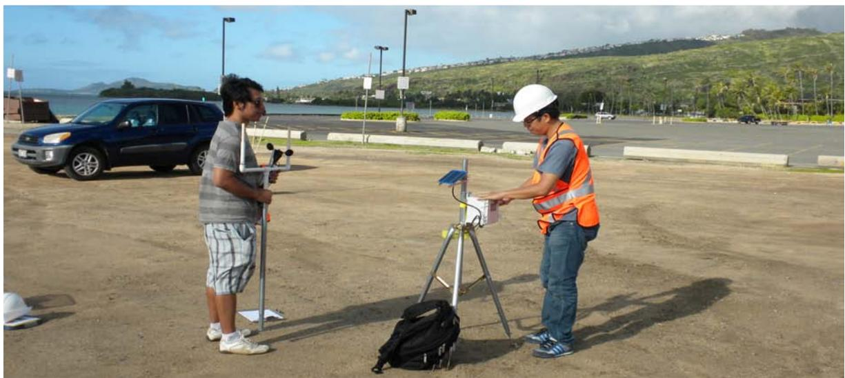
Figure 5. Calibrating and setting up the weather station (Hobo U30)
