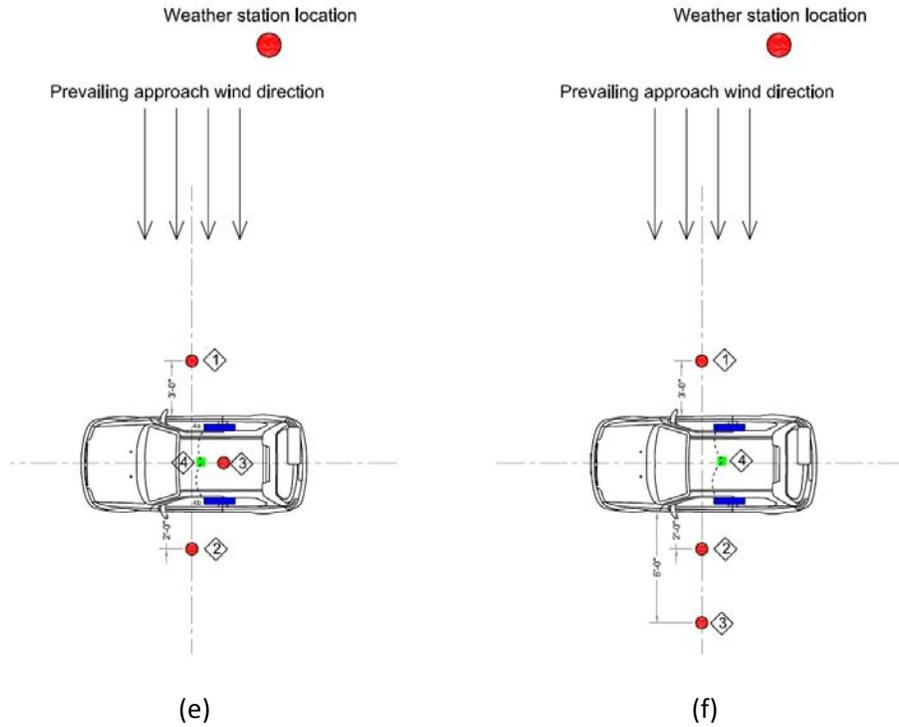
Figure 11(contd). Scenarios of sensor layouts with wind perpendicular to the car for the second field test
