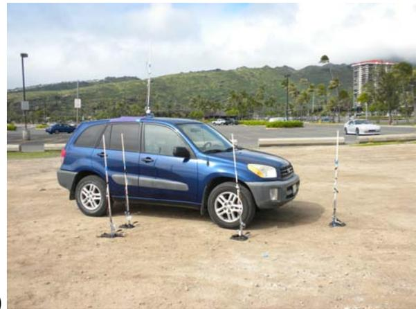
Figure 4. Scenario photos of sensor layouts with wind parallel to the car for the first field test (See Fig. 3 for corresponding scenario diagrams, Figs. 5-10 for instrumentation and field setup)
