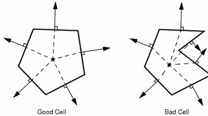
Figure 6.1.3.1 Example of good and bad cell based on cell validity criterion (STAR-CCM+ Manual).
