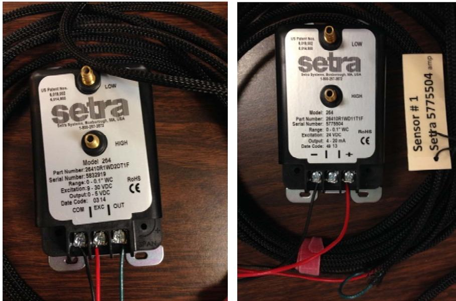
Figure 3.2.1.: Setra Differential Pressure Transducer Model 264
