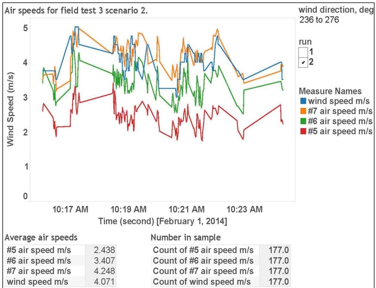
Figure 5.2.9.: Air speeds (m/s) for third field test (Scenario 2)
