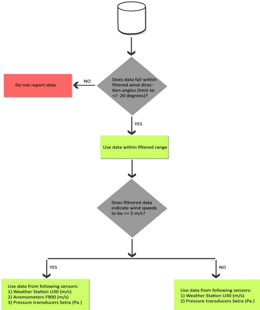
Figure 5.1.1. Flowchart indicating process applied to data through various filtering techniques
