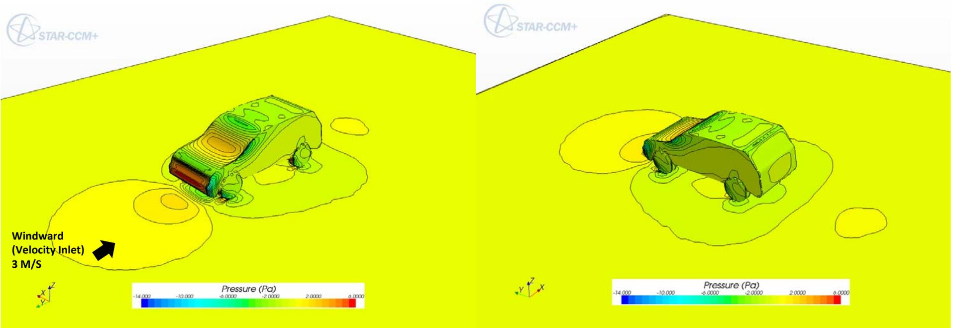
Figure 12: Example of pressure distribution on car surface in post simulation
