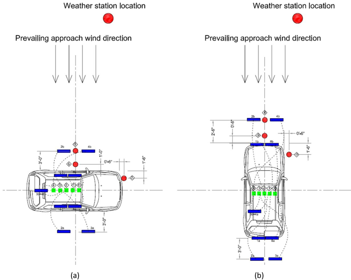
Figure 4.4.3.: . Field Test Series #3: Sensor layout for the third field test: (a) Scenario 1 (wind perpendicular to the car) and (b) Scenario 2 (wind parallel to the car)
