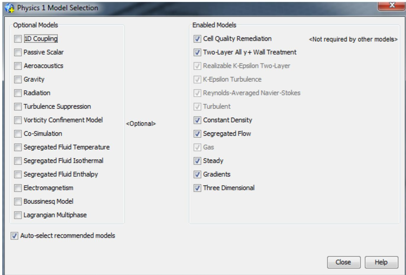
Figure 9: Continua physic model set up
