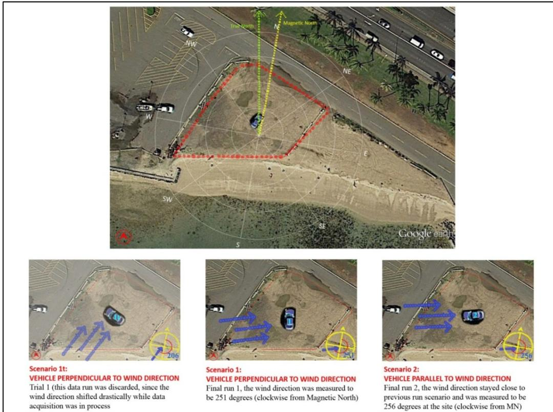
Figure 4.4.1: Field Test Series #3: Sensor layout for the third field test: (a) Scenario 1 (wind perpendicular to the car) and (b) Scenario 2 (wind parallel to the car)
