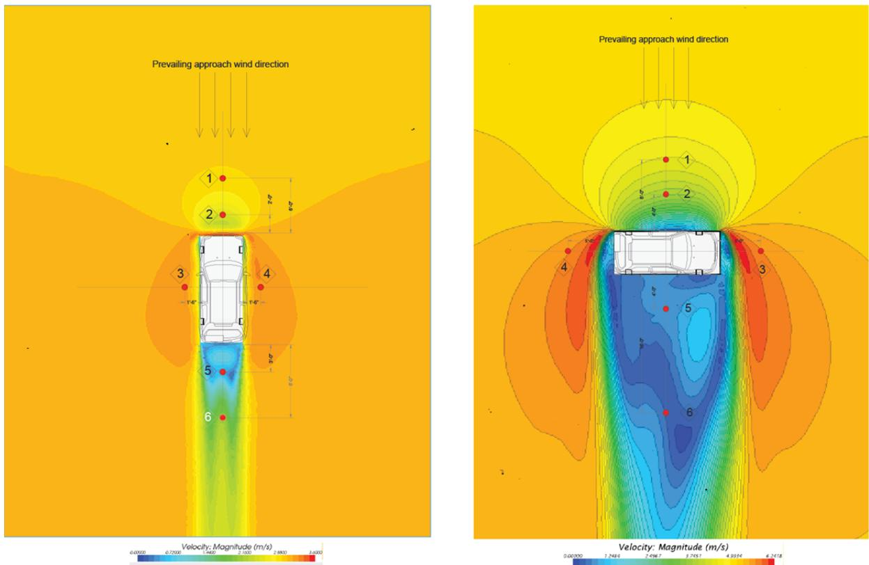
Figure 2.3.1: The example of sensors locations mapping on the initial CFD analysis for measuring test scenarios.
