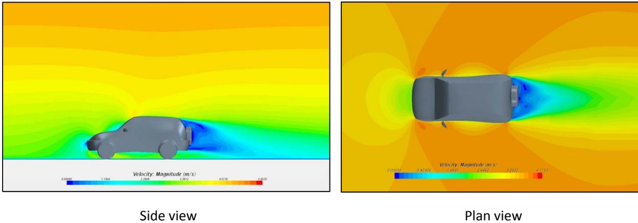
Figure 6.6.1.2: **Scenario 2:** Velocity map at cross section and Pressure map at 3 feet height elevation plane (Scenario 2: approach wind parallel to the longitudinal axis of the car)
