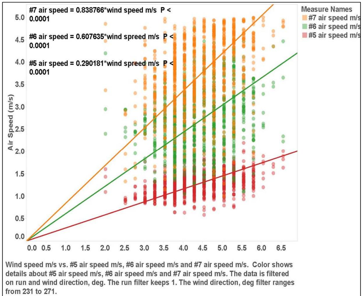
Figure 5.2.4.: Wind speeds (m/s) for sensors #5, 6, and 7 for third field test (Scenario 1)
