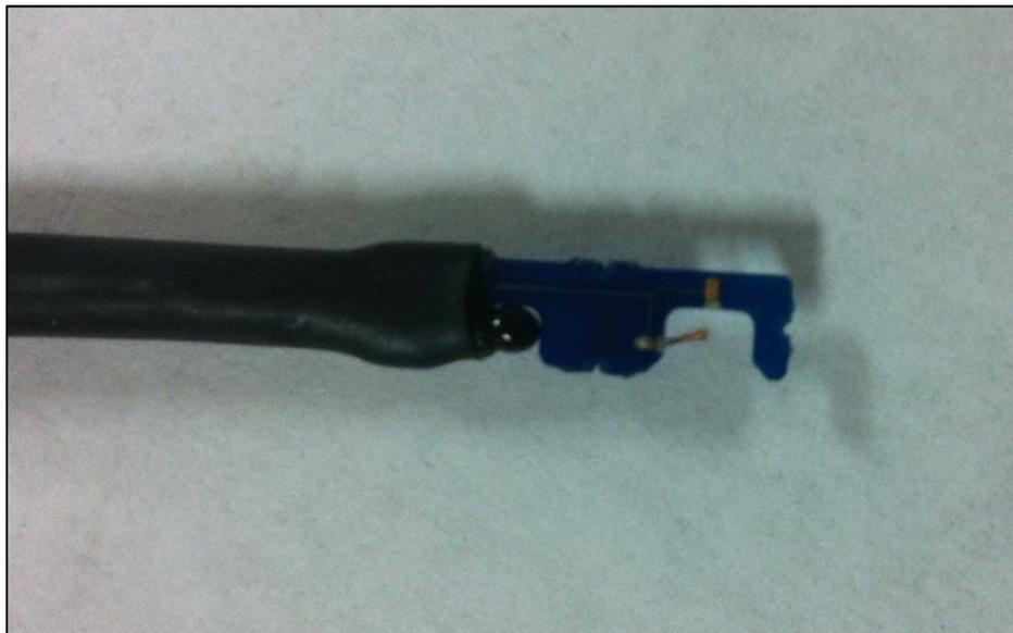
Figure 3.2.8.: The DegreeC F900 Anemometer.
