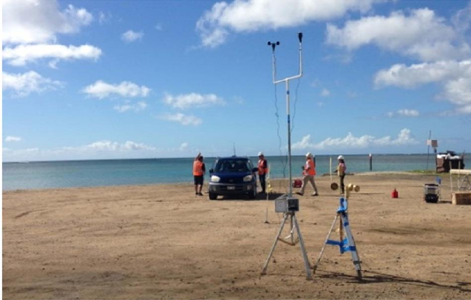
Figure 3.2.6.: Setup of the Onset U30 Weather Station at Maunalua Bay Beach Park
