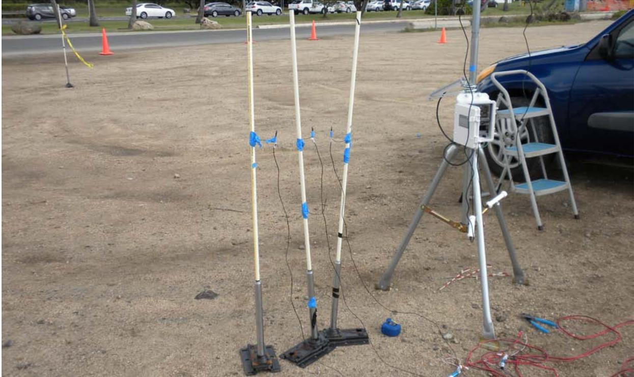
Figure 17. Calibrating airflow sensors (F900 anemometers) to compare wind speed profiles
