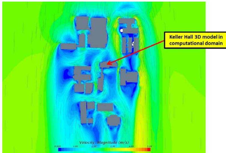
Figure 4.3.7: Type Figure 5 = Plan View of Overall Wind Velocity Streamline Map
