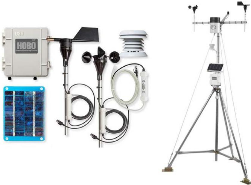
Figure 3.2.1: Onset HOBO U30 weather station (source Onset)
