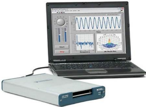
Figure 4.9: Data acquisition for differential pressure transducers
