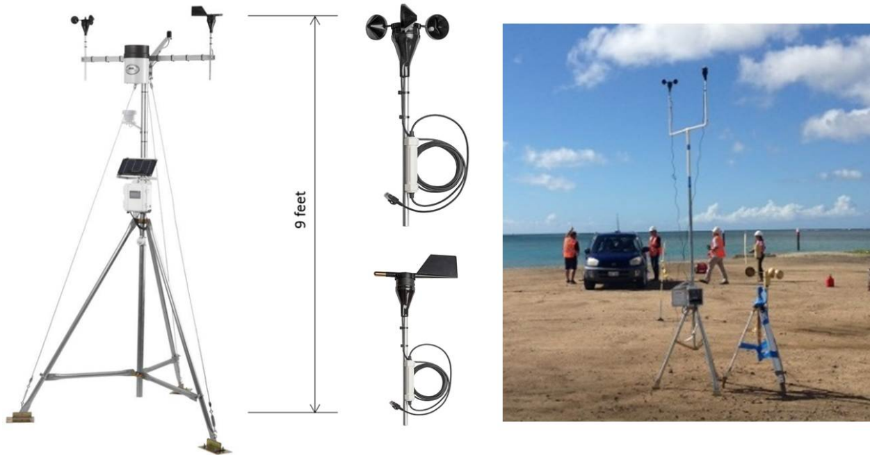
Figure 4.8: Mobile weather station; used during the shake down testing at the beach side test site. (Figure presented in Project Report 3, Develop and Test Field Measurement Procedures)
