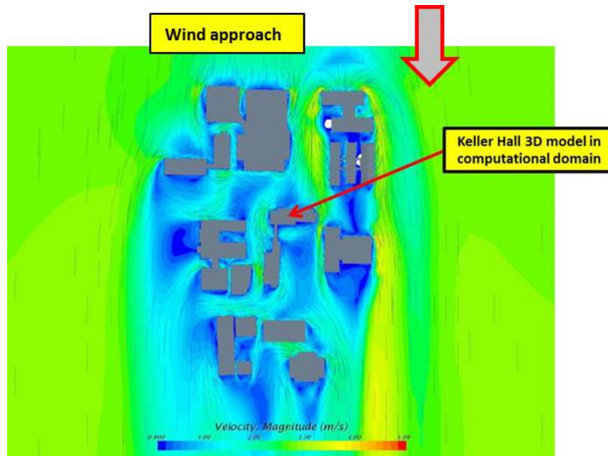
Figure 5.12: Plan View of Overall Wind Velocity Streamline Map (Figure presented in Project Report 4, External CFD Simulation and Field Validation)
