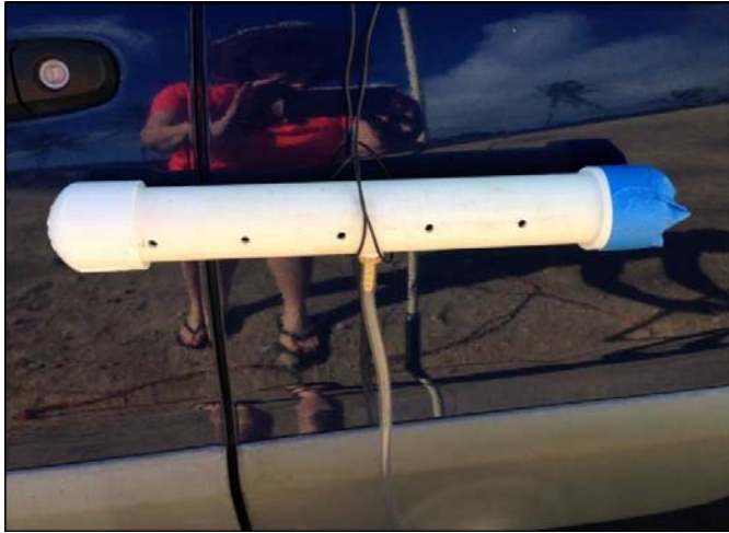
Figure 4.7: Pressure tubing terminal;
