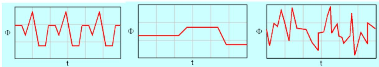
Figure 3.8.2: Time dependency of unsteady flow: (a) Periodic Flow, (b) Non-Periodic Flow and (c) Random Flow
