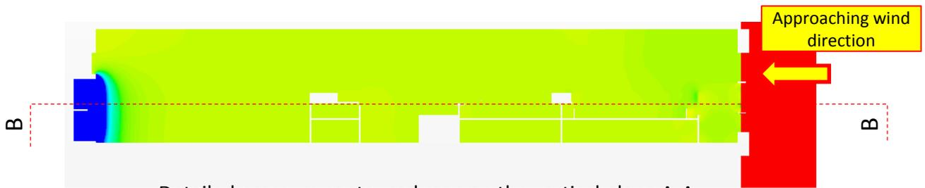
Detailed pressure contoured map on the vertical plane A-A
