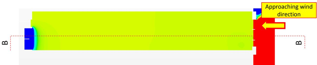
Detailed pressure contoured map on the vertical plane A-A
