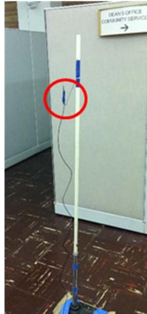
Figure 4.11: Anemometer tip held at 4’ height using wire attached to stand
