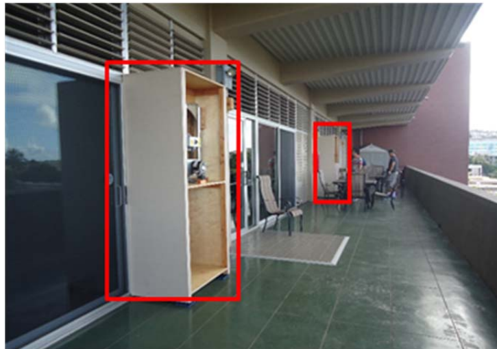
Figure 4. 9: Placement of the two exhaust fan unit on the south lanai (Note that the fan housings remained open to the South)
