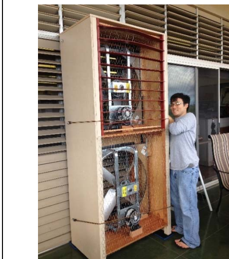
Figure 4. 8: A pair of exhaust fans installed in a custom-built housing
