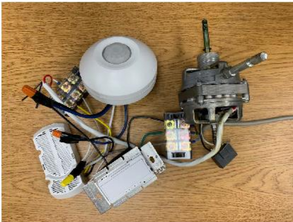
Figure 2 – Wall switch, occupancy sensor, canopy module, and fan motor connected together for mock-up.
