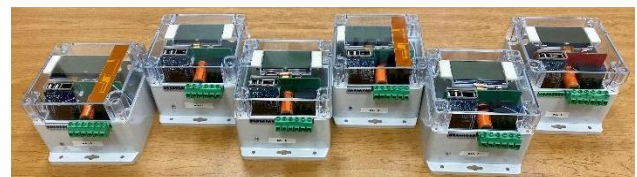
Figure 2. ARGEMS patented custom power meter and controller devices.
