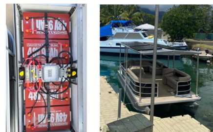
Figure 2. The E-boat's powertrain fixed battery system (left) and shade structure PV system (right).
