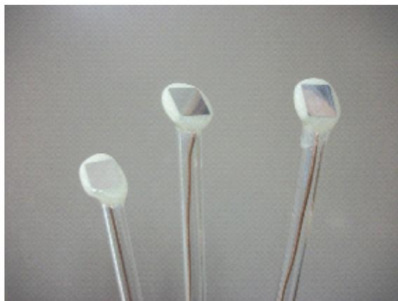
Figure 8: Three electrodes; the metallic area is  $1\text{cm}^2$
