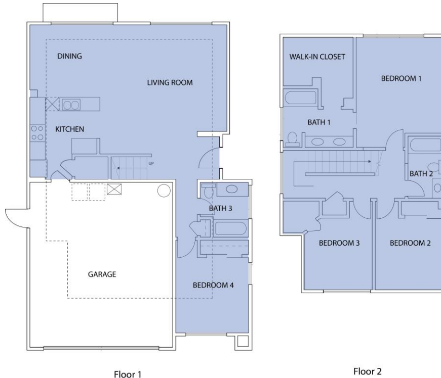
Figure 3.3.1.1. Floor Plan of House 3 with the blue representing the conditioned spaces.
