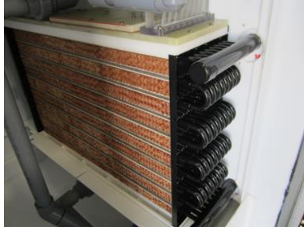
Figure 2–50 Wicking fin regenerator (Credit: AIL Research, with permission)
