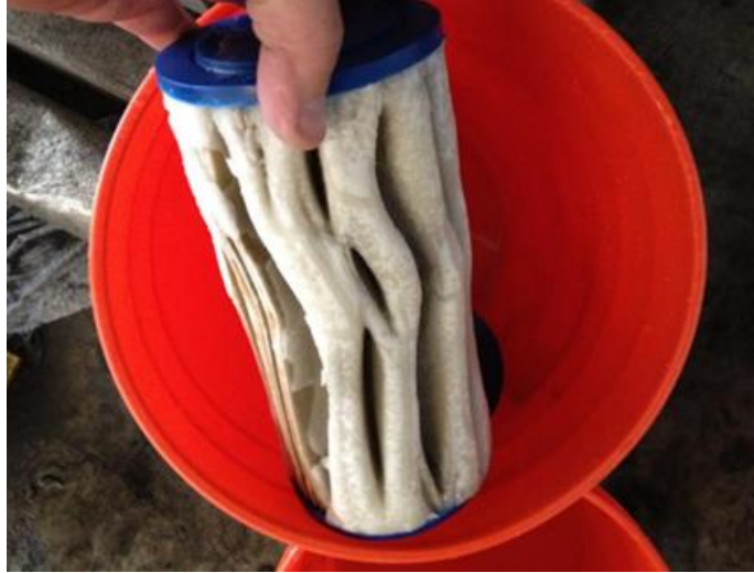
Figure 2–19 Regenerator filter clogged with precipitate, Encinitas, California (Credit: AIL Research, with permission)
