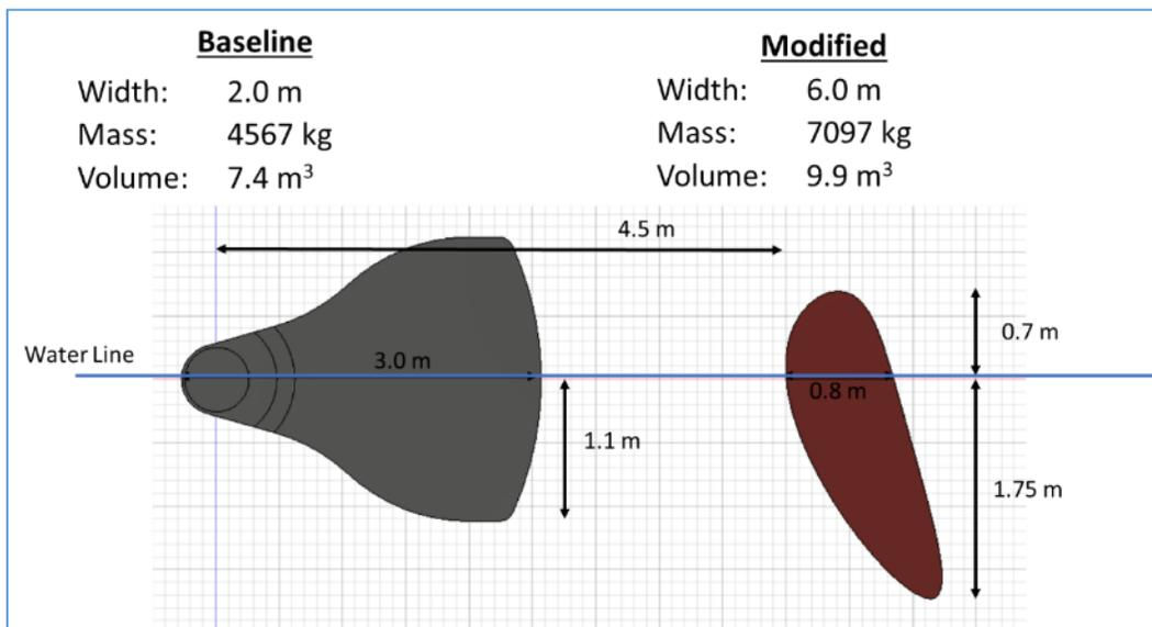
Figure 5 – Cross Section of Baseline and Modified Floats
