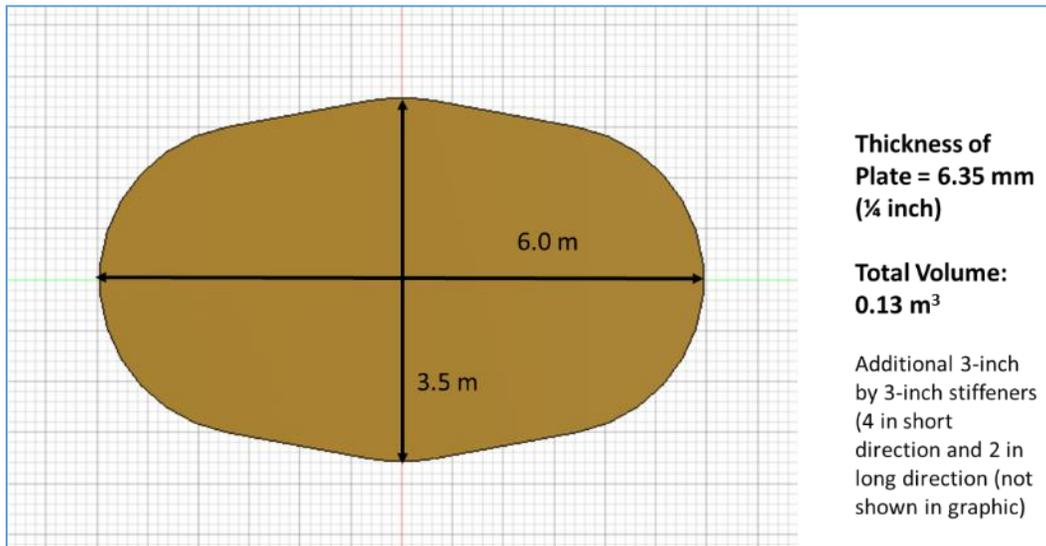
Figure 2 – Heave Plate Shape and Dimensions
