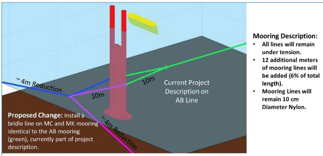
Figure 12 – Detail View of Modified Bridle
