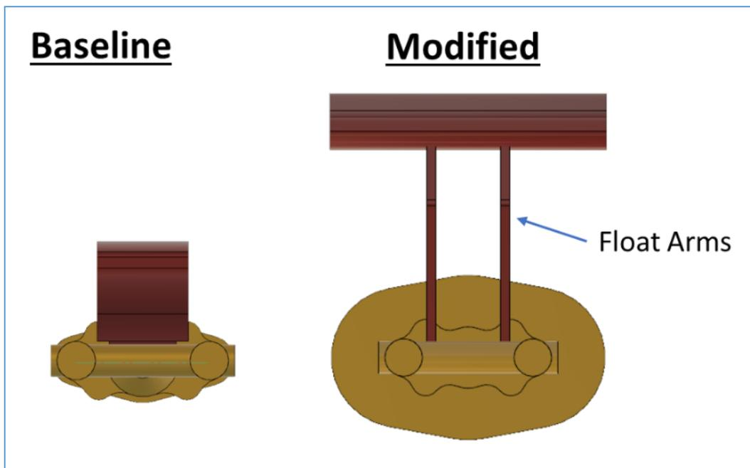
Figure 7 – Top View of Modified Float Showing Float Arms
