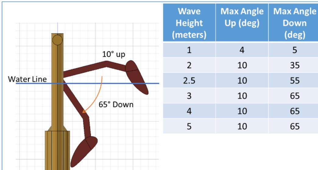
Figure 14 – Float Angle as a Function of Sea State
