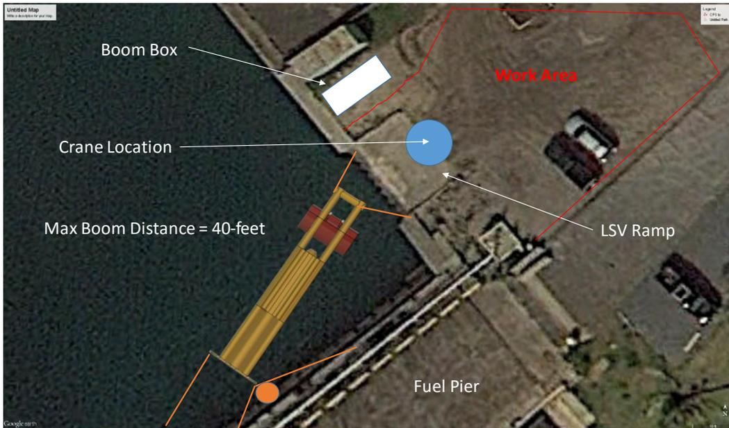
Figure 18 – Location of device during modifications
