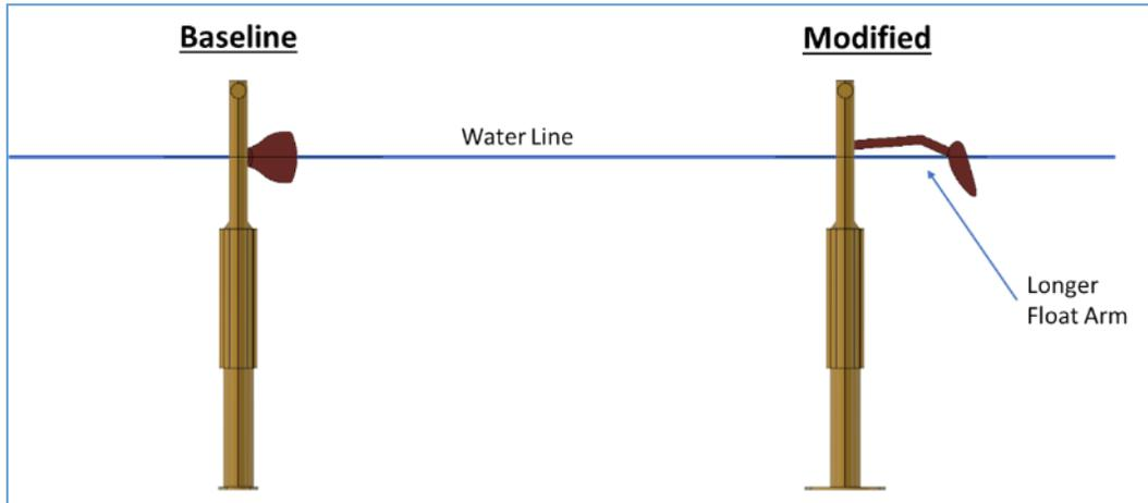
Figure 6 – Side View of Baseline and Modified Floats
