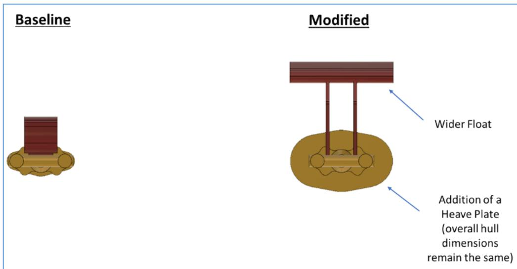
Figure 3 – Top View Showing Addition of Heave Plate
