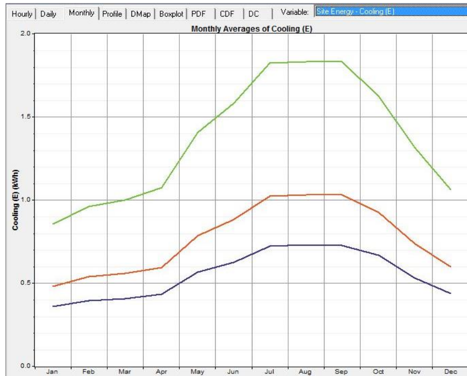
Figure 23. Energy simulation graphical output from BEOpt showing energy use over the year of a house before retrofit (green line), a retrofitted house (red line), a hypothetical retrofitted house with a deeper retrofit.
