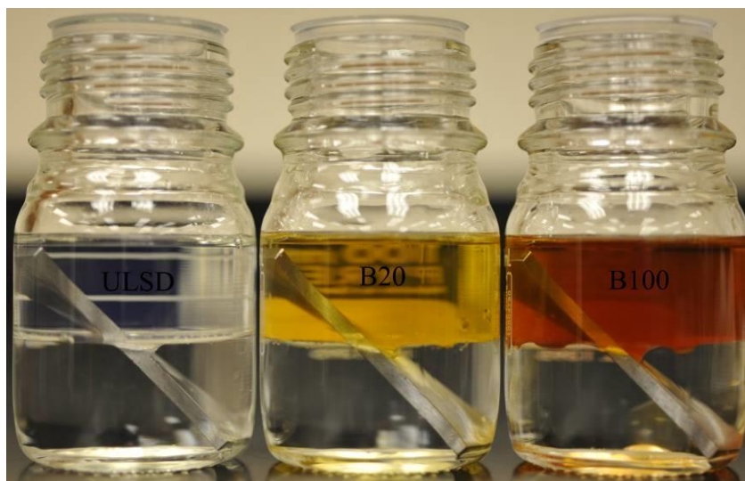
Figure 2.7.1 Experimental setup of fuel-water mixture with 1018 steel coupons immersed
