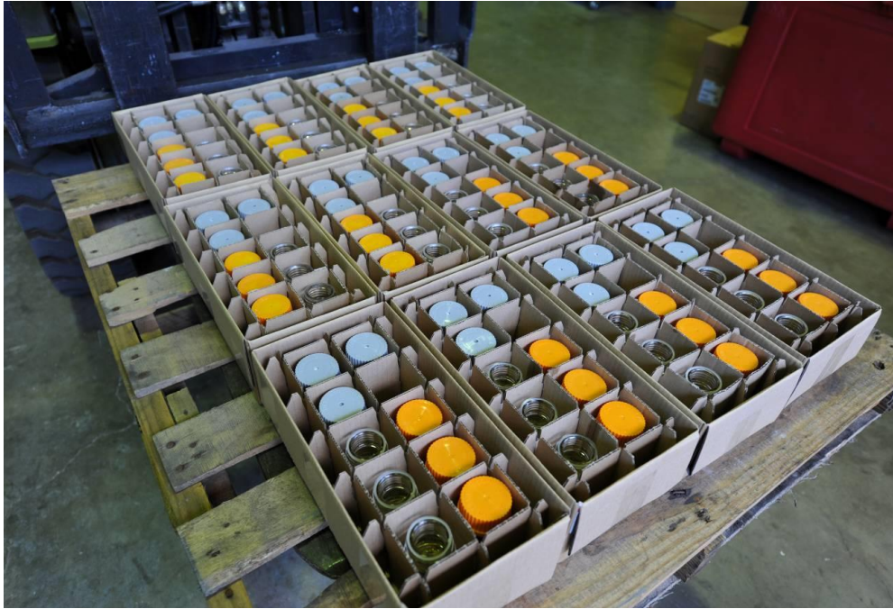
Figure 2.7.20 Samples loaded on pallet to be exposed outdoors
