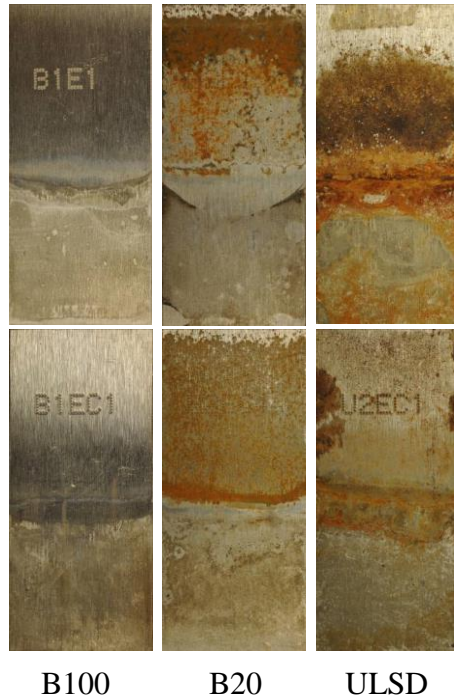
Figure 2.7.2 Photos of 1018 steel coupons after six-week exposure duration. Top row, left to right: B1E1, B2E1, U2E1; bottom row, left to right: B1EC1, B2EC21 and U2EC1 (control specimens).
