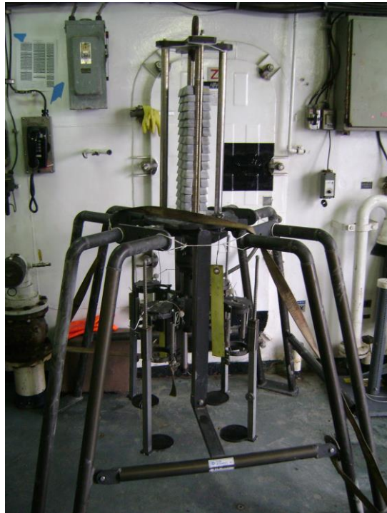
Figure 3.6 Multi-core system used to collect seafloor sediment samples during the 2009 Beaufort Sea expedition
