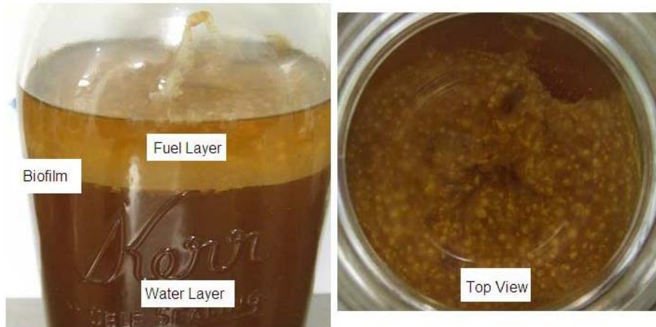
Figure 2.6.2 Contaminated biodiesel sample from the City & County of Honolulu. The sample shows the different separations including the interface film.
