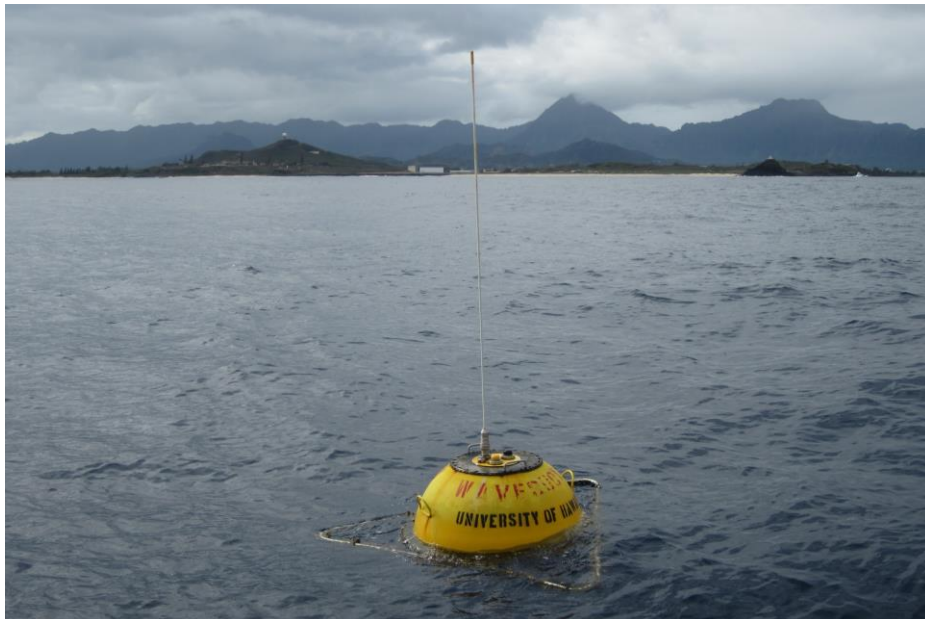
Figure 3.5. Waverider© buoy deployed at WETS, near the 60m test berth.
