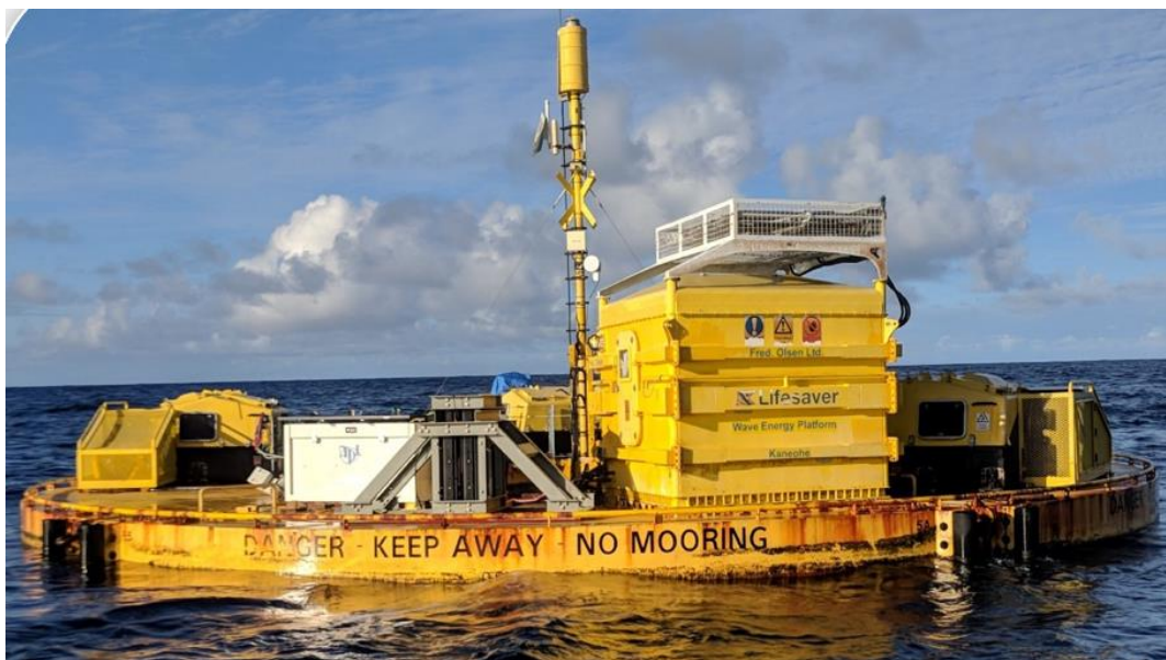
Figure 1.12. Fred. Olsen Bolt Lifesaver during second deployment at WETS. Note the UW AMP electronics enclosure (white box) and the above-water portion of the AMP instrumentation package. (The sensor head is approximately two meters below the water surface, but could be raised when the device is in transit to/from the site.)
