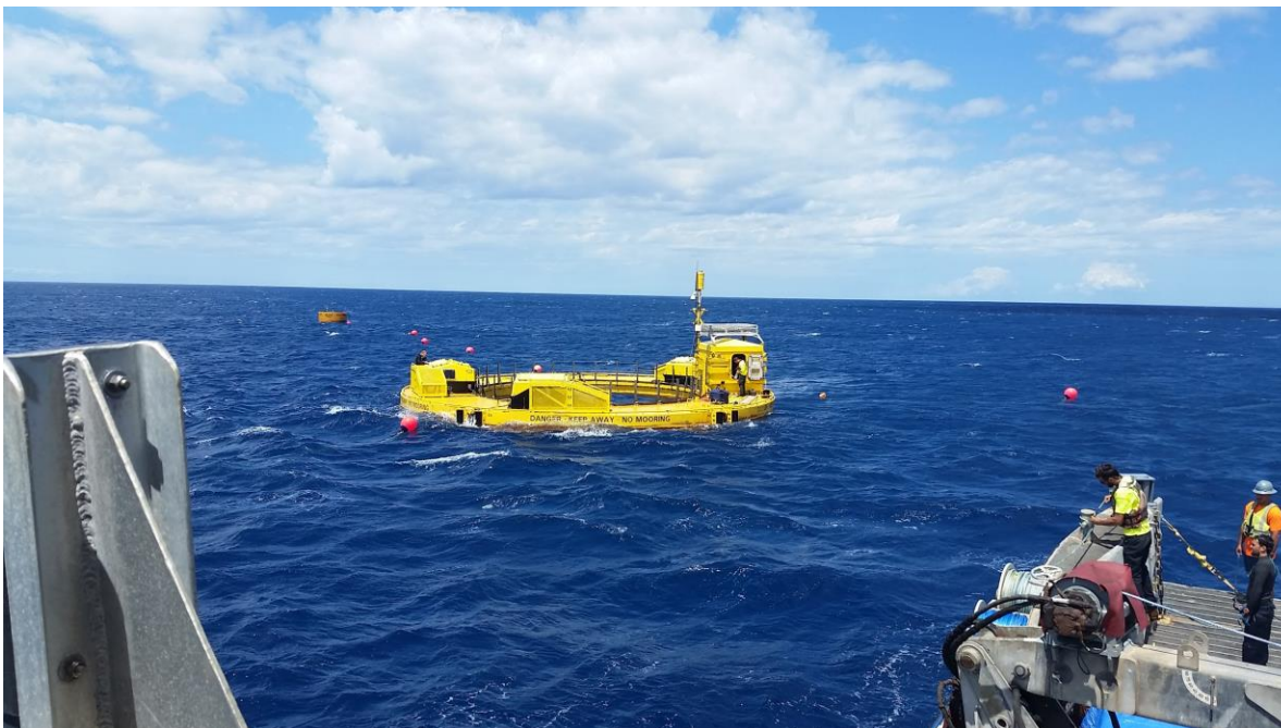
Figure 1.11. Fred. Olsen, Ltd. Lifesaver during deployment by Sea Engineering, Inc. in March 2016 at the WETS 60m test berth.
