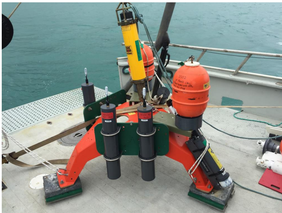
Figure 4.5. Loggerhead Instruments acoustic packages deployed aboard a Teledyne Seaspider package for deployment at WETS. System is configured with dual acoustic release system for post-deployment recovery.
