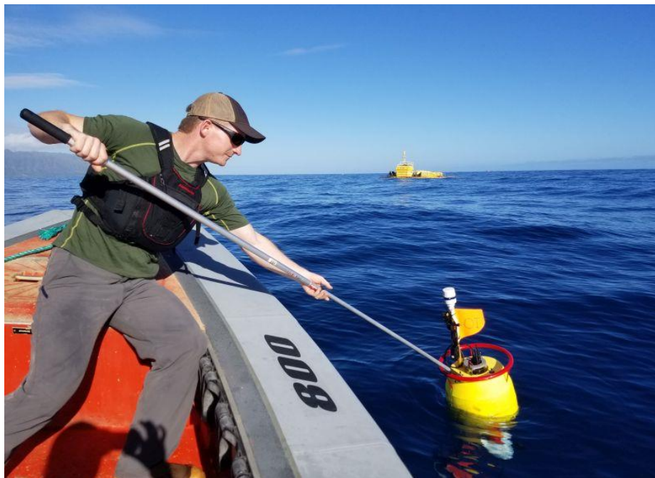
Figure 4.2. University of Washington SWIFT buoy being deployed at WETS in the vicinity of the Fred. Olsen Lifesaver WEC.
