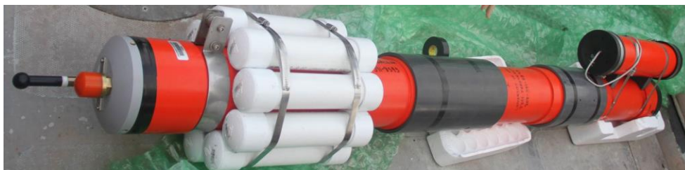
Figure 4.1. The Acoustic Monitoring Package, single channel (AMP-1) was developed at the University of Hawaii (UH).
