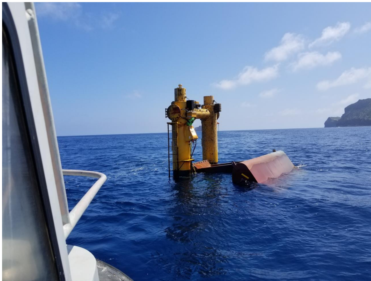
Figure 1.10. Advanced Azura Prototype during an inspection by Sea Engineering at WETS in spring 2018. Note larger float with greater moment arm, as compared with baseline Azura.
