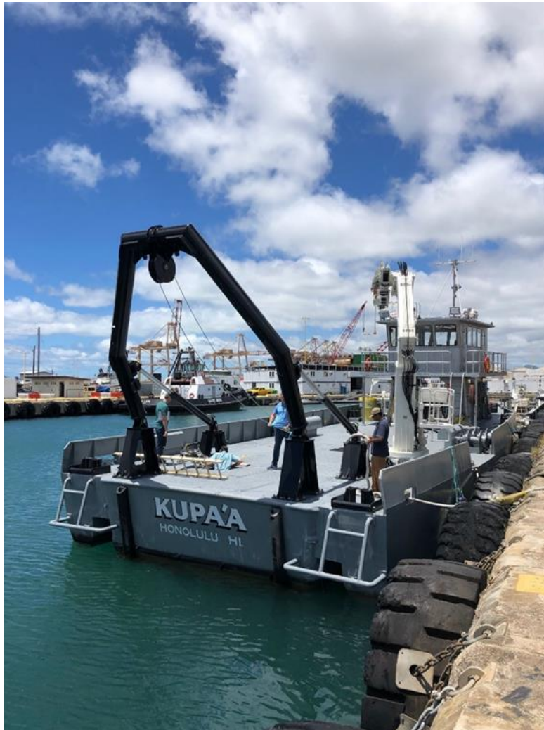
Figure 1.7. Kupa'a, nearing completion for service at WETS in September 2019. A-frame and knuckleboom crane are visible, as are modified (wider) hull sponsons and expanded wheelhouse.
