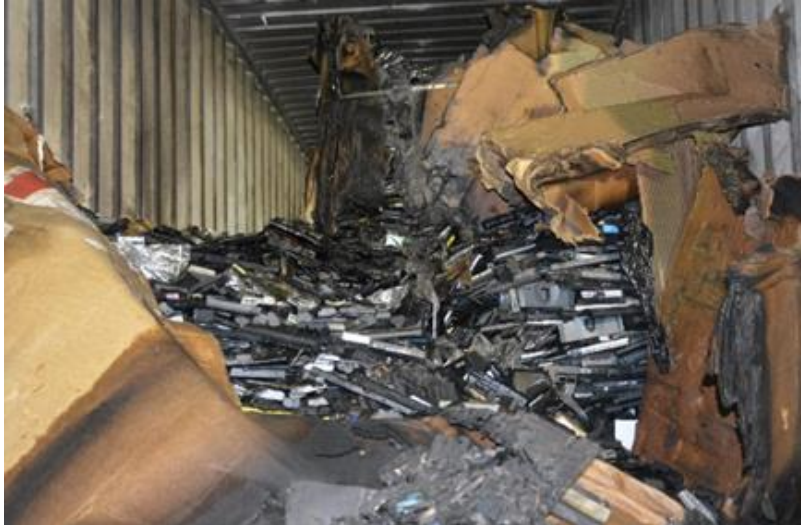
Figure 6. Burned Li-ion batteries found in fiberboard boxes after the August 19, 2021 fire. Photo courtesy U.S. Coast Guard.
