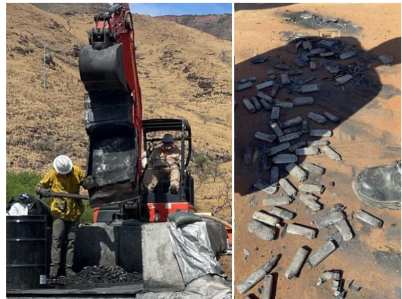
Figure 5. Burnt Li-ion batteries recovered from Maui fire. Photo courtesy of onsite team.
