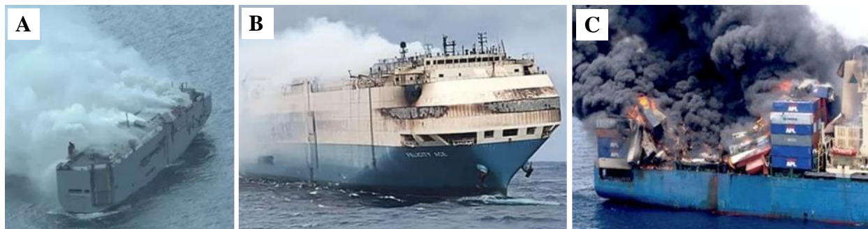
Figure 4. Recent cargo ship fires due to EVs containing EOL still activated Li-ion batteries. (A) the Fremantle Highway (2023); (B) the Felicity Ace (2022); and (C) the Hoegh Xiamen (2020). All fires resulted in a total loss of all cargo.
