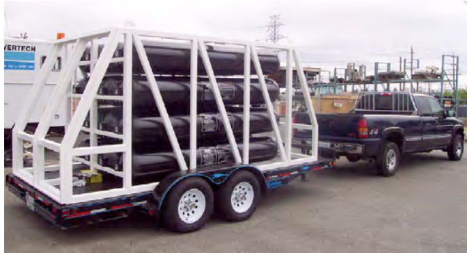
Figure 5.3: Lightweight hydrogen tube trailer
