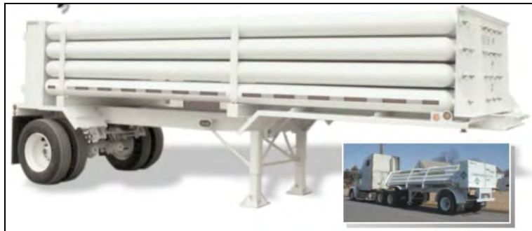
Figure 5.4: Full size hydrogen tube trailer
