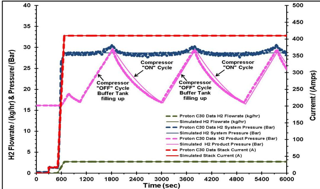
Figure 18: Simulated compressor cycle results compared with data from the Proton C30 electrolyzer
