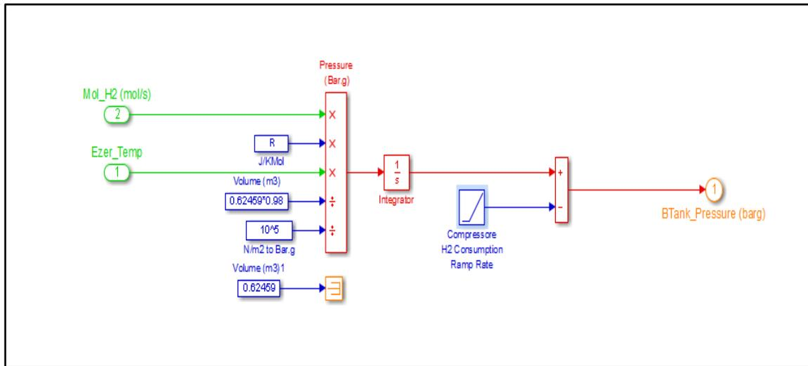
Figure 14: Buffer tank pressure control model block
