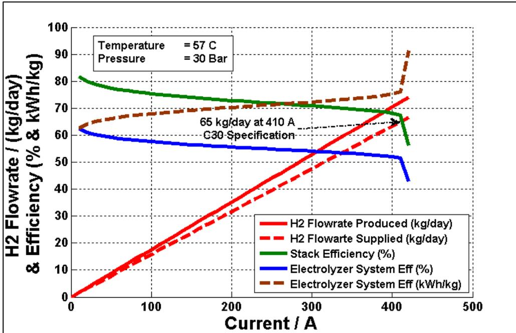
Figure 7: H<sub>2</sub> Flow Rate & Efficiencies of C30 System
