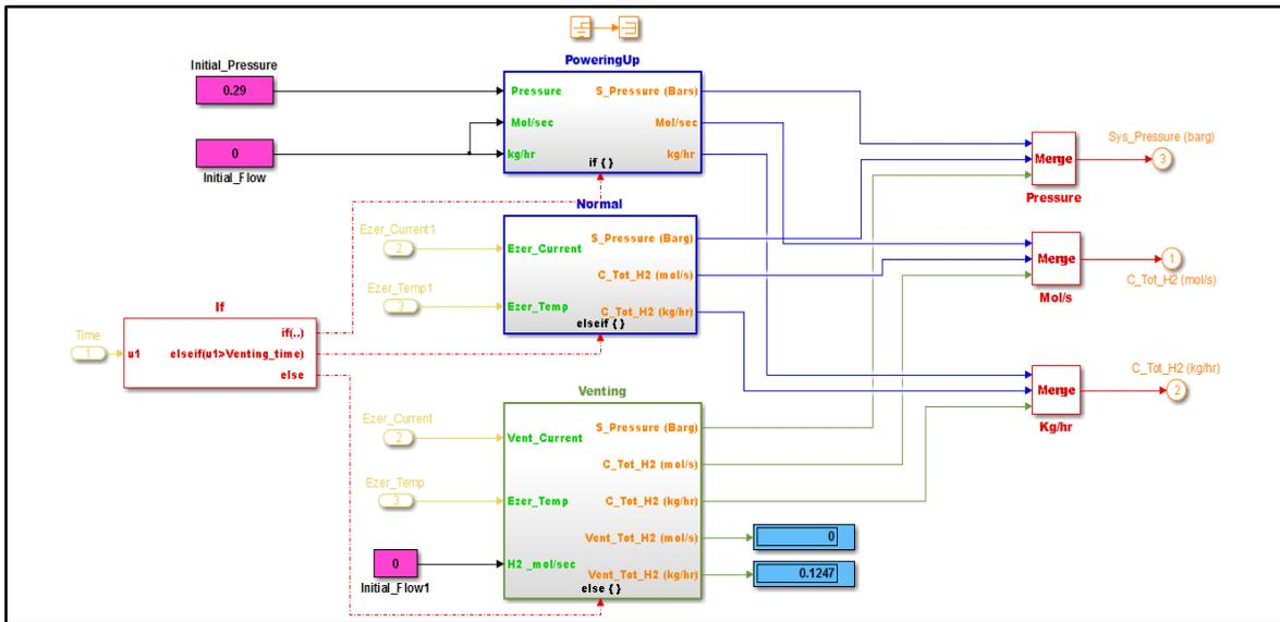
Figure 12: Overall system pressure control model
