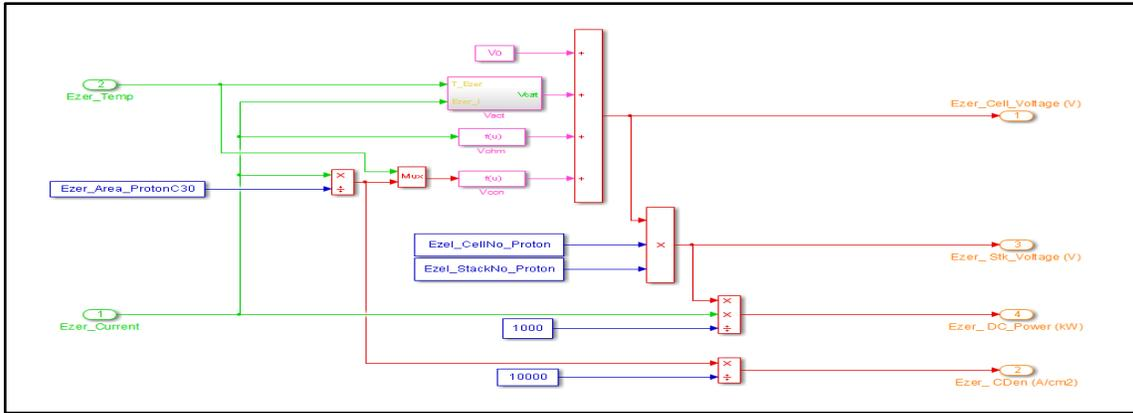
Figure 10: Electrolyzer cell and stack model block
