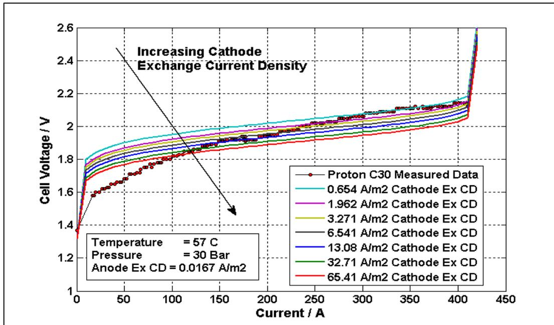
Figure 4: Cathode Exchange Current Density
