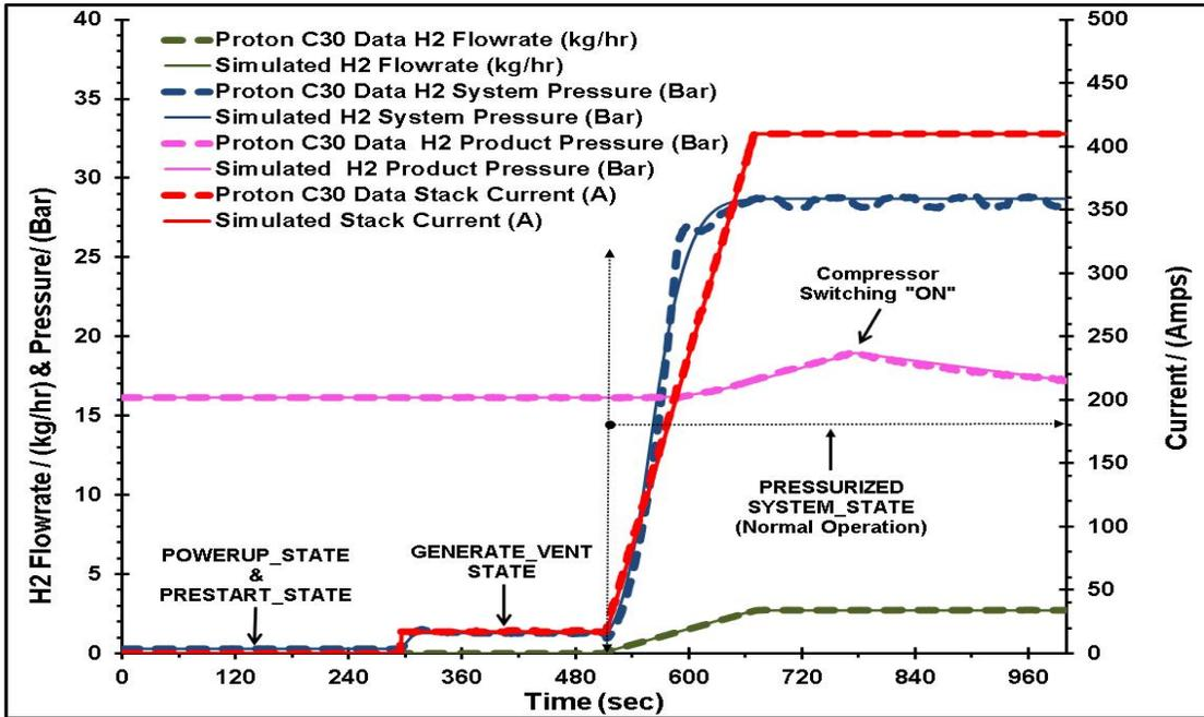
Figure 15: Simulated results compared with data from the Proton C30 Electrolyzer
