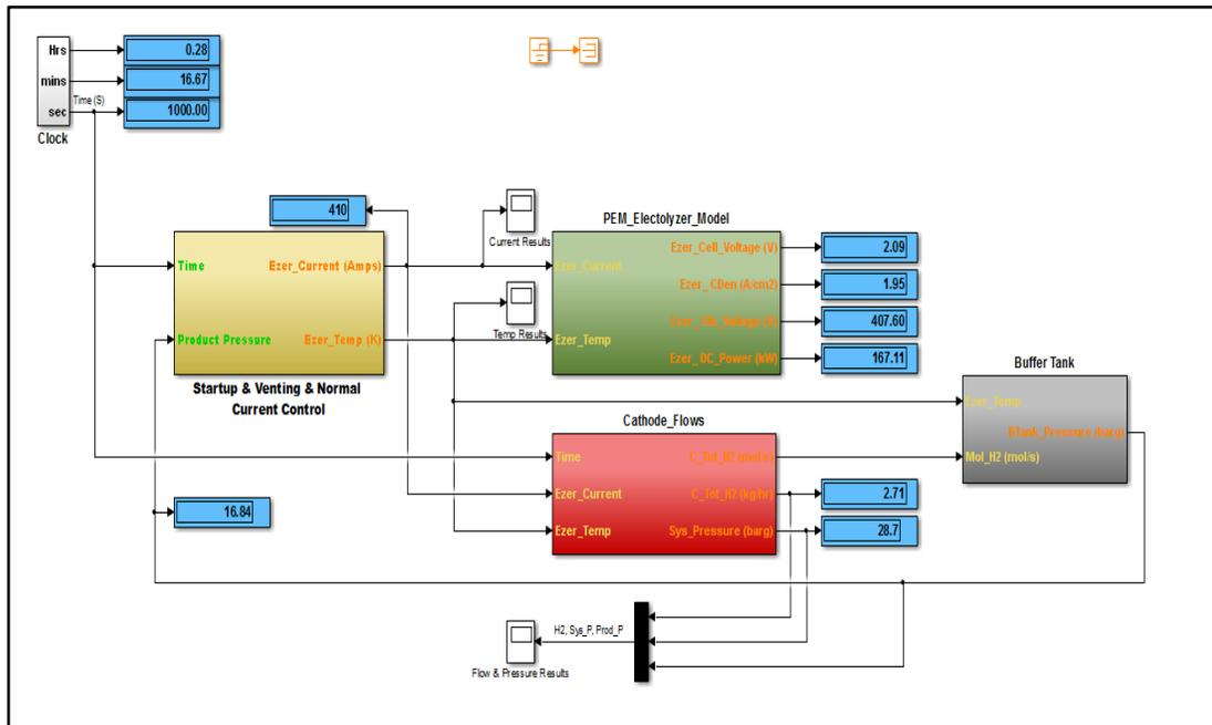
Figure 9: Electrolyzer System Model in the Matlab/Simulink Environment
