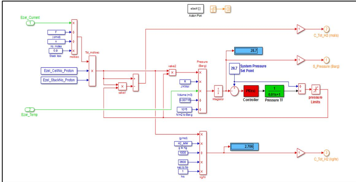
Figure 13: System pressure control model block during the normal operation
