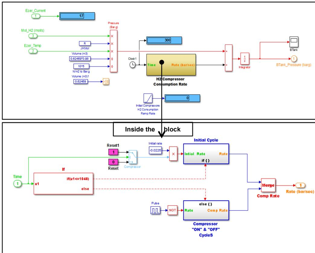
Figure 17: Compressor cycle model inside the buffer tank block
