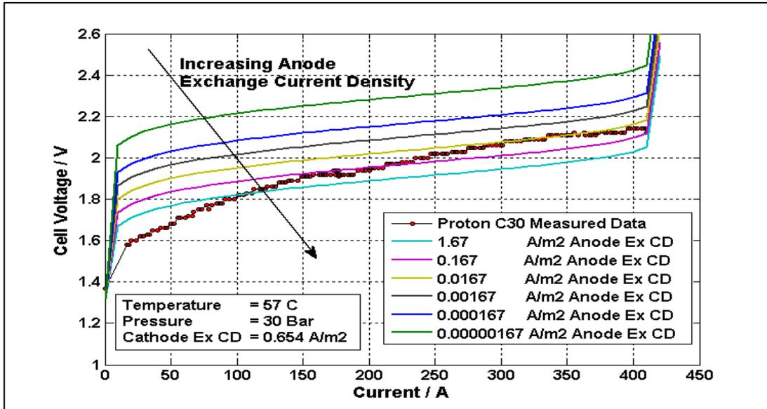
Figure 3: Anode Exchange Current Density
