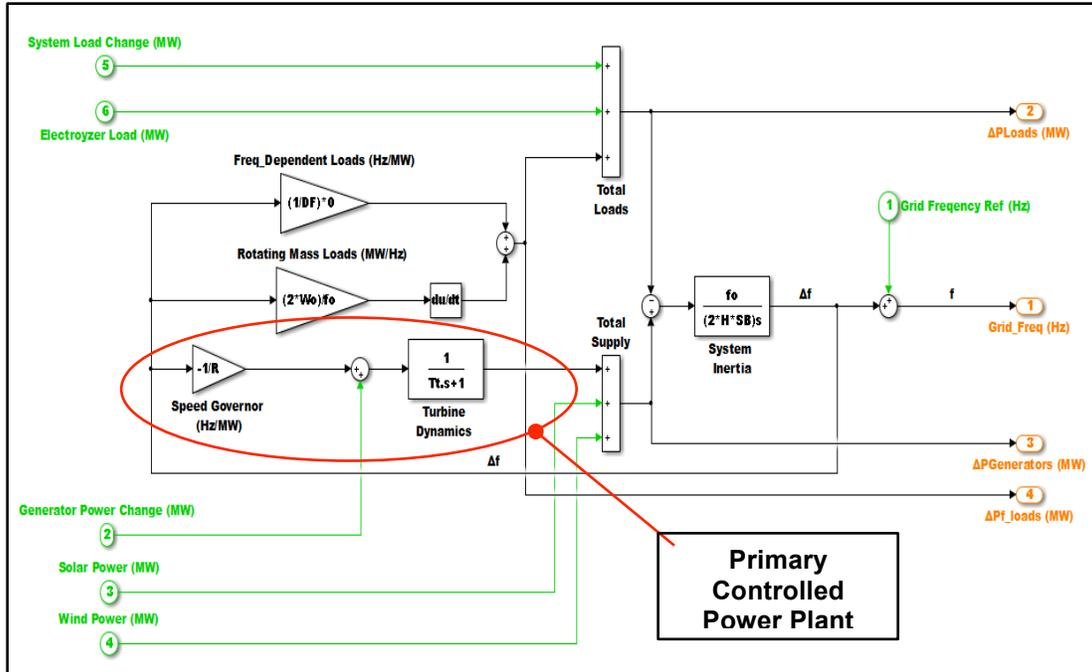
Figure 19: Grid Power System Simulink block with dynamic frequency model with the primary controlled power plant.
