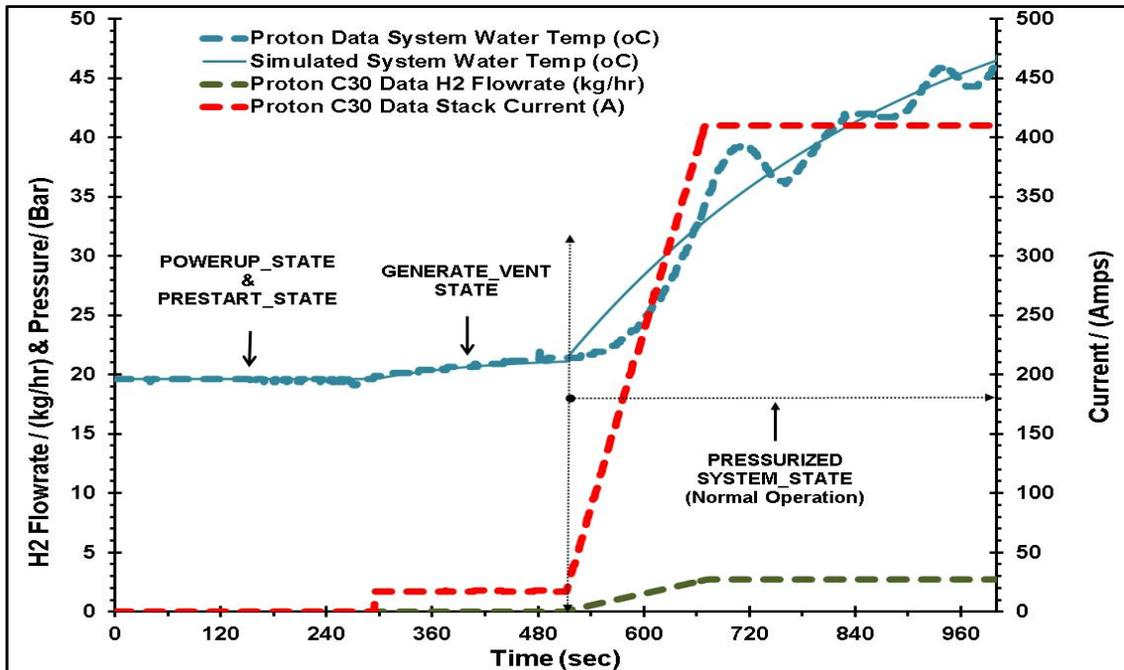
Figure 16: Simulated temperature result compared with data from the Proton C30 Electrolyzer
