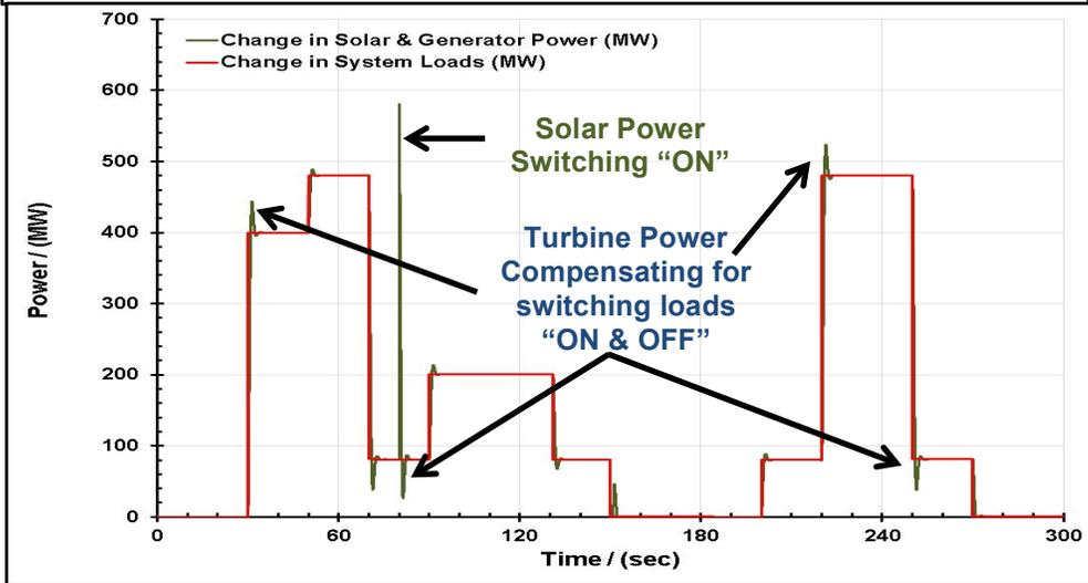
Figure 20: Simulated results from the grid power system model for different step change input power signals
