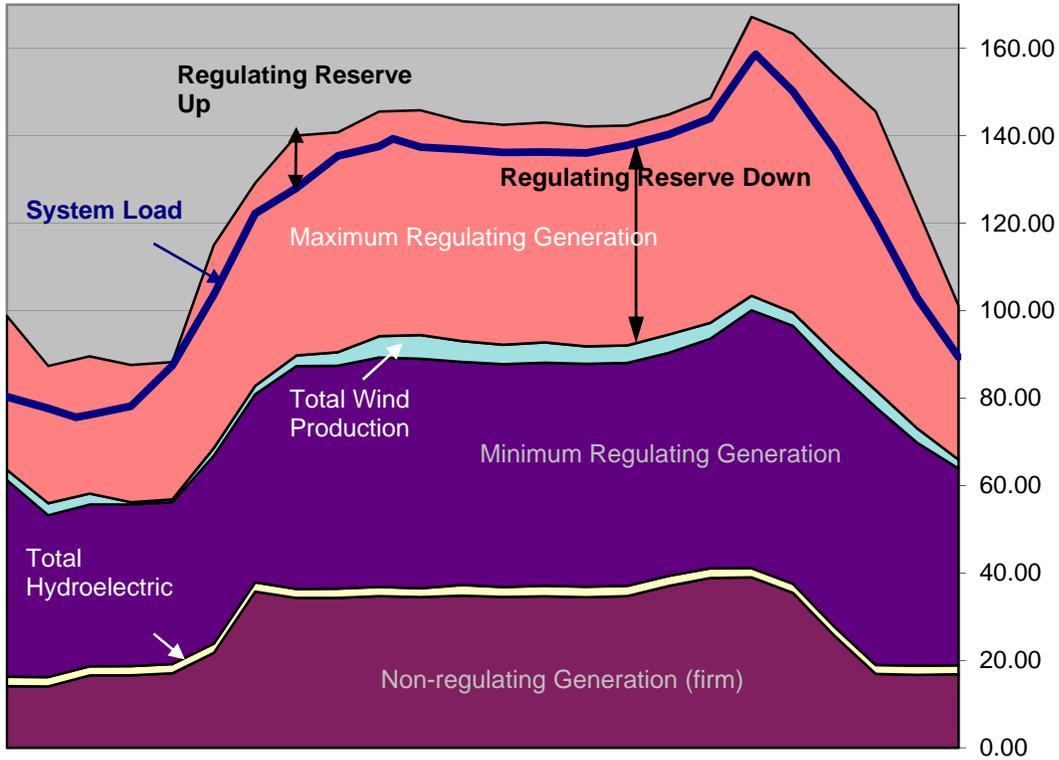
Figure 4 illustrates a scenario that HELCO will be encountering in the future. This figure assumes that three steam units – Hill 5, Hill 6, and Puna – can regulate the system frequency. (It is possible that with more renewable generation the utility may need to have more regulating generation reserves.)
