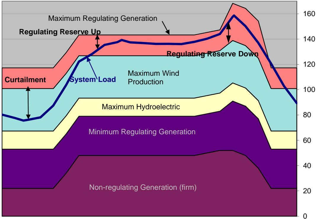
The figure includes PGV and HCPC at contract levels for the fixed generation. Hydro is at 14.4 MW and consists of Wailuku River Hydro at 11 MW and HELCO’s hydro at 3.5 MW. The expected maximum wind production, based upon planned expansion of Kamaoa, Lalamilo and Hawi, is expected to be approximately 40 MW in the near future. This example is based on wind loading at 83% and has Kamaoa at 16 MW, Lalamilo at 8.5 MW, and Hawi at 9 MW.
