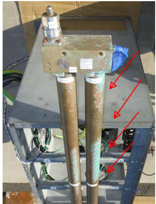
Fig 4: Corrosion by salt air flow
