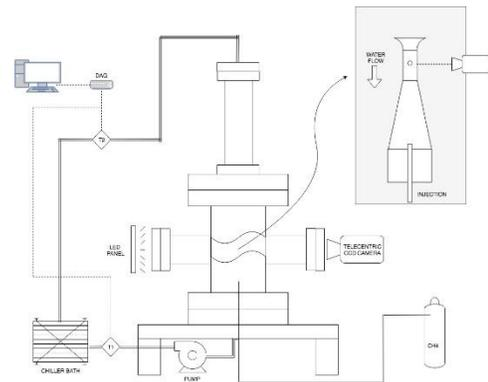
Figure 1. Schematic diagram of the water tunnel.
