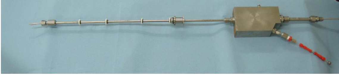
Figure 3.1.4 Photograph of the fiberoptic probe assembly
