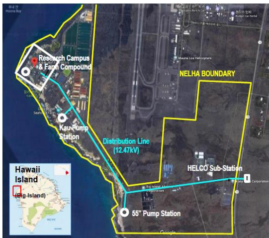
Figure 1. NELHA's HOST Park site and existing HELCO primary distribution feeder.
